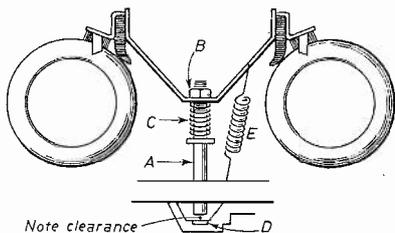
Fig. 3: Sketch of the brake mechanism used in Philips tape decks.
