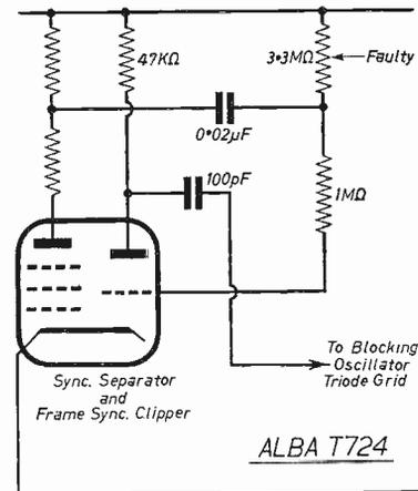
The  $47\text{k}\Omega$  anode resistor was correct, as was the  $0.02\mu\text{F}$  coupler from the anode of the sync separator (pentode section). All that was left was the fixed potentiometer in the grid circuit, which consists of a  $3.3\text{M}\Omega$  and a  $1\text{M}\Omega$  in series from the h.t. line, with the  $0.02\mu\text{F}$  coupler taken to their junction.
