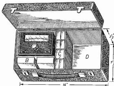
It is in four sections, as shown in the drawing. The leather partitions are about an inch shallower than the base, allowing one to overlay the compartments with a soldering iron, valve manual and duster. The iron shank and bit are housed in a tubular spanner  $\frac{1}{4}$  in.  $\times$   $\frac{1}{8}$ , standard size for potentiometer locknuts.
