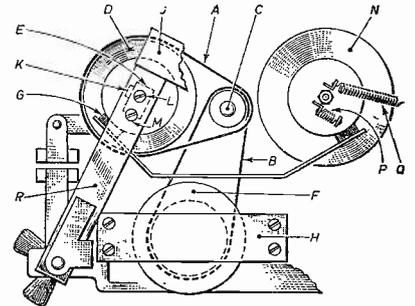
Fig. 4: Main mechanical assembly, underside, of a typical Walter tape deck.
