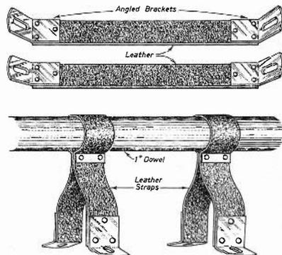
reasonable allowance for movement of the straps along the rod to facilitate the gadget's use on various types of machines.
