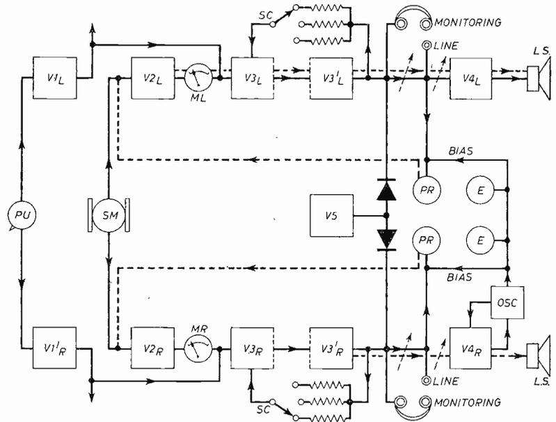
Fig. 3: Block diagram of the Philips EL3536, showing switching.
