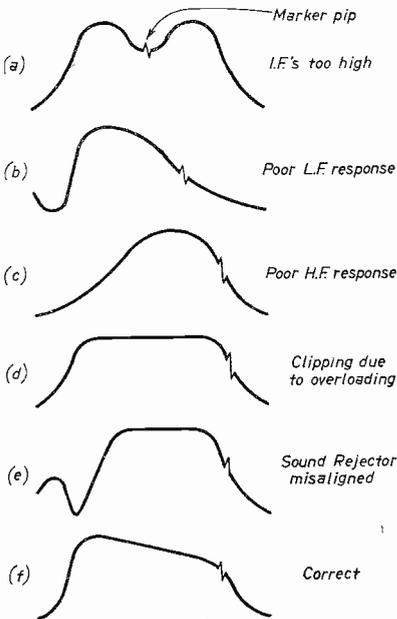
Fig. 4: Typical alignment traces obtained on oscilloscope as described in the text.
