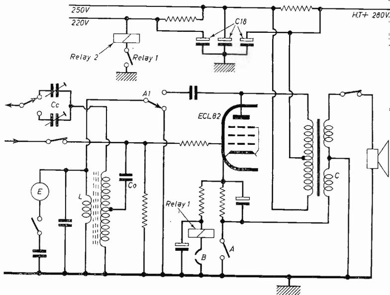
Fig. 2: Output stage of the Philips EL3542, showing positions of relays.
