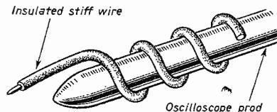
Fig. 1: Method of loose coupling to oscilloscope for testing e.h.t.
