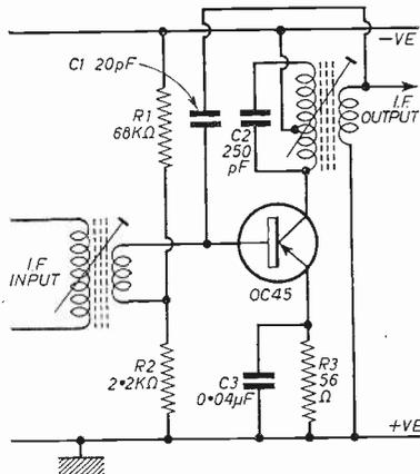
Fig. 1: Typical transistor i.f. stage.
