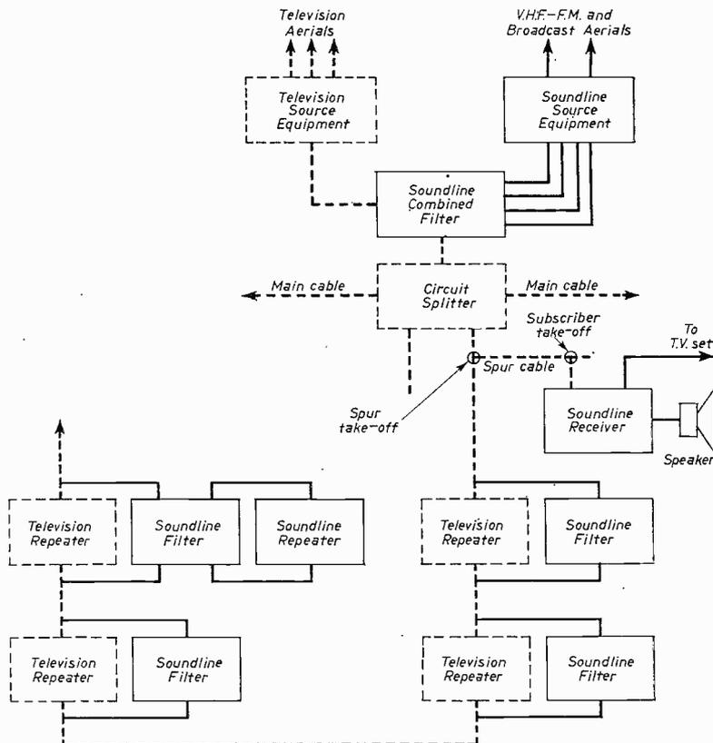
Fig. 1: Showing how Soundline may be added to an existing co-axial system. The broken line items are those which may already be in use on television, while the full line items are the sound additions. Owing to the smaller cable loss at the lower frequencies, a Soundline repeater is required after three or four television repeaters.
