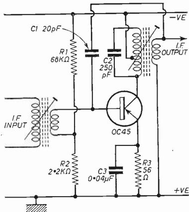
Fig. 1: Typical transistor i.f. stage.
