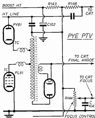
From the circuit diagram it will be seen that the short from the junction of R143/R148 was in effect cleared when the focus control centre tap was turned to the earthy end of the track. Replacing the 0.1 $\mu$ F capacitor restored the circuit to its proper working conditions.—D.Mc.L., Lochgilphead (1050)
