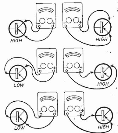
Fig. 2: Typical measurement of transistor with 20,000Ω/V meter. Note that the positive terminal refers to polarity at meter (ohm-meter battery may apply positive voltage to negative terminal of meter). Do not take these readings with transistor in circuit. Use Ohms X100 range of meter.
