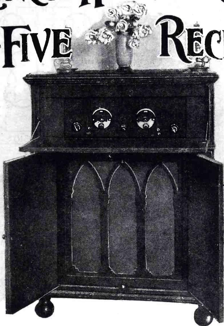
THE battery operated Lynch-Hammarlund Five receiver was described in the preceding number of this publication. The remarkable popularity of this receiver following its introduction to the radio enthusiast has more than justified a revision of the circuit to adapt it to the use of alternating current tubes.
