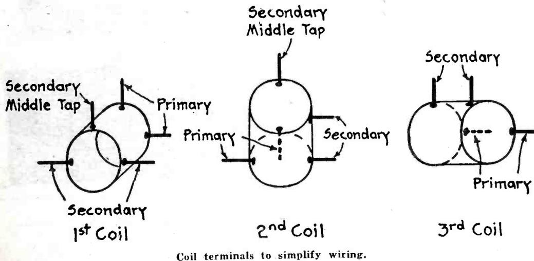
Coil terminals to simplify wiring.
