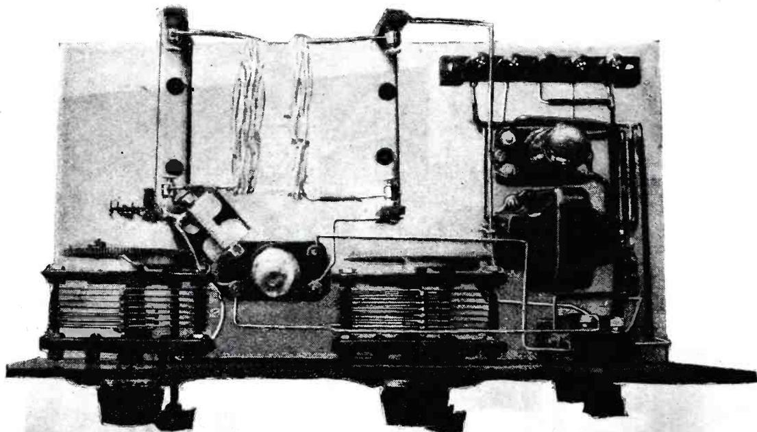
that both capacity and resistance losses are reduced to a negligible amount. The position of the coils is such, relative to the other apparatus, that neither dielectric materials nor metal parts are situated closely in the fields of the coils, yet, all connecting leads in the radio frequency portions of the circuit are short and direct.
