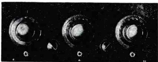
Panel view of the three-range receiver. The three larger dials are the tuning controls. The first knob at the left is the rheostat and the one at the right is the potentiometer.
