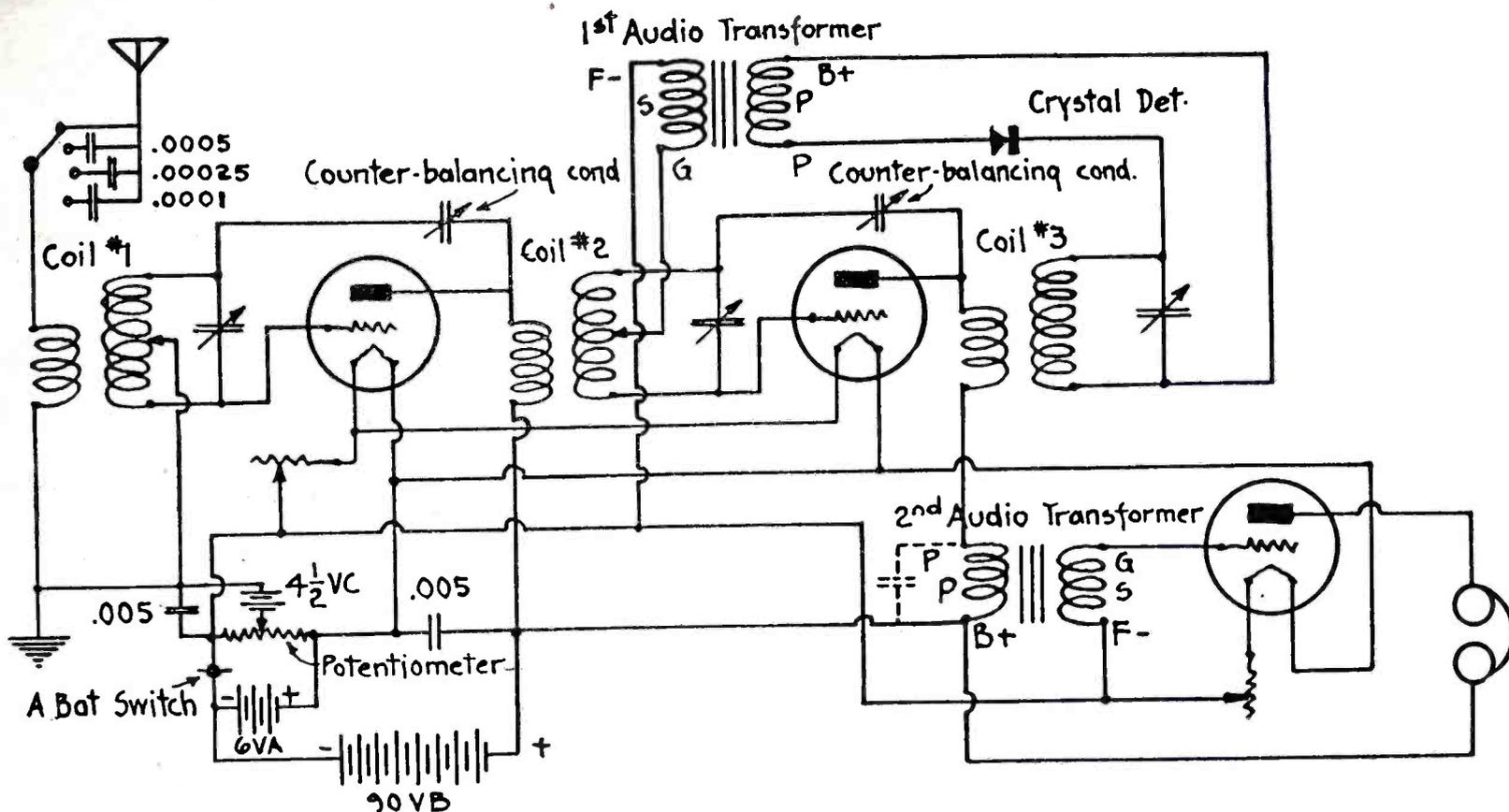
Circuit diagram for three-tube reflex receiver.
