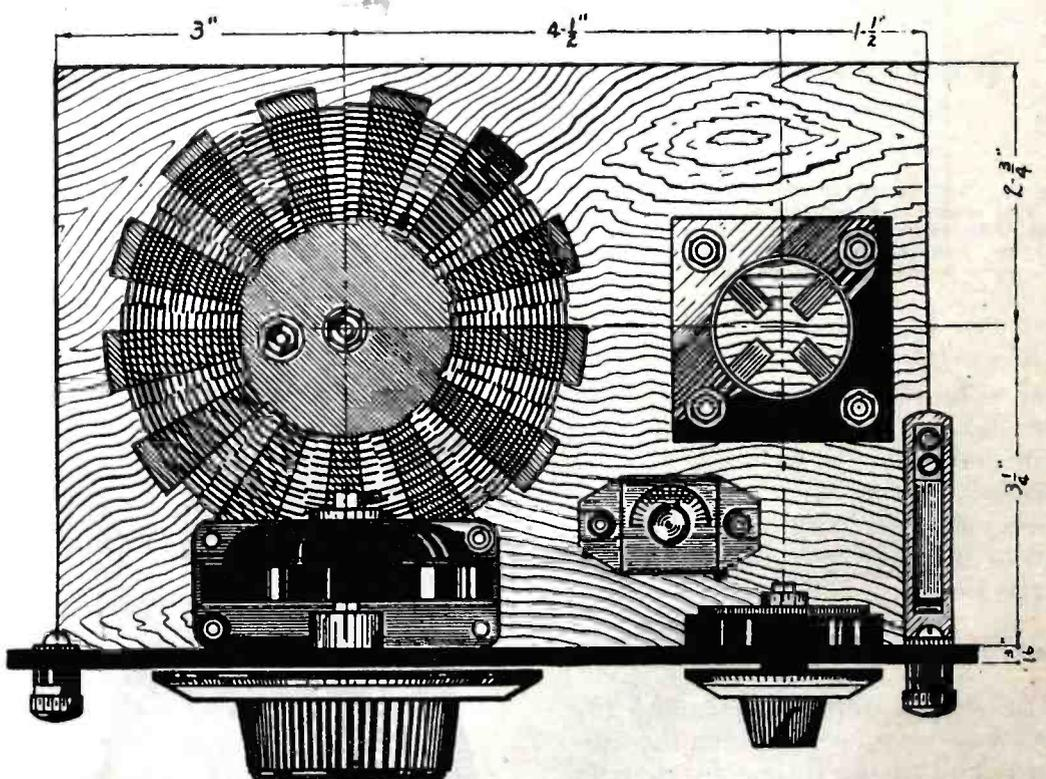
Fig. 2. Baseboard layout of the set with dimensions.
