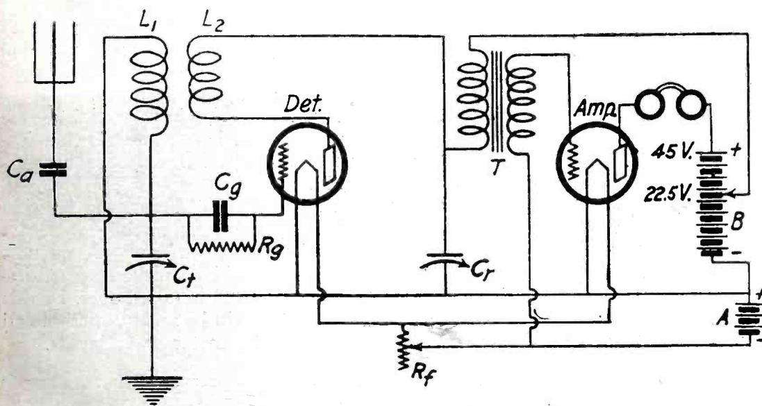
Schematic diagram of the 9XH-9EK short wave set No. III. See nomenclature at the right for parts.
