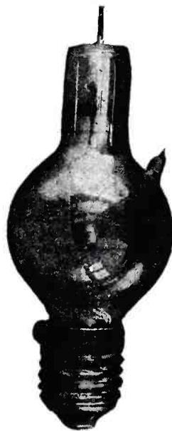
Fig. 12. A typical rectifier tube. The screw base allows it to be inserted in a standard lamp socket from which current is obtained for the filament. Connection is made to the graphite disc by means of a Fahnestock connector which clips on to the wire post projecting from the other end of the tube.
