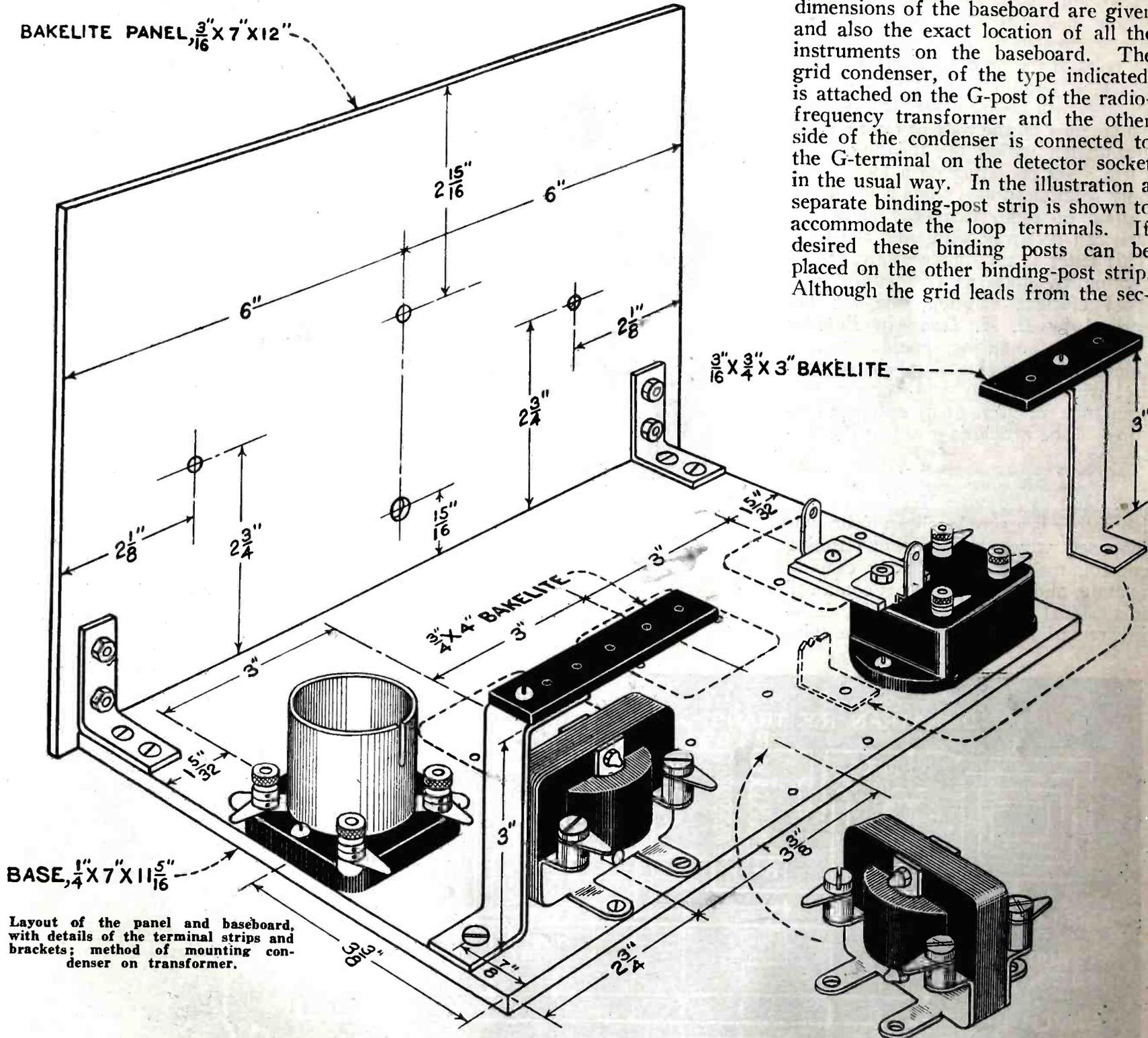
Layout of the panel and baseboard, with details of the terminal strips and brackets; method of mounting condenser on transformer.
