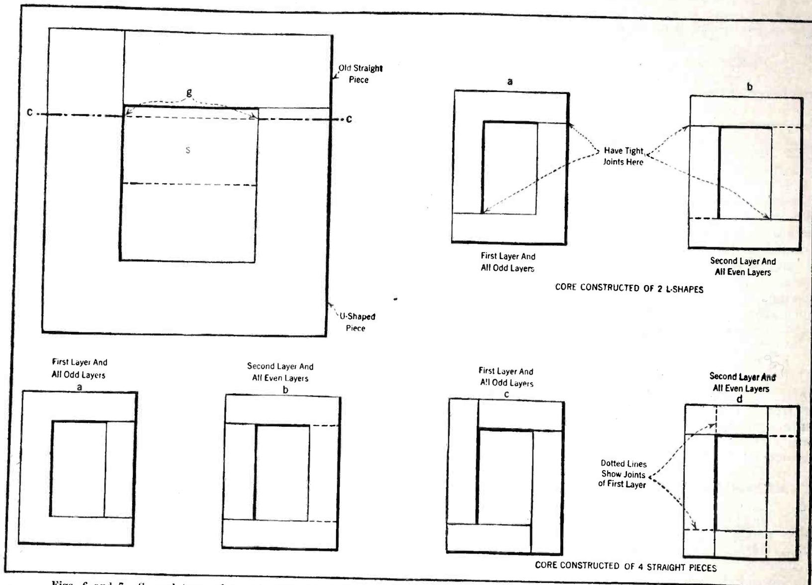
Figs. 6 and 7. Several types of transformer cores which may be employed in this construction. The sketches are self-explanatory.
