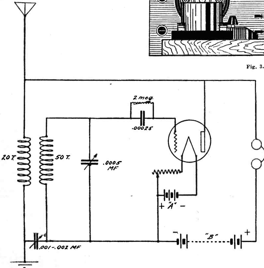
Fig. 4. Circuit diagram of the set.
