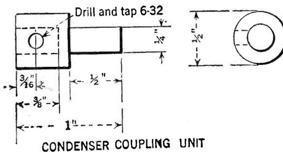
Fig. 8. To shield the condenser from body capacity effects it should be placed some distance from the panel and this coupling member enables the proper spacing to be carried out.
