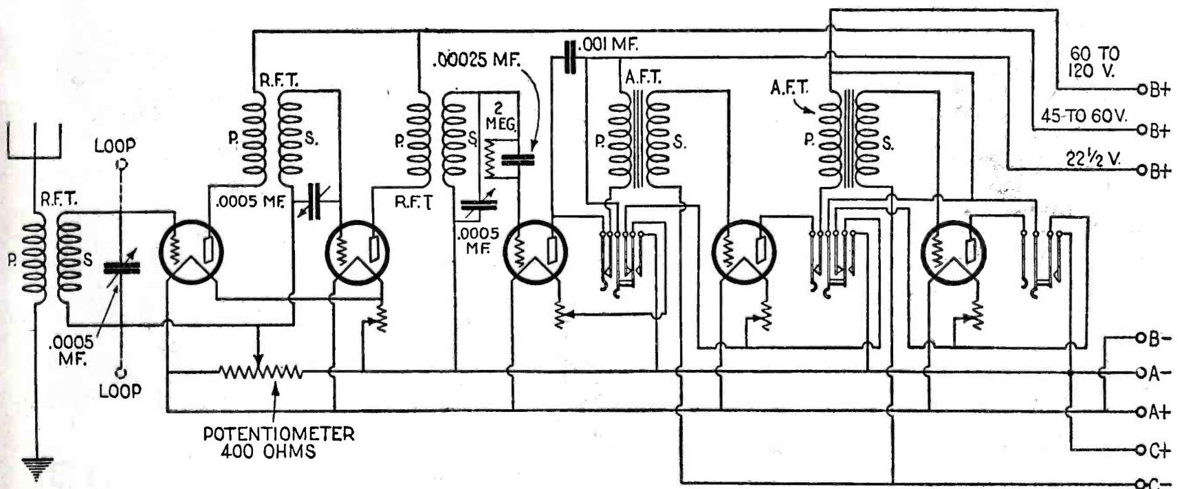
Fig. 1. Circuit diagram for receiver that has a wave-length range from 40 to 555 meters.
