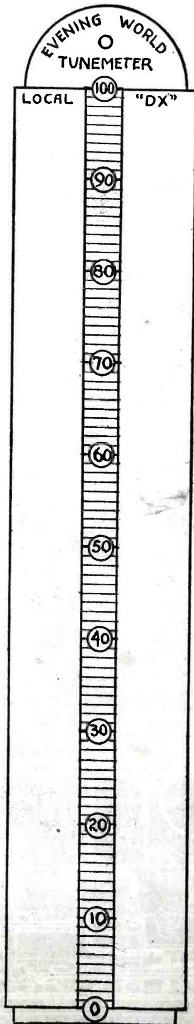
The log as illustrated can be used not only for one-dial sets, but also for others, as in most cases the main tuning, so far as station logging is concerned, is done with one dial.
