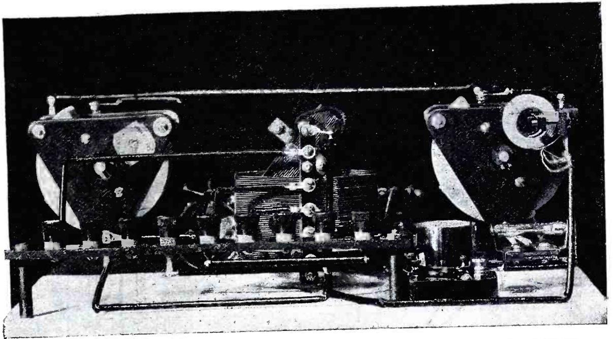
Fig. 9. This rear view shows clearly the disposition of the coils and other apparatus. Note how the oscillator coils are clamped between the two bakelite strips which are fastened to the oscillator condenser.
