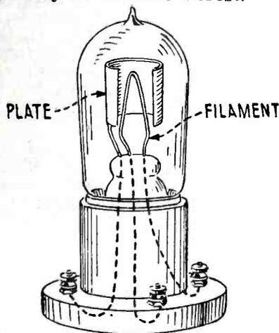
Fig. 1. The Fleming valve, which contained but two elements; i. e., filament and plate. It was the forerunner of the modern vacuum tube.
