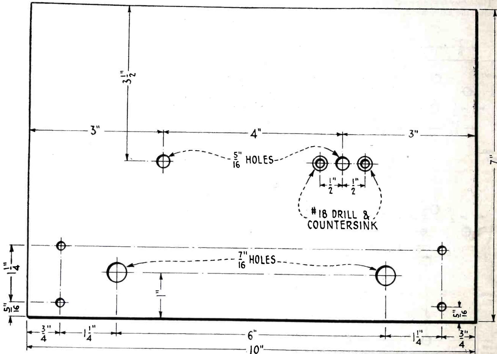
Front panel layout of the amplifier with dimensions of the holes to be drilled.
