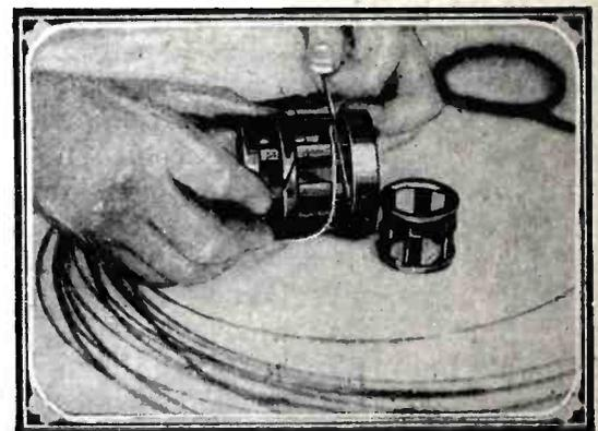
Winding the bare copper wire and the heavy cord side by side on the secondary section of the stator form.
