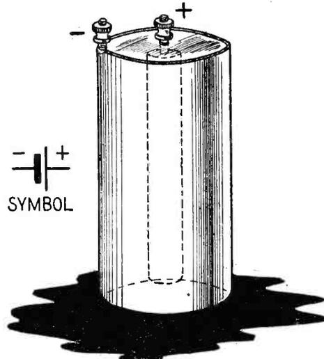
Dry cell showing positive and negative electrodes.
