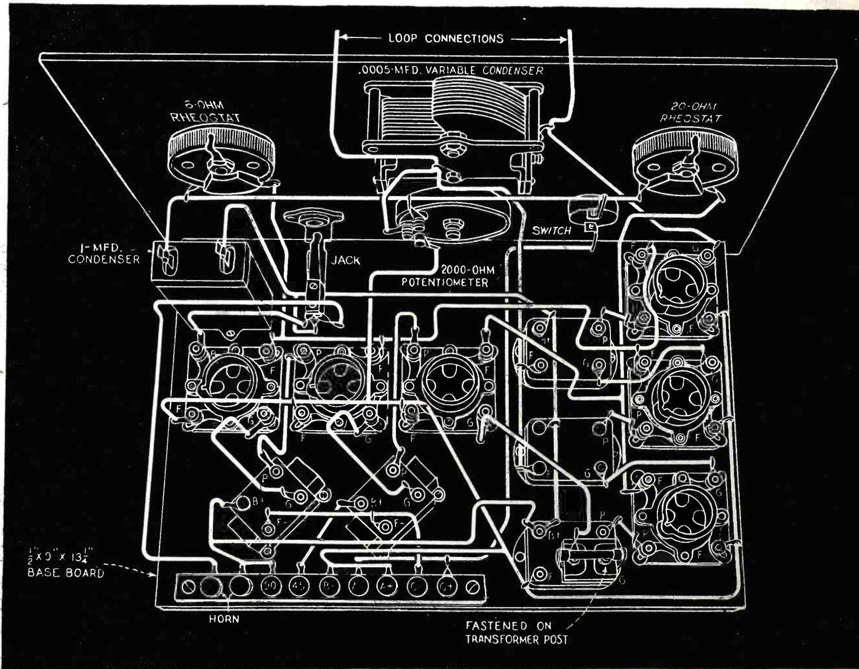
The above shows the complete assembly and wiring of the six-tube self-contained loop set. The binding posts on the insulating strip are connected as follows: Reading from the left—First two, loud speaker; third, 90 volts + "B" battery; fourth, 45 volts + "B" battery; fifth, "B" battery —; sixth, "A" battery — 4 1/2 volts; seventh, "A" battery +; eighth, "C" battery — 4 1/2 volts; and ninth, "C" battery +.
