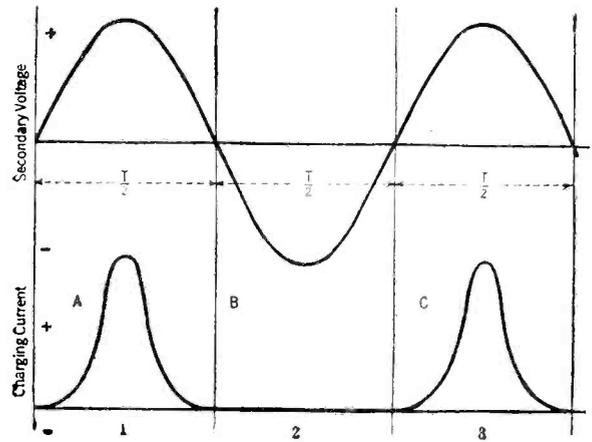
Fig. 1. A graphic representation of how a charger functions. The curve labeled "secondary voltage" shows the sine wave-form of the 60-cycle lighting circuit. That curve labeled "charging current" shows the portion of the alternating wave which is rejected in the rectifier allowing only the periodic pulsations of that portion of the curve where the current is "direct current" to enter the battery.
