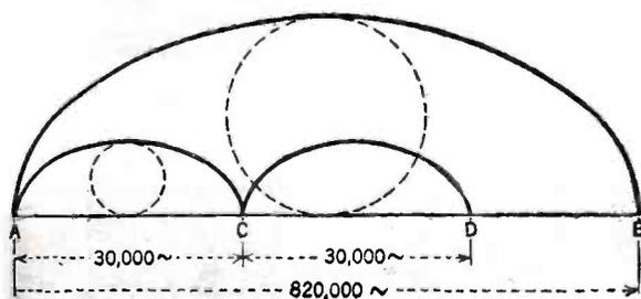
Fig. 1. The broadcasting band of frequencies is 820,000 cycles wide and is represented here by taking a point on the circumference of a wheel and marking out its path as it rolls along the frequency line. At the end of one complete revolution the point has traversed 820,000 cycles. The smaller wheel representing the oscillator dial traces a similar path but in one revolution it traverses only 30,000 cycles. There are two points 60,000 cycles apart that a given station may be heard.
