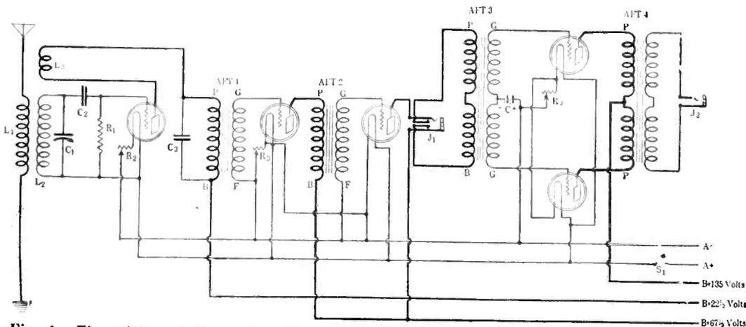
Fig. 1. The wiring of the push-pull audio set. Photos of the completed set are shown in Figs. 1A, 2, 3 and 4.
