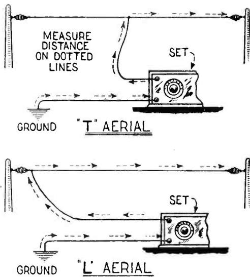
Method of measuring the fundamental wave-length of "T" and inverted "L" types of aerials.
