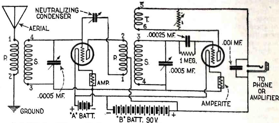
Q. 22 (Fig. 1). Revised "Baby Super Set" which permits neutralization. In this circuit using 201A tubes up to 90 volts may be used for detector "B" battery, but the correct amount must be determined by experiment.
