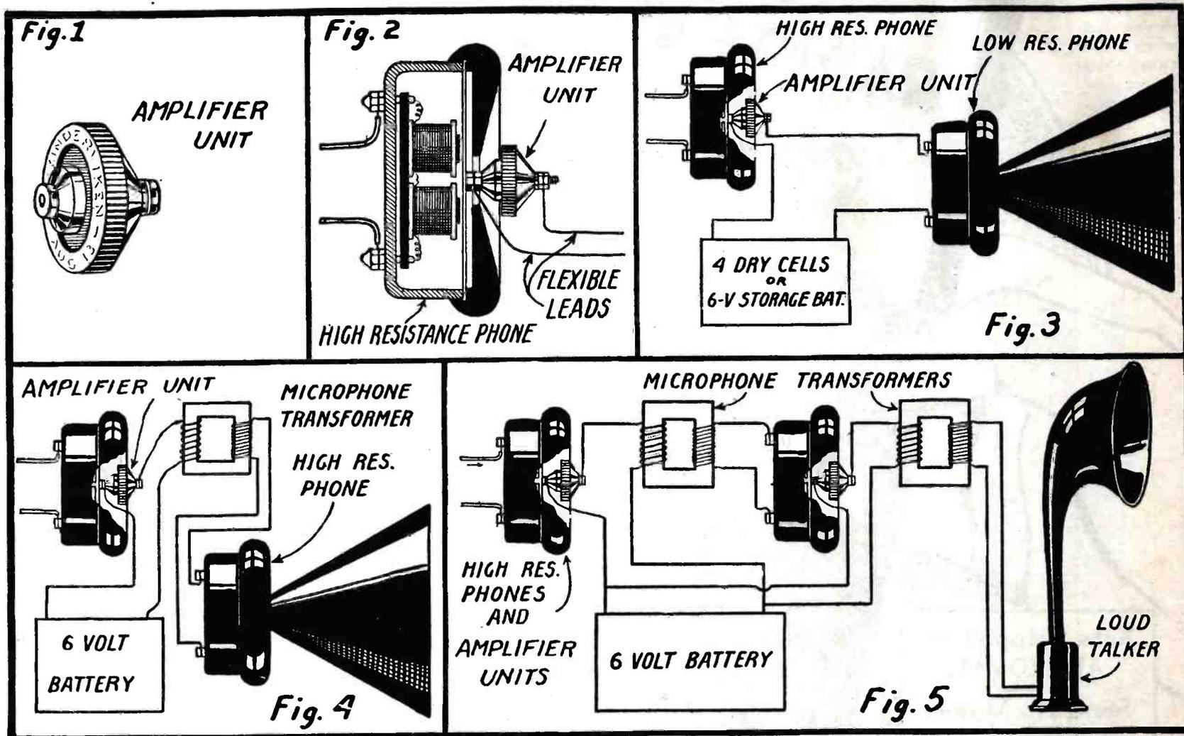
FIG. 1 shows the amplifier unit, actual size.
