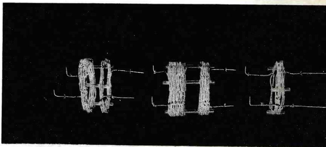
Coil systems removed from receiver.
