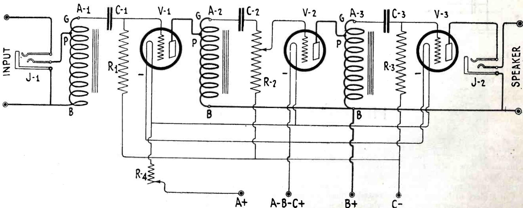
Schematic wiring diagram of the amplifier. Care should be taken to make all connections as shown, especially to the choke coils.
