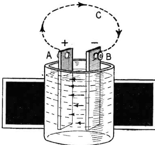
Fig. 1-A. A simple primary or electrolytic cell.
