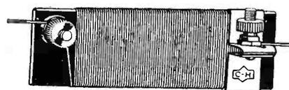
Illustration by Courtesy of The Cutler-Hammer Mfg. Co. Fig. 4. Resistance used in series with a rheostat having a small resistance in order to enable its use with tubes requiring less current.
