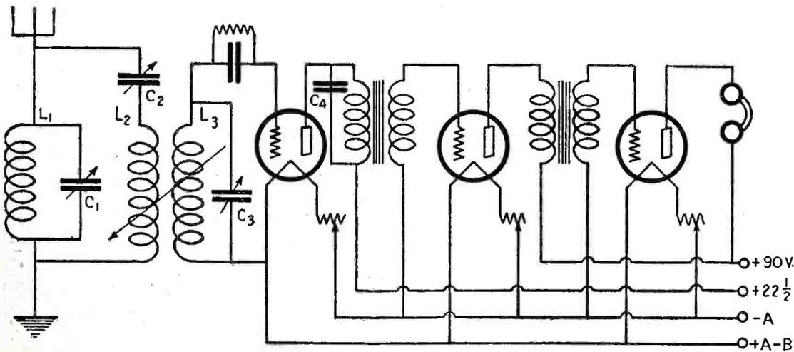
Q. 2. A three-tube set incorporating the principle of the Selector Tuner.
