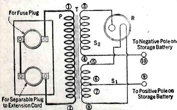
Fig. 3. The actual circuit diagram of the Beers tungar rectifier. This is different from that of the charger circuit in Fig. 10 in that a separate charging secondary is provided. Alternating current is induced into this secondary while the circuit in Fig. 10 is that of an auto-transformer employing the conductive system. There is no great difference between the two.
