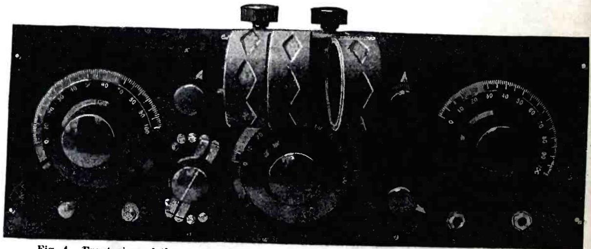
Fig. 4. Front view of the completed receiver. The two honeycomb coils to the left function as a tuned radio frequency transformer.
