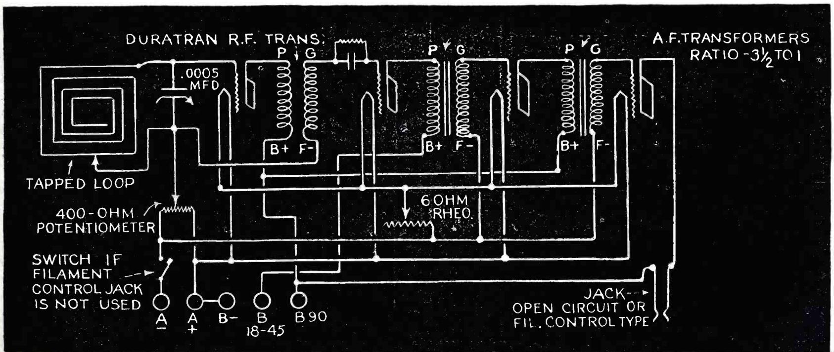
Schematic diagram of the set. Note the tapped loop employed. This loop is of the Lincoln or Nazeley type.
