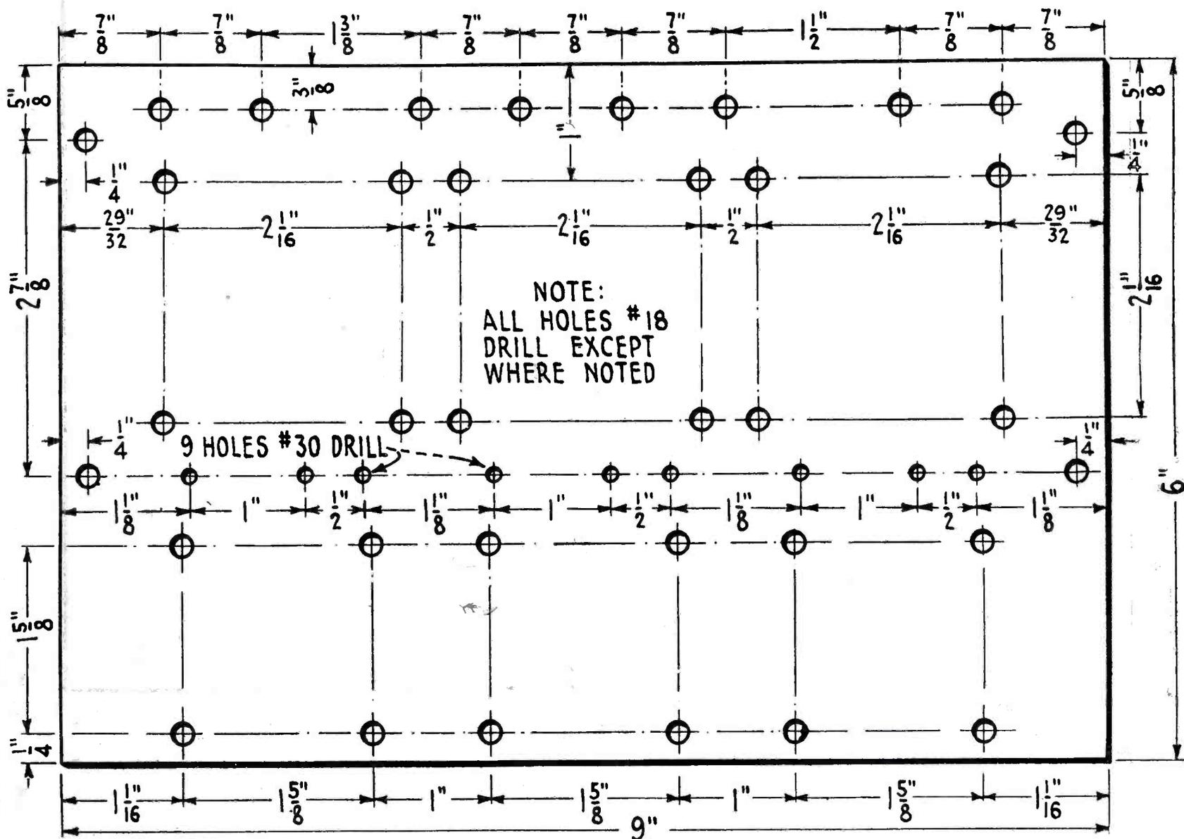
Details for drilling the bakelite or hard rubber sub-panel on which the three choke coils, sockets and binding posts are mounted. Note how the sockets are mounted in the accompanying photo. All connections are made beneath this sub-panel.
