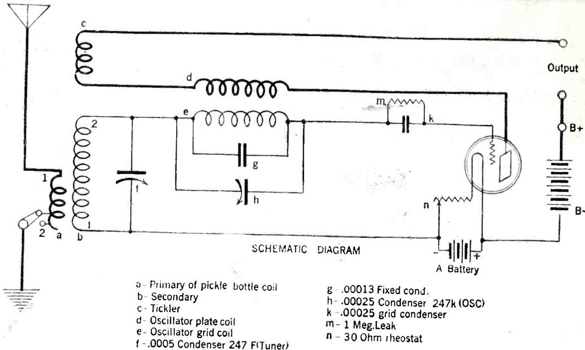
Fig. 4. The Schematic diagram of the frequency changer showing the Armstrong system of securing local oscillations in the first detector tube.
