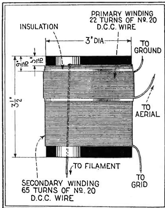
Q. 14 (Fig. 1). Radio frequency tuner for "Baby Super Set."
