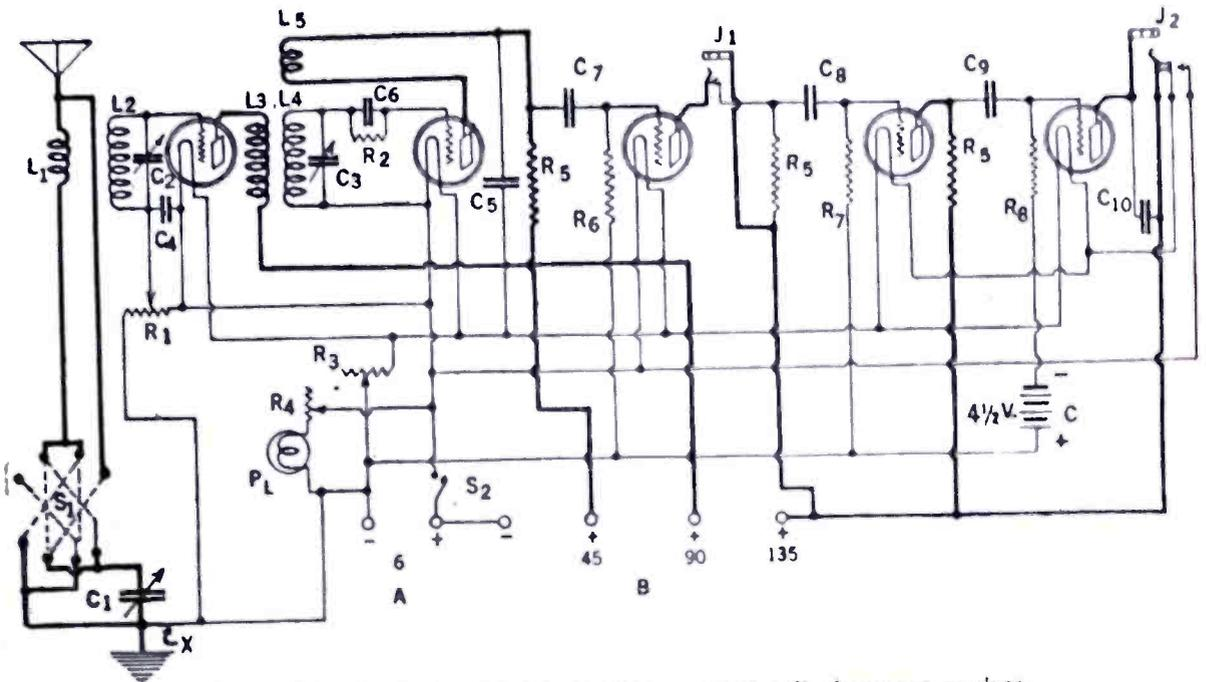
Fig. 1. The circuit diagram for the all-wave tuned radio frequency receiver.
