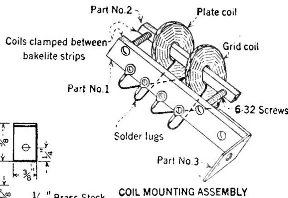
Fig. 10. The details of the oscillator coupler are shown in this figure. Small coils placed at some distance from their tuning condensers decrease the external field and the resultant coupling effects to other parts of the circuit.
