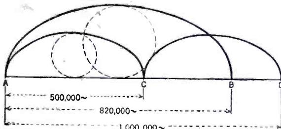
Fig. 2. By making the smaller wheel much larger, the path a given point on its circumference would trace out is longer. Before it completes two revolutions however, it is outside the broadcasting band, and for this reason there will be only one point on the oscillator dial where a given station will be heard.
