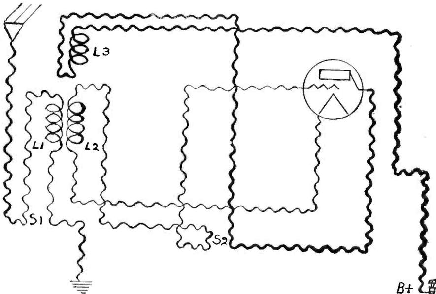
Fig. 3. This diagram shows course of waves through the circuit in Fig. 1 when used on broadcast range.
