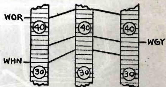
How a three dial set can be logged. Three calibrated strips are numbered to correspond to the divisions of the dials. Thus, the dial settings for each station can be logged as shown.
