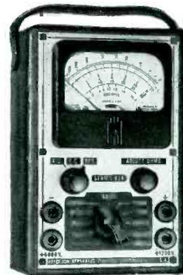
12/60/300/600/1200/6000, and 4 current ranges of 1.2/12/60/600 mils. Resistance ranges are 0-5000/500M/5 Megs. Also 6 db ranges from -10 to +70. All measurements from only two pin jacks except 1200 and 6000 volts. New type large 400-microampere rectangular meter. Overall size is 7" x 4½" x 3". By Precision Apparatus Co., 647 Kent Ave., Brooklyn, N. Y.
