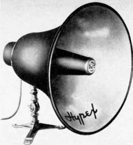
Projector with driver unit and stand. Used for general sound reinforcement work where principle requirement is good speech reproduction. Horn is the re-entrant type.
