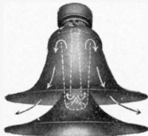
Radial Horn Speaker—a re-entrant type employing sound-reflection to foreshorten length of horn for given length of sound travel. Distributes sound, with even intensity, downward with 360° radius.
