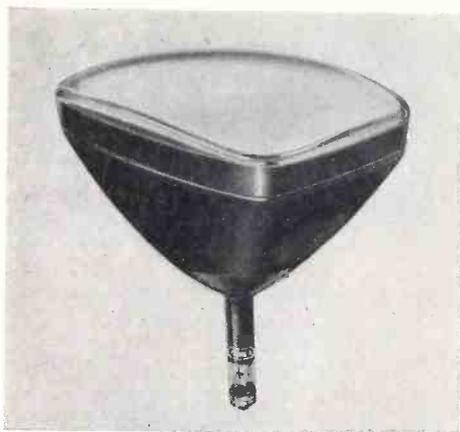
glass to provide increased picture contrast; employs magnetic focus and magnetic deflection; has an in-built capacitor formed by the internal and external conductive coatings to serve as a supplementary filter capacitor for the high-voltage supply; and utilizes an ion-trap gun requiring only a single-field, external magnet. The 17EP4-A has a diagonal deflection angle of  $70^\circ$  and a horizontal deflection angle of  $65^\circ$ .
