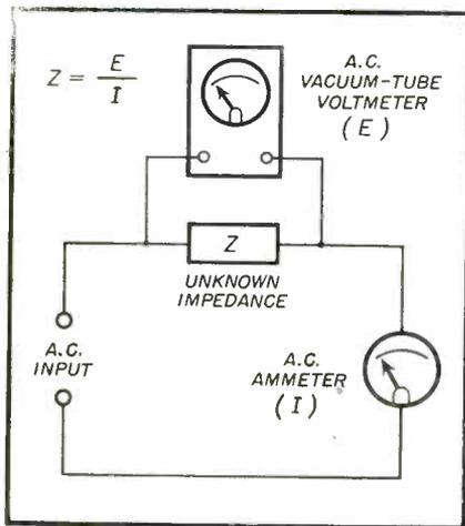
Fig. 2—Connections for the Volt-Ammeter method of Z measurement.
