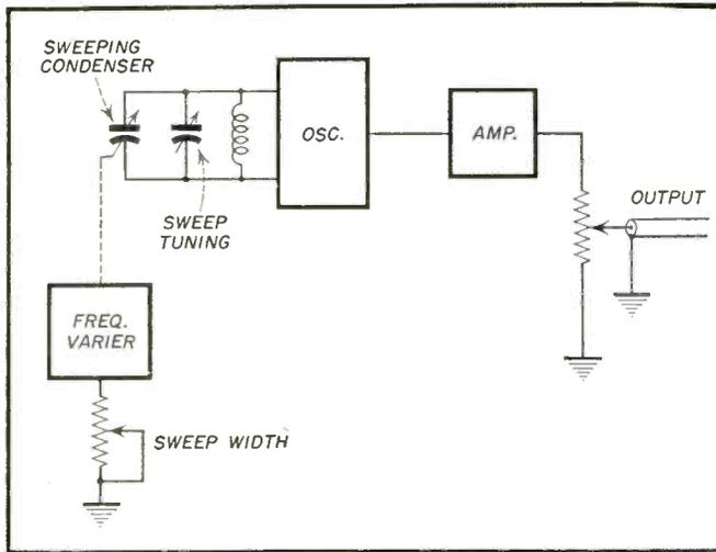
Fig. 2—Sweep Generator block diagram showing Oscillator, Sweep, Amplifier and Output.
