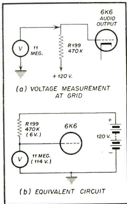
Fig. 4—Effect of meter on R.
