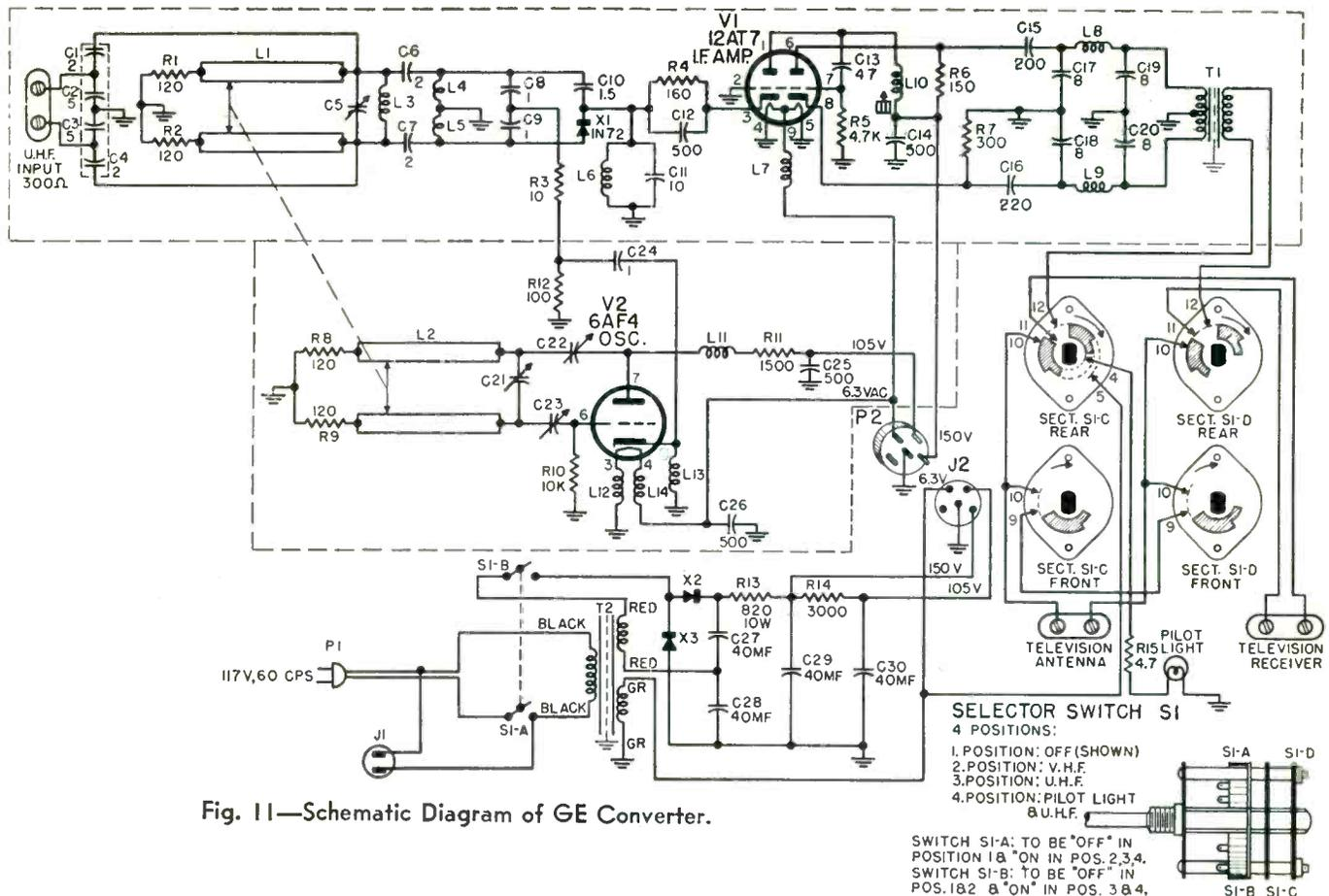
most UHF conversion systems, there is no rf amplifier. A 12AT7 is used as the if amplifier; the input is to the cathode on pin 3. The grid of this section is at ground potential and it operates as a grounded grid amplifier. The plate output is capacitively coupled to the grid of the second amplifier on pin 7. Output is taken between plate and cathode and inductively coupled to the 300 ohm output going to the standard television receiver.
