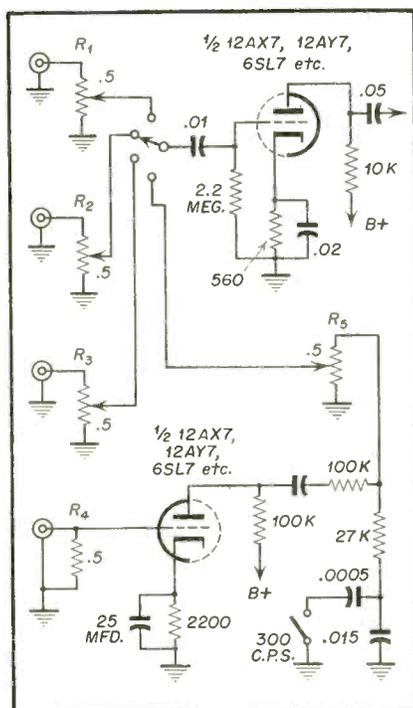
Fig. 1—Shown above is the input-selector section of a high-quality amplifier. The switch at lower left marked "300 cps" changes the turnover point (bass boost) of the phono preamp. Selector switch is shorting type to prevent loud switching noises in speaker.
