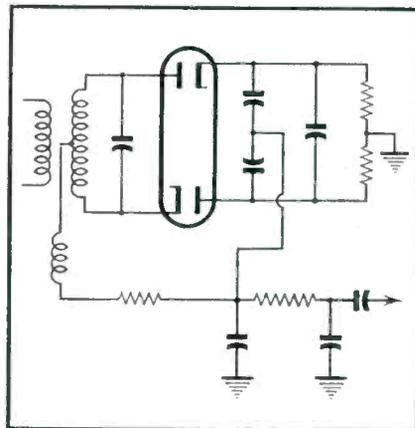
Fig. 8—Ratio detector schematic.
