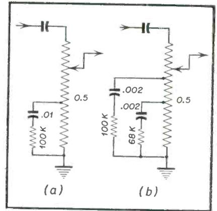
Fig. 4 (a)—Above left is shown a volume control employed by RCA for many years on most of its radios. Actually a simplified "loudness control," it was surprisingly effective. 4 (b) is the same sort of circuit, and is employed by present-day makers of many high-quality audio amplifiers to provide superior Fletcher-Munson compensation.
