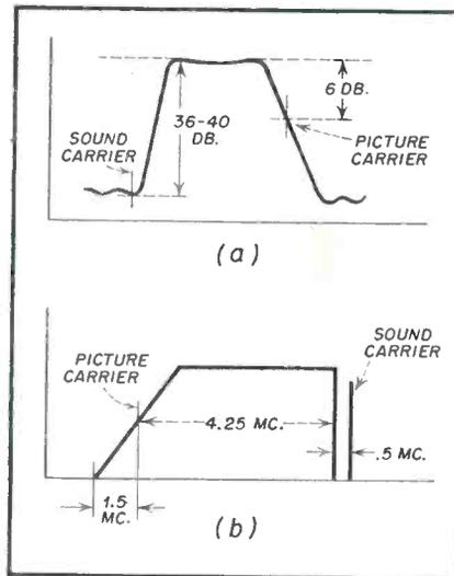
**Fig. 1—**a. Actual I-F curve. b. Ideal I-F composite curve.
