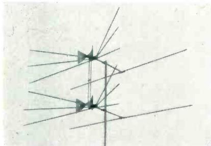
The Stacked Ultra Fan was designed to eliminate the "Twin Terrors" of UHF: vibration, and the accumulation of dirt and moisture at the terminals. The terminals of this antenna are isolated in free space, preventing the accumulation of dirt and moisture which can dim or short out the picture completely. The filters also have "free space" terminals.
