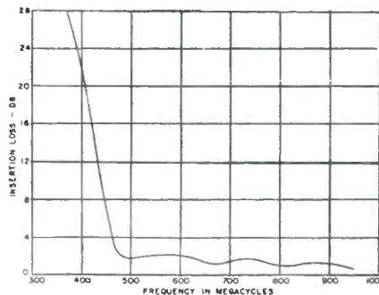
Fig. 19—High pass filter characteristics of RCA tuner.
