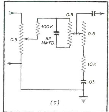
Fig. 4 (c)—This is the schematic of a continuously-variable loudness control which may be purchased in kit form (IRC) at most jobbers. It is easy to construct and very effective.
