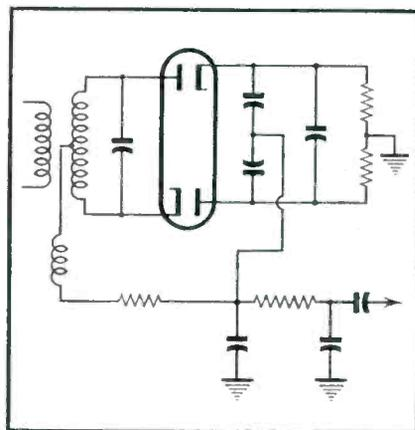
Fig. 8—Ratio detector schematic.
