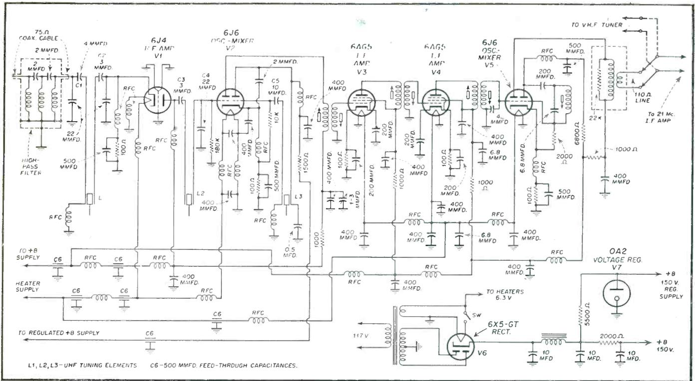
Fig. 18—RCA U-H-F Tuner schematic.
