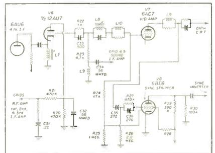
Fig. 3—Conrac video detector, agc, and sync stripper.
