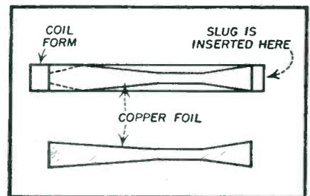
Fig. 20—Detail of U-H-F tuning element used in RCA tuner.
