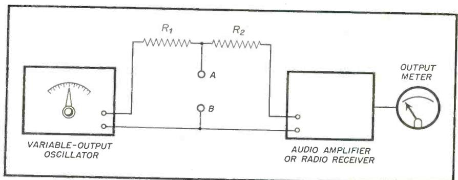
Fig. 4—Set up for measuring Z by the Network method.
