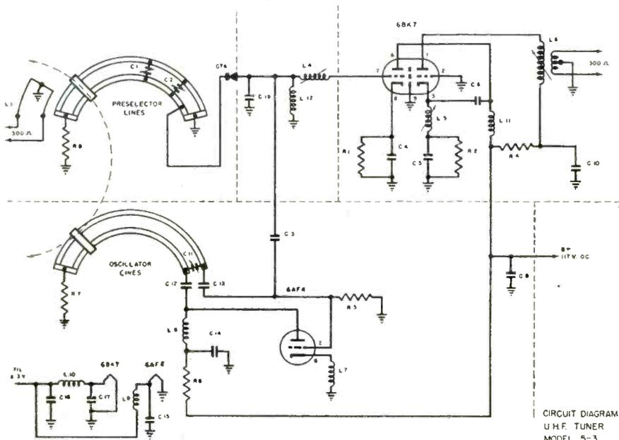
Fig. 14—Schematic of Kingston Converter.
