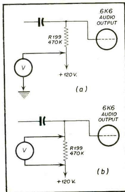
Fig. 5—Measuring grid voltage with low resistance meter.
