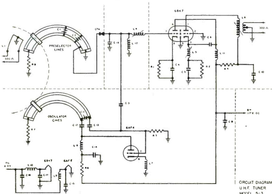
Fig. 14—Schematic of Kingston Converter.
