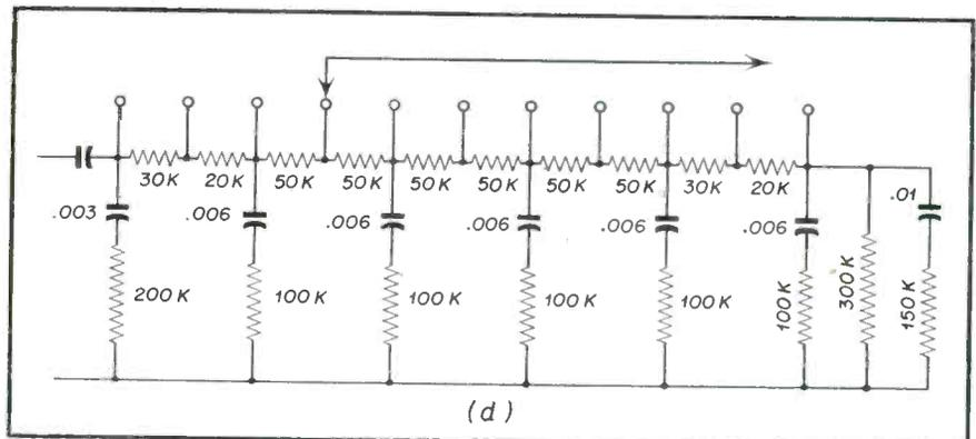
Fig. 4 (d)—This is the most elaborate sort of loudness control. It provides rather complete compensation for ear-loss at lower volume-lower frequencies. Its advantages are cost (many parts) and the fact that it has steps instead of smooth variation.
