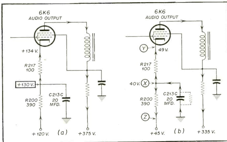
Fig. 6—(a) Normal path for current flow. (b) Current flow through cathode resistors with C213C leaky.
