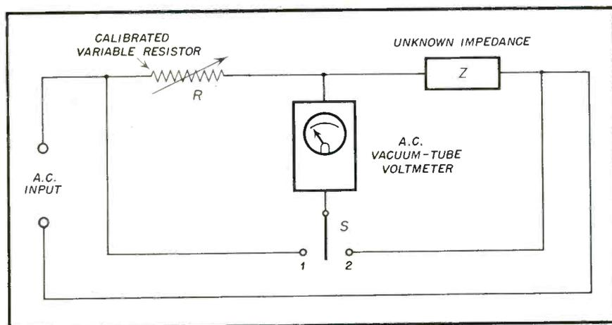
Fig. 5—Series-Resistance method—Set up pictured in Fig. 1.
