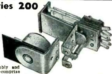
Two basic parts—a coil assembly and a contact switch assembly—comprise this simple, yet versatile relay. The coil assembly consists of the coil and field piece. The contact assembly consists of switch blades, armature, return spring and mounting bracket. The new Guardian Midget Contact Assembly which is interchangeable with the Standard Series 200 coil assembly, is also available in either single pole, double throw; or double pole, double throw.
