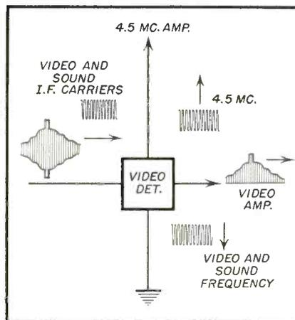
Fig. 4—Block diagram of intercarrier video detector inputs and outputs. As a result of the detector action the incoming video and sound carriers beat against each other, producing a separate 4.5 mc FM sound signal and a demodulated video signal.
