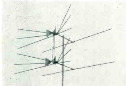
The Stacked Ultra Fan was designed to eliminate the "Twin Terrors" of UHF: vibration, and the accumulation of dirt and moisture at the terminals. The terminals of this antenna are isolated in free space, preventing the accumulation of dirt and moisture which can dim or short out the picture completely. The filters also have "free space" terminals.
