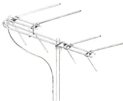
Coverage of all uhf channels, uniform gain of 8 db across the band, low vswr and 300 ohm impedance are electrical features. It has a sharp directional pattern, too, to cut down the critical uhf ghost problem. Small—about two feet by two feet; light weight—less than two pounds; and completely preassembled, it is all aluminum construction. Two and four stack models are also available.
