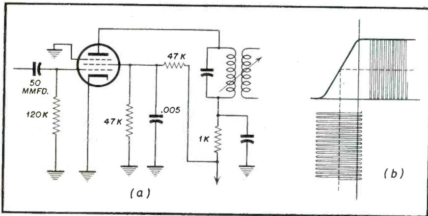
Fig. 6—Limiter action and schematic.
