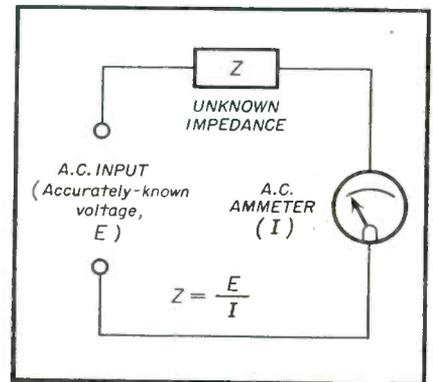
Fig. 3—Connections for Ammeter method of Z measurement.
