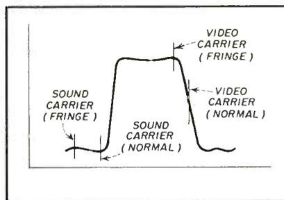
Fig. 5—I.F. signal showing the drift and fringe limits. In split-sound receivers sound drift results as the local oscillator drifts in frequency.
