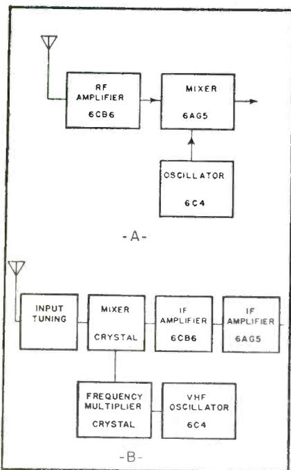
Fig. 17—Block diagram of Zenith System.
