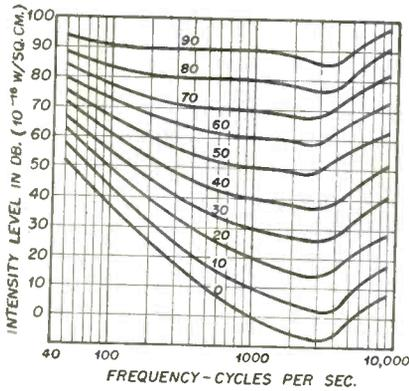
Fig. 3—Fletcher-Munson curves indicate the amount of boost needed at various listening levels to give the same apparent strength to different frequencies as would be heard (by the average ear) if the sounds were played at concert-hall levels.
