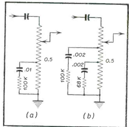
Fig. 4 (a)—Above left is shown a volume control employed by RCA for many years on most of its radios. Actually a simplified "loudness control," it was surprisingly effective. 4 (b) is the same sort of circuit, and is employed by present-day makers of many high-quality audio amplifiers to provide superior Fletcher-Munson compensation.
