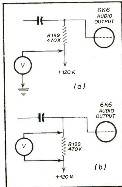
Fig. 5—Measuring grid voltage with low resistance meter.
