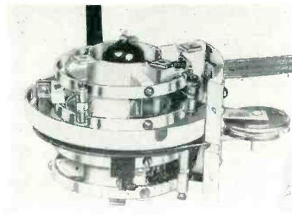
Fig. 15—Kingston Converter with cover plate removed.
