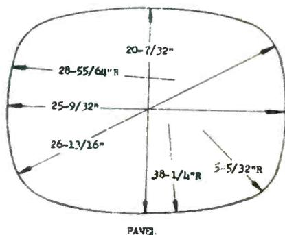
Physical dimensions of Hytron's new 27EP4 CRT.
