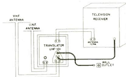
Fig. 10—Connections for wiring GE U-H-F converter to TV receiver.
