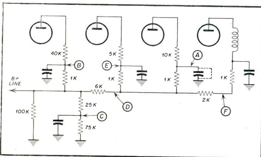
Fig. 3—Resistance readings are: (B+)-7K, (B)-8K, (C)-23K, (D)-1K, (E)-2K, (F)-3K, and (A)-150 ohms.
