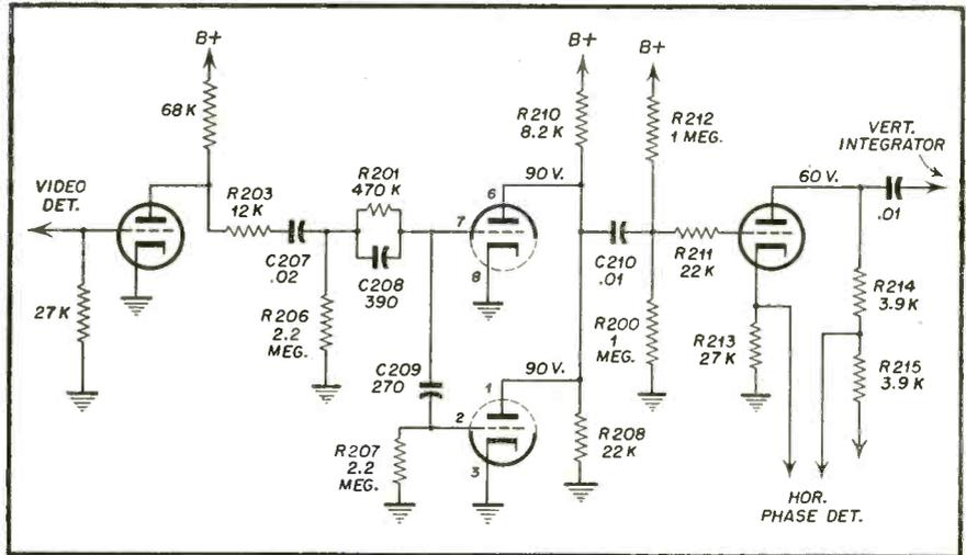
Fig. 1—Separate sync amplifiers used in C.B.S. Columbia Models 817, 820.
