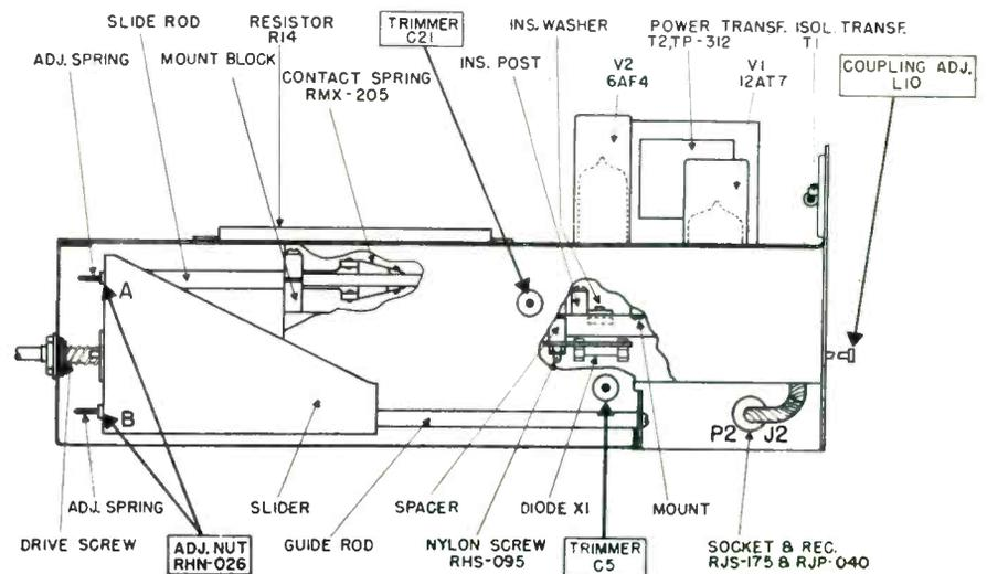
**Fig. 12—Tube, trimmer and component location of GE Converter.**
