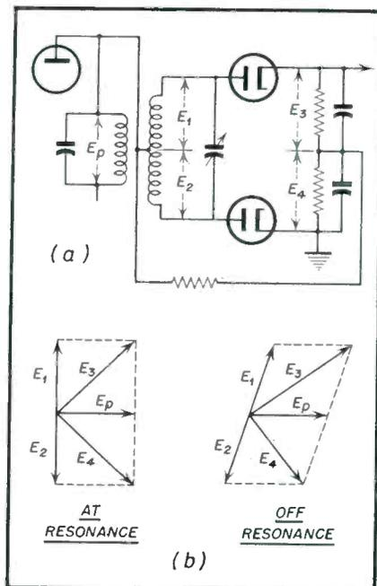
Fig. 7—Discriminator diagram with vector analysis of action.
