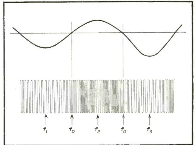
Fig. 3—Relation between Sine Wave modulating signal and F.M. output signal.
