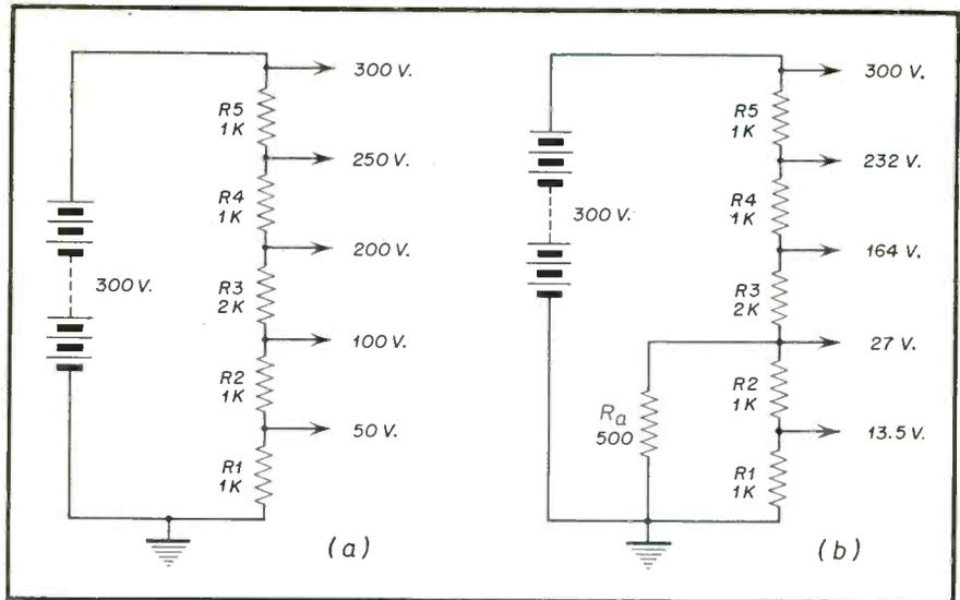
Fig. 2—(a) Simplified series voltage divider circuit. (b) Restribution of voltages caused by partial short.
