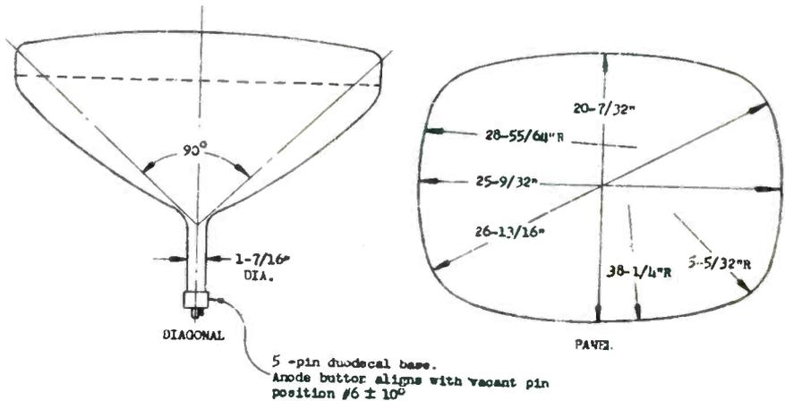
Physical dimensions of Hytron's new 27EP4 CRT.
