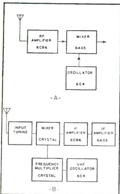
Fig. 17—Block diagram of Zenith System.
