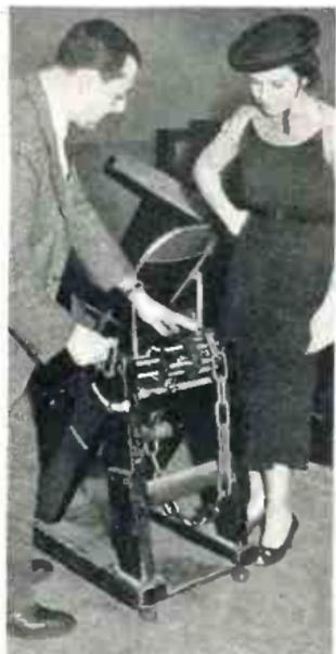
This is called a chain windlass machine. As the crank is turned, heavy chains make noises like those of a docking ship or ferry.
