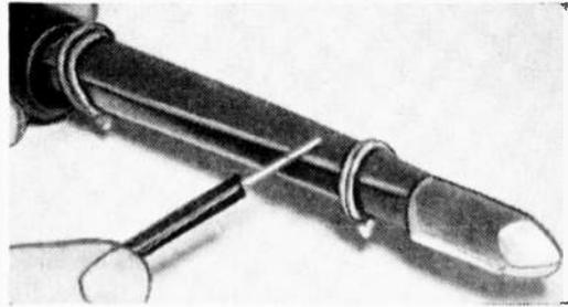
• Quite often a small file is needed to file corroded parts and wires clean before the application of solder. If you want to eliminate the necessity of hunting up such a file every time you have a soldering job to do, attach one to your iron's barrel with heavy solid wire. (You may have to break off the file's tang if it is longer than your iron's barrel.)—J.A.C.
