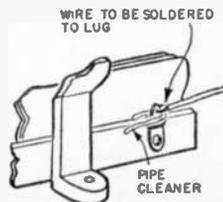
• For a neater job of soldering a wire or cable to a lug, build a dam around it with a pipe cleaner as shown. This idea is particularly good for automotive or radio jobs, where precision is necessary.—V. H. LAMOY.
