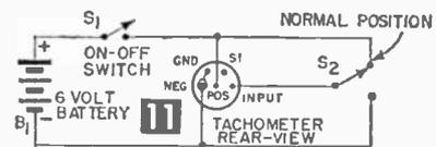
**CONNECTION FOR MOTORS, DRILL PRESSES, LATHES, ETC. WHERE PULSE IS SUPPLIED BY SHAFT-ACTUATED SWITCH.**
