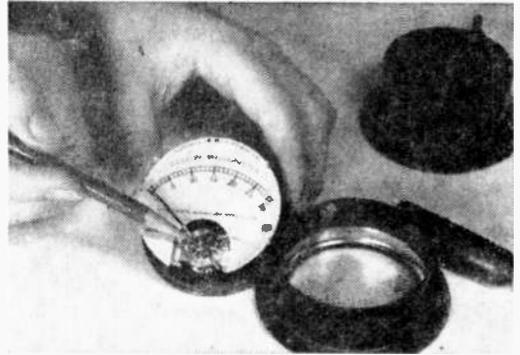
Pointing to pivot bearings, which, if broken, makes factory repair imperative.
