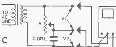
C CAPACITANCE OR INDUCTANCE (ADJUST "R" UNTIL V1 = V2)
