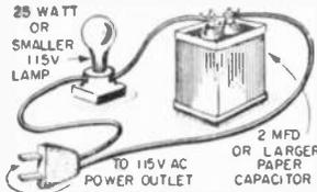
Now connect your capacitor in series with a cleat lamp socket and screw in a 25-watt, or smaller, bulb. When you connect the series combination to the ac power line, you will note that the bulb lights up, although not at full brilliance. Since the ohmmeter had just shown us that the capacitor is an open circuit, how, then, can the lamp light?
