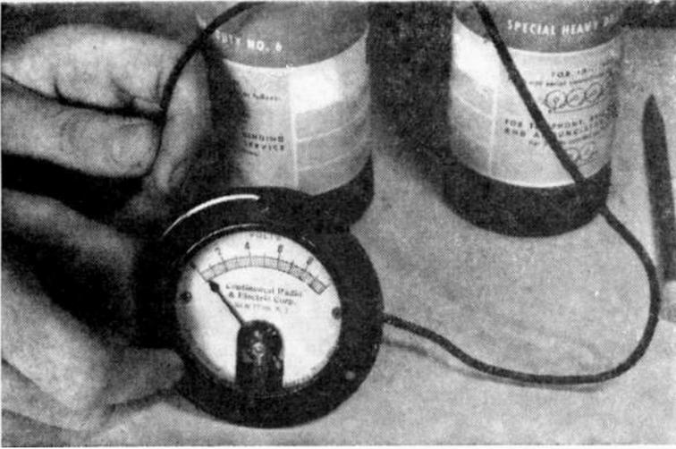
Voltmeter accuracy may be checked within reason by dry cell giving 1.5 volt readings.
