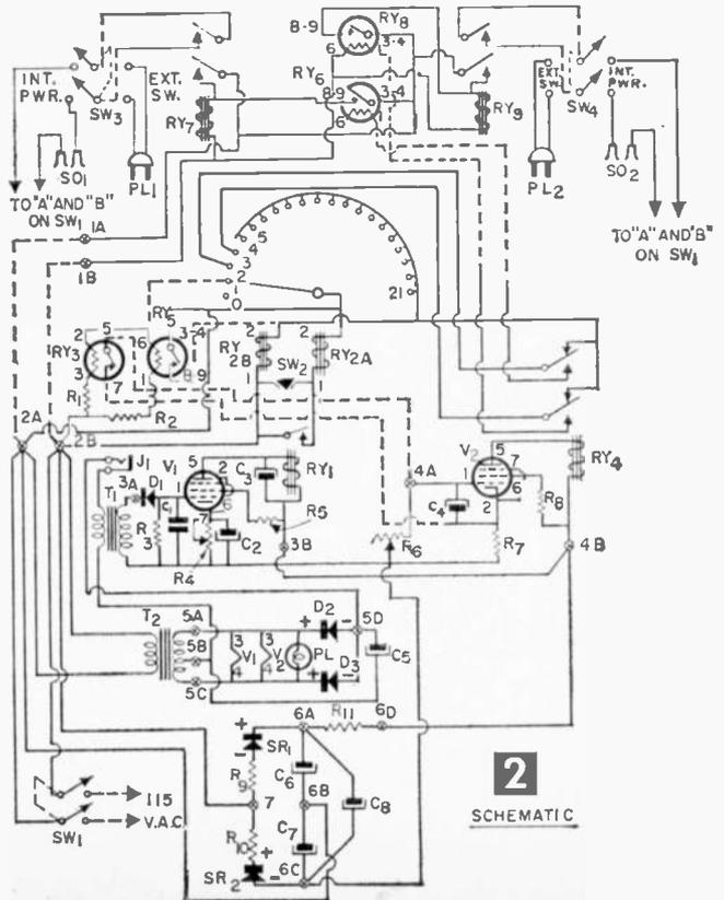
Ry5 starts cooling, having had insufficient time to close. If you hang up after the first ring on the second call, Ry2 remains on Position 2, which completes the circuit to the heater of thermal relay Ry6.
