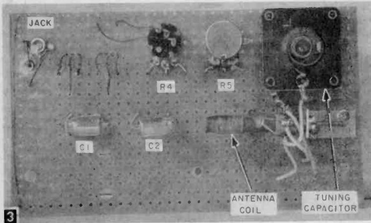
Back view of home-made lab kit circuit board.
