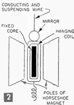
wire and fewer turns will work, too, with a slight drop-off in sensitivity.
