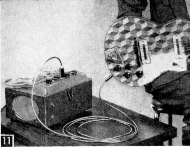
Here a small tape recorder (purchased second-hand for \$40) not only serves as an amplifier for the guitar, but also will record what you play if you want to hear it later—an invaluable method for improving your playing. And, an extension speaker plugged into that jack on the front of the recorder will give you some stereophonic effects.
