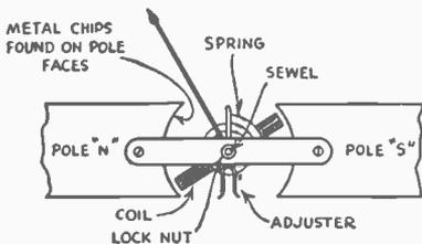
1 VITAL PARTS OF MOVING COIL VOLT METERS AND AMMETERS
