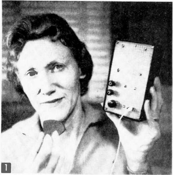
1 The utility amplifier can be used with a microphone as above or as a voltmeter audio amplifier.
