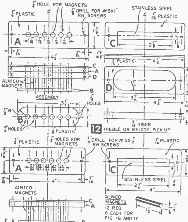
of six 1/4 in. dia. magnets 1 1/4 in. long by inserting the magnets through the 1/4 in. holes. Cement magnets in place with household cement.
