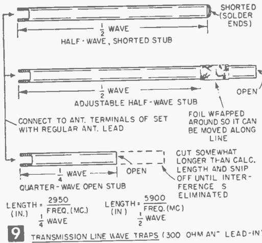
close to a TV channel frequency that an antenna filter might also filter out the desired signal, connect a simple filter or trap to the antenna terminals of the TV set (with the regular antenna lead). If you know the TVI frequency, make the filter of a section of 300-ohm antenna lead-in cut to exactly  $\frac{1}{2}$  the wavelength of that signal as in Fig. 9; solder the free ends of the stub together. If you don't know the TVI frequency, cut the
