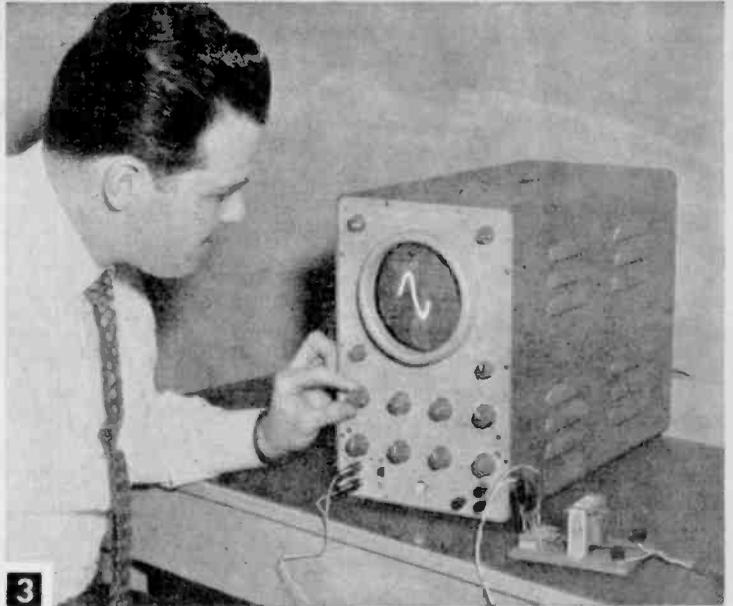
Testing the completed oscilloscope with a small step-down filament transformer. The sine wave shown in the above photograph is one cycle or two alternations of the 60 cycle current.
