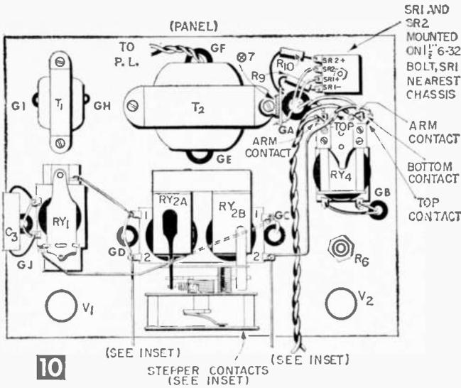
mentarily short Pins 1 and 2 of V2. The relay should close for over a minute with R6 at full resistance. Later, R6 can be adjusted for the exact time interval required.
