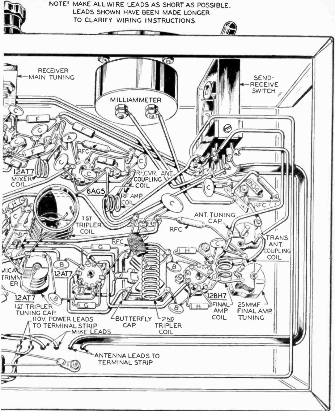
the receiver throughout its range. At some point on the dial the hiss should disappear. Turning the grid-dip meter off should cause it to reappear. If it does, the receiver is operative. If it doesn't, you'll need to recheck the wiring in the mixer and R.F. amplifier circuits only; the oscillator has been checked.
