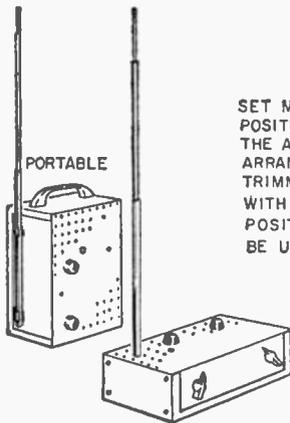
SET MAY BE USED IN EITHER OF POSITIONS SHOWN BY CHANGING THE ANTENNA MOUNTING ARRANGEMENT. THE ANTENNA TRIMMER SHOULD BE TUNED WITH THE ANTENNA IN THE POSITION IN WHICH IT WILL BE USED MOST FREQUENTLY
