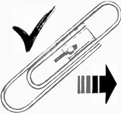
Nestled inside this paper clip—with room to spare—is a tunnel diode, one of last year's most startling electronics developments. If an FM receiver were rebuilt using one of the new diodes, all the conventional components shown at the right could be omitted.
