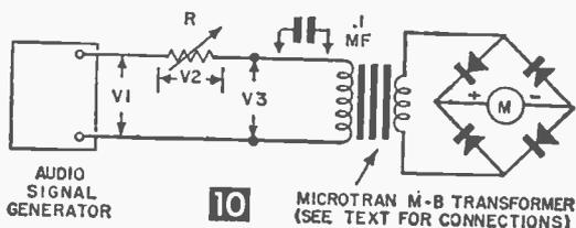
Method used for experimental verification of calculations:  $V_1 = 5$  volts;  $R$  (60,000 ohms) adjusted for full-scale deflection of  $M$ .  $V_2$  was 1.9 volts. Calculated value of  $Z_{in}$  is 103 K ohms, sensitivity is 33,400 ohms per volt using the measured values.
