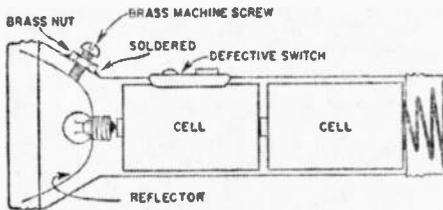
drilling a hole in the case close to the reflector, soldering a square or hexagon nut over the hole, and twisting a roundhead machine screw into the nut. To light the lamp, simply turn the screw clockwise until the end of the screw contacts the reflector. This provides the necessary connection from the case to the reflector, as the reflector is usually in contact with the lamp base but not the case. To turn off the lamp, back up the screw.
