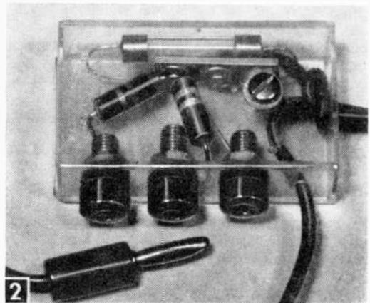
2 Complete adaptor, not including extension wire, fits into  $\frac{3}{4} \times 1\frac{1}{8} \times 2\frac{1}{2}$ -in. box and may be stored in car glove compartment.
