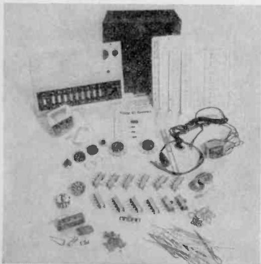
The components of the tube checker.
