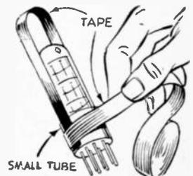
around the bottom with another strip of tape. Don't use tape on tubes that heat up excessively, because of the possible danger of fire due to tape igniting. *Never* use plastic tape for this purpose as it ignites easily.—J. A. COMSTOCK.
