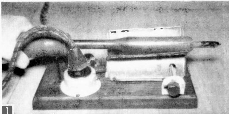
1 Thermostatically controlled stand regulates heat of iron through three levels— saves on electric bills!
