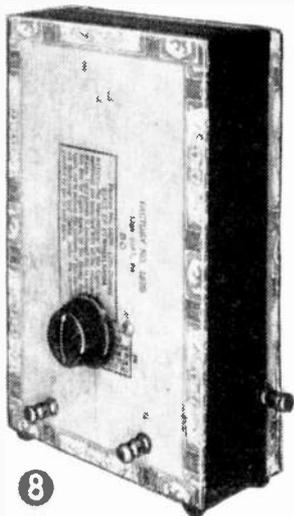
to antenna post and stator of variable condenser. The width of loop winding will be about  $1\frac{1}{4}$  in. with the turns spaced the diameter of the wire apart. Connect germanium diode cartridge from another variable condenser stator lug to left-hand phone binding post (Figs. 6 and 7). Mount a pointer knob or a graduated turning dial, on the variable condenser shaft, and tack or glue 4 small rubber bumpers onto the bottom of the cabinet. The set is now completed (Fig. 1).
