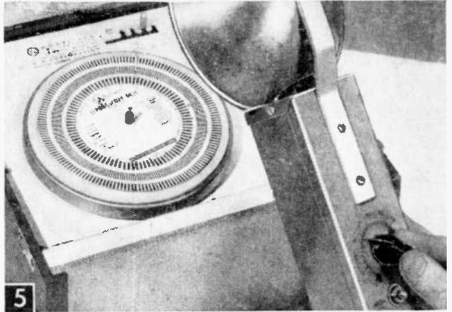
5 An ordinary record turntable and stroboscopic disc are used to calibrate your strobe light.
