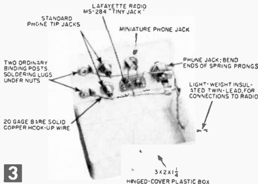
Holes in plastic box lid for mounting parts are reamed up to size with small knife blade. The jacks are wired in parallel, with solid copper hook-up wire.
