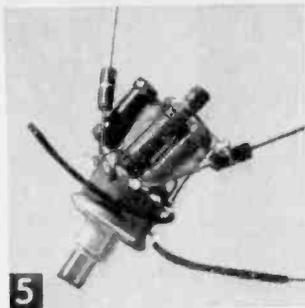
minal and the plus lead of C1 to the plus terminal of rectifier D. Place the negative lead of C1 under the negative terminal screw and solder the other two leads to the negative C1 lead. Connect one end of R9 to contact "C" of S2. Resistor R9 is made by folding 6½ ft. of #30 insulated copper wire on itself till it is 1 in. long. Insulate R9 with tape, and tape it to the meter case.
