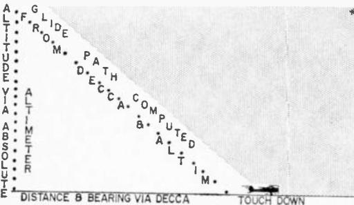
A control system incorporating DECCA—RAILS (Remote Area Instrument Landing System). Although the accuracy of this system is still being evaluated, chances are good it will enhance DECCA's overall superiority. At present it's only commercial use is in conjunction with the Bell helicopter service in the Dallas-Fort Worth area.
