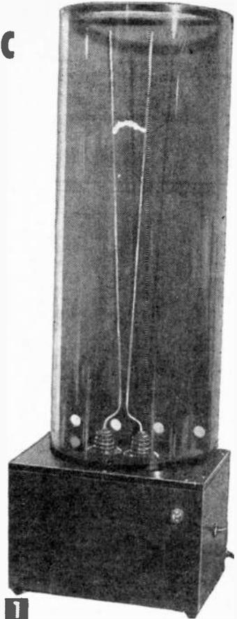
**1** A continuous series of flaming arcs will move up the electrodes of this device, which is similar to one shown at the Boston Museum of Science.
