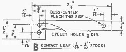
with the brass side of the armature from behind, and rivet the armature and bracket *lightly* together with  $\frac{1}{8}$ -in. diameter eyelets. Mount the armature assembly on the thermostat base with  $\frac{1}{4}$ -in. x 4-40 fh machine screws. Adjust the armature blades parallel with the armature base, and set the eyelets.
