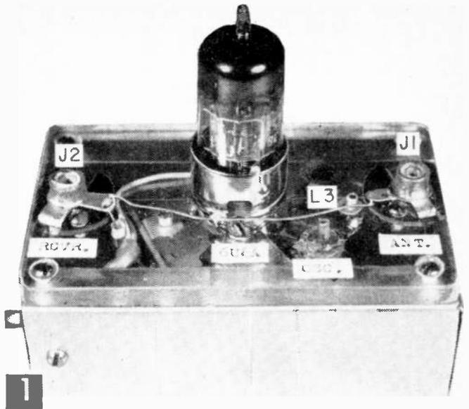
**T**HIS converter can be constructed with parts from most ham scrap-boxes, but even with new parts its cost will not run much over \$5! Naturally, with only one tube, it is not as hot as many commercial multi-tube units, but it will generally hold its own with crystal-controlled converters costing much, much more.
