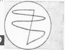
9 DOUBLE CYCLE PATTERN, WHERE FLASHING RATE IS TWICE OSCILLATOR FREQUENCY. USE FOR 10-20 C.P.S.
