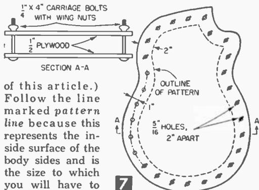
of this article.) Follow the line marked pattern line because this represents the inside surface of the body sides and is the size to which you will have to make the center
