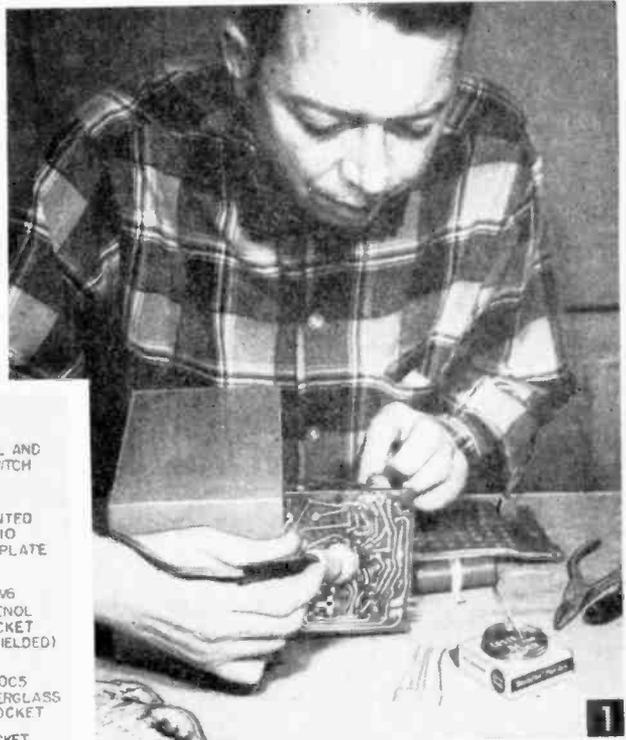
Many printed sets are vertically mounted in cabinet and slide out for quick circuit repair. Note that a fine-tip pencil iron, not over 40 watts, is used to prevent wiring damage.
