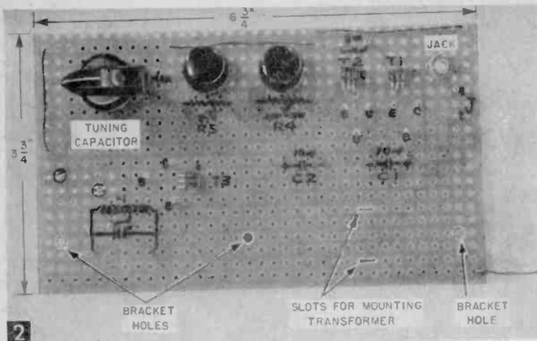
Front view of home-made lab kit circuit board.
