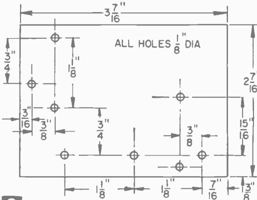
3 CIRCUIT BOARD LAYOUT (TOP VIEW)
