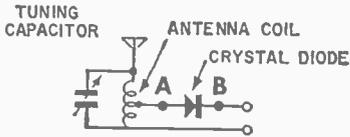
**E. SIMPLE TUNER CONNECTED IN PLACE OF MIKE IN 5B CONVERTS UNIT TO SIMPLE RADIO**
