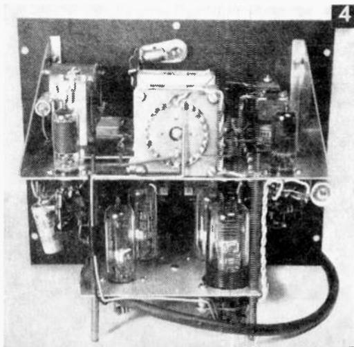
Back view of unit showing dual chassis construction.
