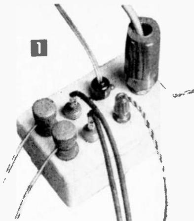
Built in less than an hour, this "Jack Box" accommodates five kinds of non-interchangeable earphone and speaker connections, permitting instant hookup of many combinations.
