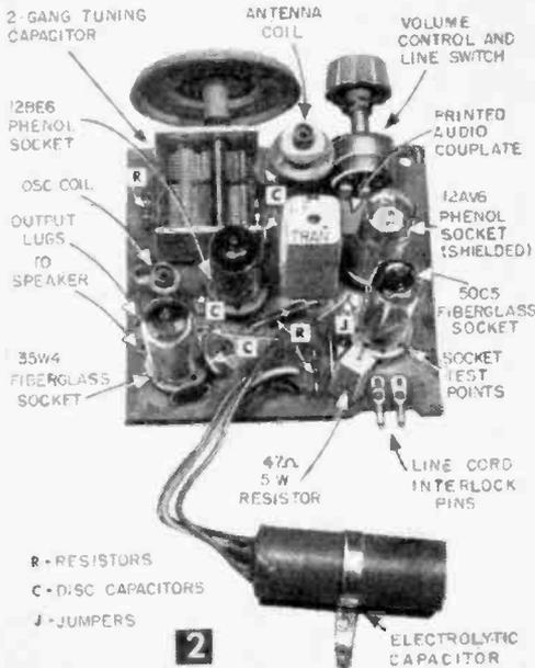
A typical "printed" circuit four-tube superheterodyne showing top of chassis. Note set is complete except for attachment of speaker and line cord. Strap of electrolytic capacitor is secured to a speaker mounting screw in cabinet.
