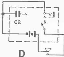
**D. KEY IN SERIES WITH BATTERY LEAD CONVERTS UNIT OF 5C TO CODE PRACTICE OSCILLATOR**
