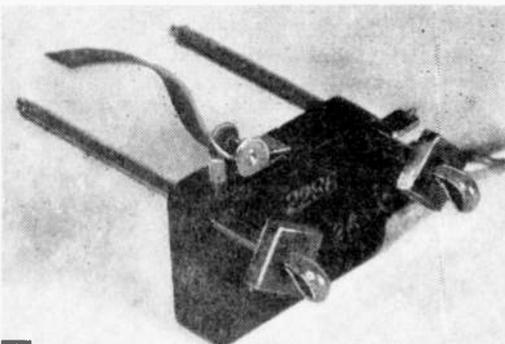
6 Micro-switch with cotter pins and nuts ready for mounting on phone.
