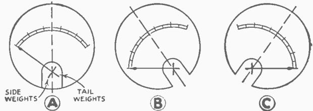
2 HOW TO BALANCE METER POINTER,
