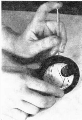
ing. We are here dealing only with moving coil meters inasmuch as they are by far the most common type in use today for direct current. For A.C. we have the moving iron meter which is also relatively simple and can be easily repaired in many instances. Where major damage has been done, and this is evident by examination, then the owner of the meter had best give up the job or send the meter back to its maker for rehabilitation.
