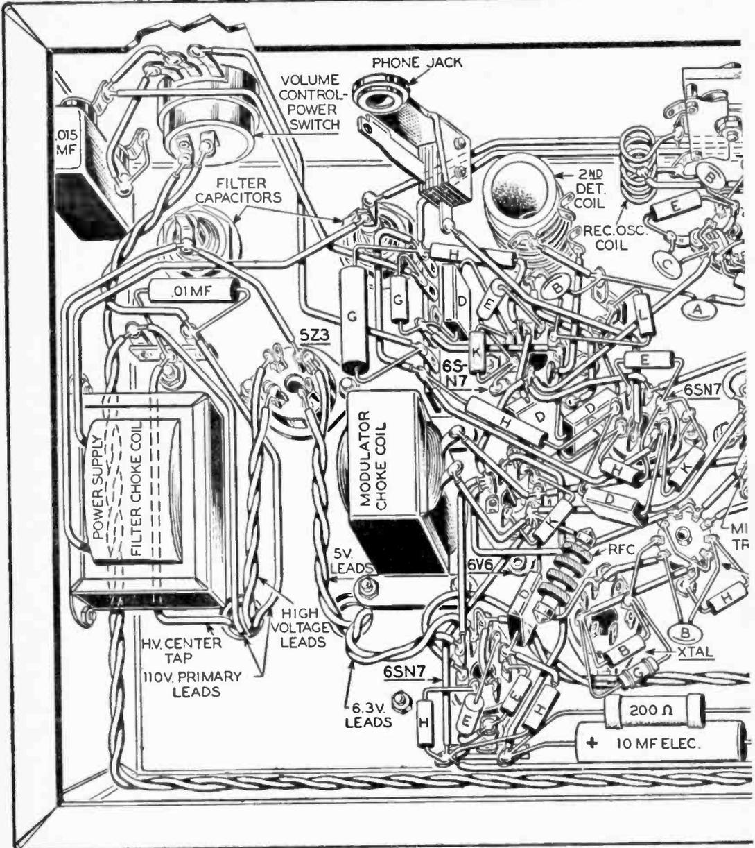
tion of the 12AT7 is soldered to the coil one turn from the ground end. When the R.F. amplifier, mixer and oscillator circuits are completed, apply power and throw the send-receive switch to the receive position. The tuning range for the oscillator, as indicated by a grid-dip meter, should be from within about 115 to about 132 megacycles. If the oscillator is not oscillating, look for shorts between tube pins or try a dif-
