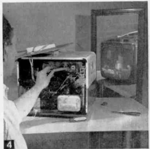
The service tech uses an insulated plastic wand to tap tubes. He watches the screen in a mirror, or reflected from a window. Erratic picture or sound pinpoints the faulty tube.
