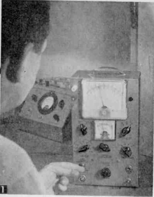
Determining leakage current at various collector voltages. Transistor under test is in socket at right of large meter.
