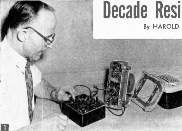
Decade resistance box in use in radio servicing job. Various values of resistance are being applied across terminals where a defective resistor was formerly soldered, and which is now unidentifiable due to extreme heating.
