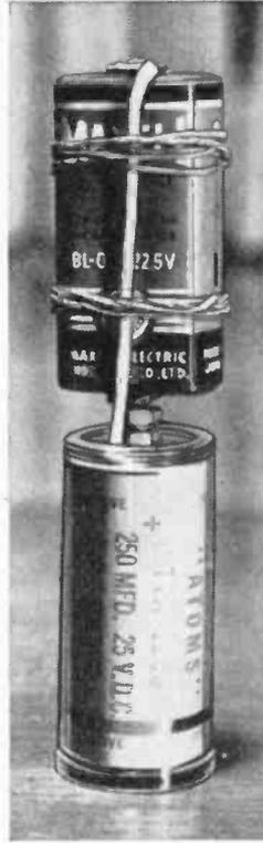
FIG. 6: Place the negative pole of a 22.5-volt battery in the recess. Then run the insulated lead wire from the positive end of the capacitor up along the side of the battery. Leave the tip bare and wedge it tightly under the positive battery pole strip.
