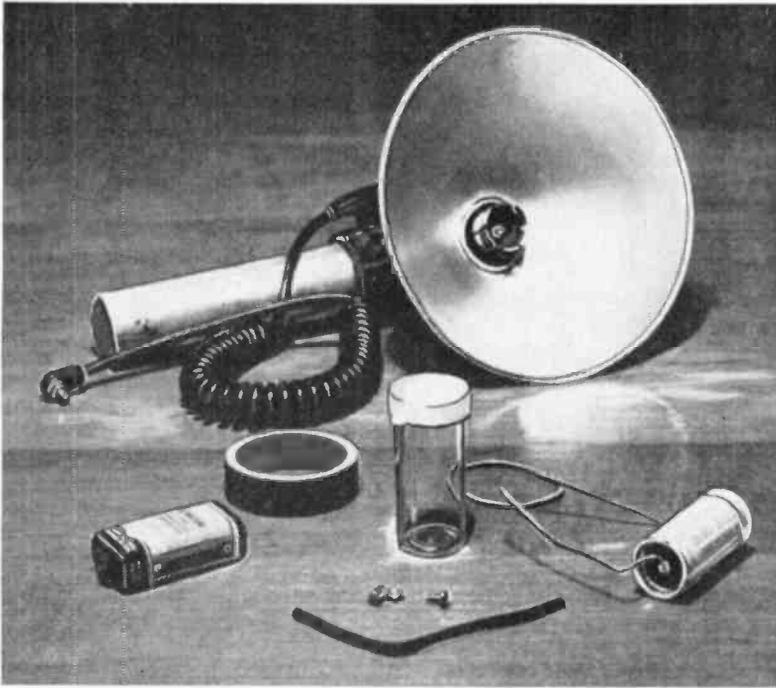
FIG. 1: Items in foreground are all that are needed to convert the flashgun into a more dependable, economical B-C unit; 22.5-volt "B" battery, small piece of friction tape, plastic pill bottle, rubber bands, 250 mfd 25-volt capacitor, small bolt, two nuts, and sleeving.
