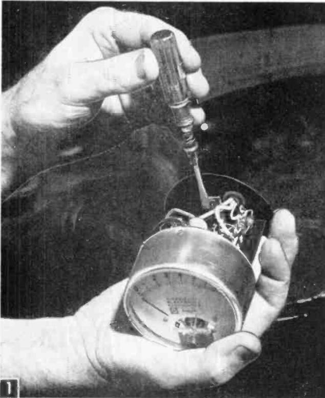
After the kit is assembled, you connect one of the leads to an a-c power line to calibrate the needle setting for your car. A simple screwdriver adjustment completes the job.
