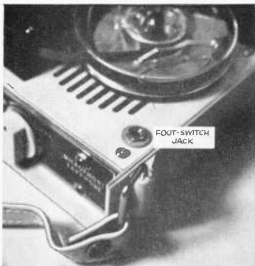
FIG. 1: Locate the jack for the foot switch on the front panel. Place it so the foot switch cord will not interfere with normal tape recorder operation.
