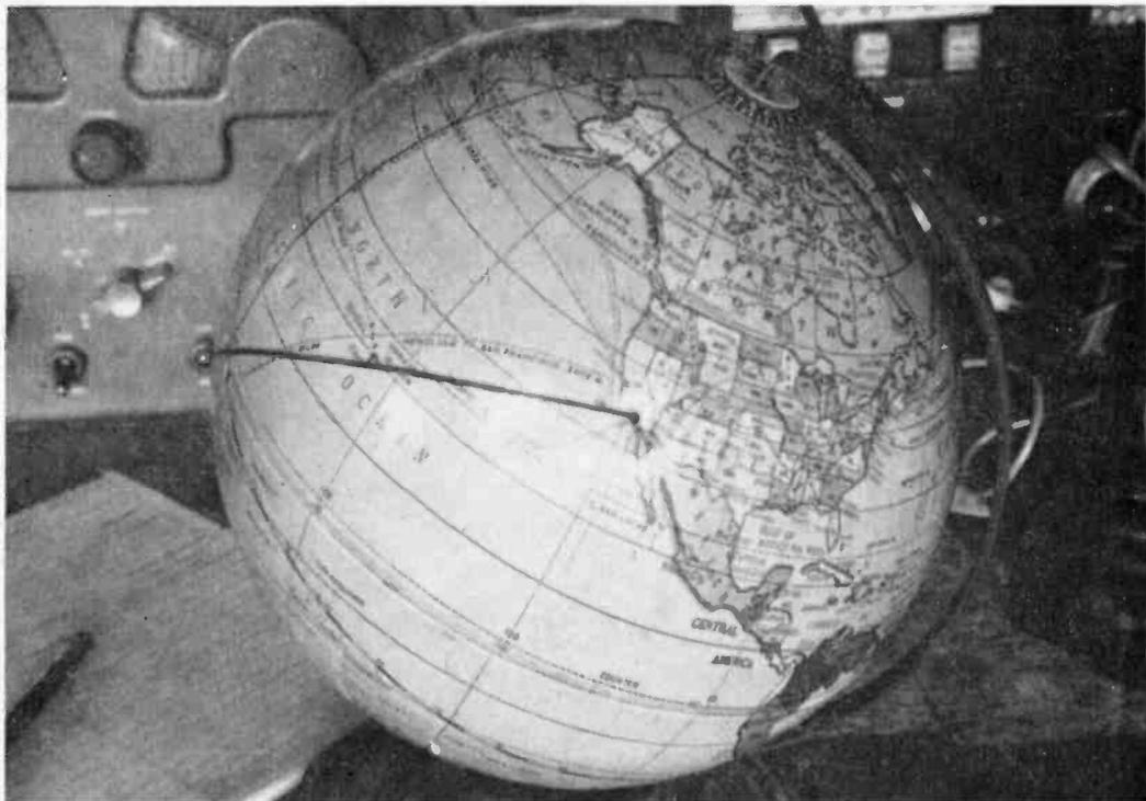
Fig. 1: The directional wire is mounted at Los Angeles and swings over the globe. Here we take a bearing on Hawaii and we can read the approximate distance in miles.
