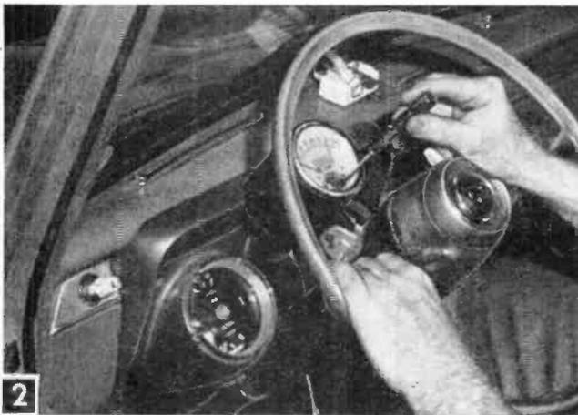
Space between the dash and steering column on this import car was limited. But a good fit was made by mounting the housing casting backwards. Kit brackets also make over or under-dash mounting possible.
