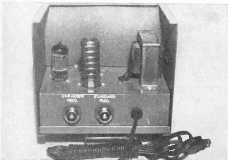
**FIG. 4:** Microphone connectors are shown for input and output terminals. Use any coaxial connector.
