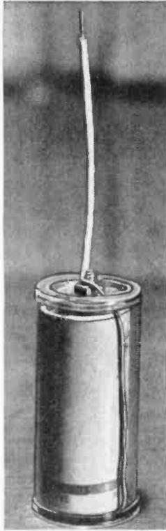
FIG. 5: Now crimp the negative wire to the stove bolt and tighten the nuts to insure a good connection, but be very careful not to crack the plastic. The stove bolt should be short enough so that the second nut can be threaded only partially. This recess holds the negative pole of the battery.
