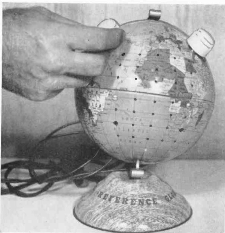
Tune in a station with the knob at the left. The other knob is your volume control and on-off switch. Holes allow sounds from speaker to come out.
