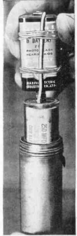
FIG. 7: Secure the lead wire against the battery with two rubber bands. The wire is stiff enough to hold the battery firmly in place. Slip the completed unit into the battery case and it's now ready to be fired.
