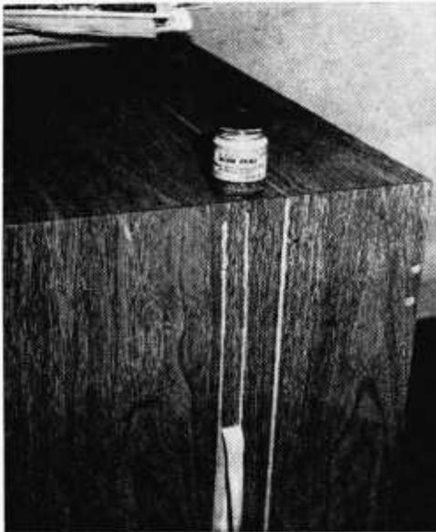
is drying (above) peel the tape off leaving two silvered lines that can serve as conductive leads. Wood finishers used to cover and hide deep scratches (right) hide the silver leads and restore the wood finish. A little practice at home is a good idea.
