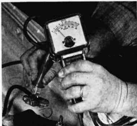
1: COMBINATION volt and ammeter is used to record battery voltage. Volt meter is connected in parallel with circuit being tested. Ammeter is attached in series to show draw.
