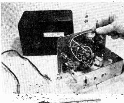
Tune-up tool, supplied with kit, is used for aligning two coils in the completed kit. CB rig provides signal for tune-up.
