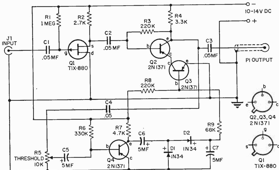
The unusual symbol for Q1 indicates the part is a field effect transistor. Its case resembles Q1's and Q2's. Part placement is not critical, however, try to duplicate the original design.
