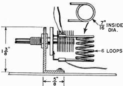
Coil L1 and capacitor C1 comprise the only tuned circuit in the TD-FM radio. Utmost care in assembly is necessary in order to insure a high-Q circuit on the frequency band the receiver is to operate. Bracket is made from an aluminum bracket strip 5/8" wide.
