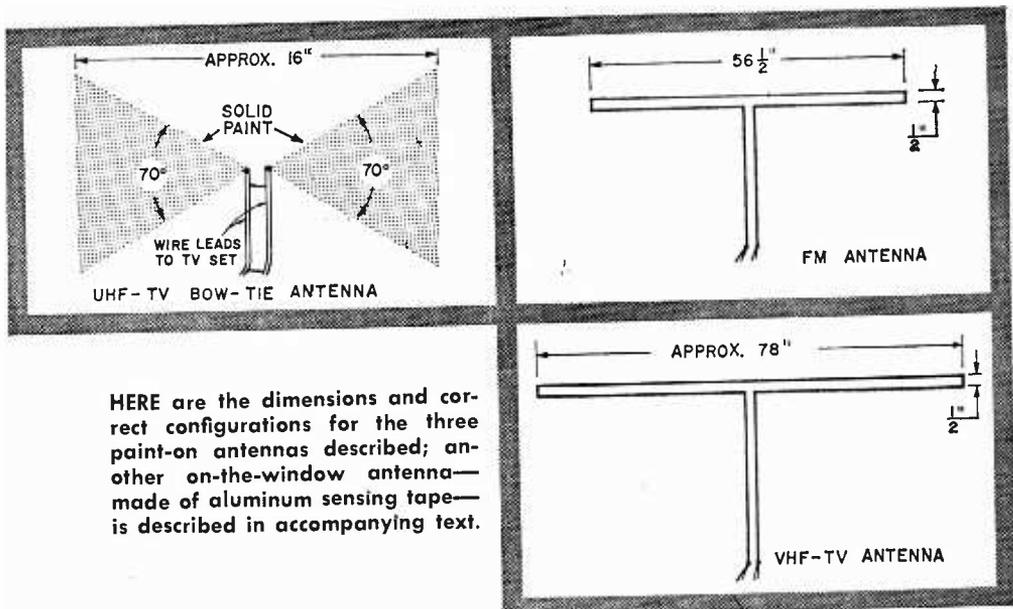
HERE are the dimensions and correct configurations for the three paint-on antennas described; another on-the-window antenna—made of aluminum sensing tape—is described in accompanying text.
