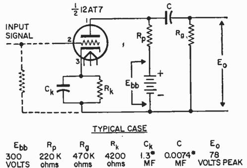
Fig. 4. The schematic diagram above is for a typical resistance-coupled amplifier circuit using one triode section of a twin-triode 12AT7 vacuum tube. One set of typical values for circuit constants are given below the diagram. Capacitors should be valued at next highest rating available.
