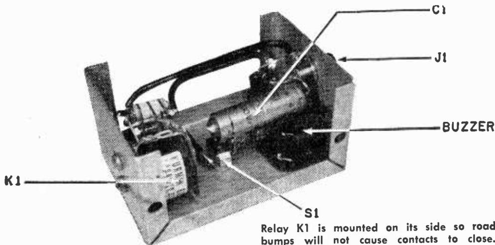
Relay K1 is mounted on its side so road bumps will not cause contacts to close.
