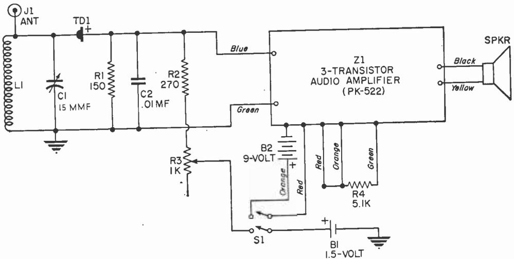
The placement of parts in the RF section is critical, but neatness in construction will lick more than half the problem. Keep leads and parts away from coil L1 and capacitor C1.
