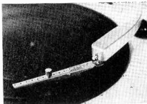
Stylus pressure gauge helps make correct tone arm tracking pressure adjustment. This adjustment prevents rapid record and stylus wear due to excessive pressure.
