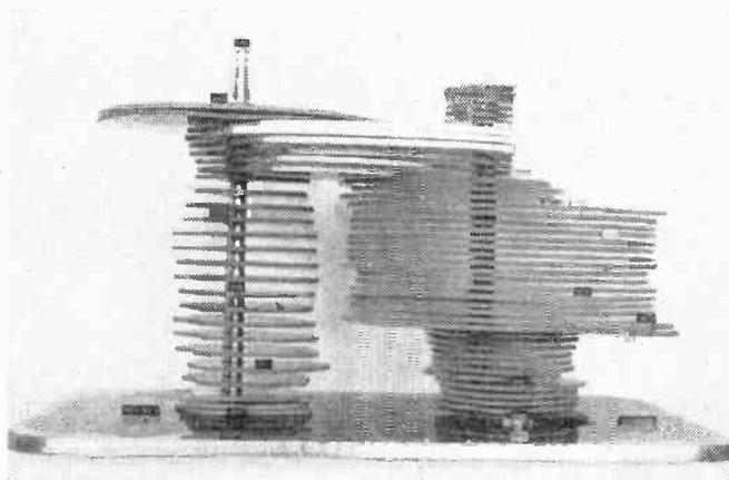
Plastic disks cut to scale (1 inch equals 20 feet) are stacked one on top of the other to give well makers an exact model of the underground cavern washed from the salt bed. Irregular shape results from different solubility of varying strata of the salt beds. Model at left shows a very deep well. Model above shows how two caverns were accidentally connected together by a washout that only the sonar caliper can discover.
