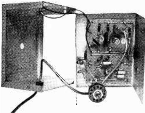
The CB-Lim prior to final assembly. There is enough room inside to mount dry cells.
