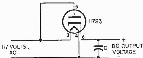
Fig. 3. Half-wave rectifier circuit using a capacitor input filter. The 117Z3 vacuum tube filament pins can be connected directly across the power line eliminating the need for any filament transformer.
