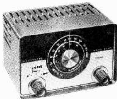
unit from line voltage variations. Illuminated plexiglass dial is calibrated from 50-54 mc. (6 meters) and 114-148 mc. (2 meters). Output voltage is 10-20 volts rms. Priced at \$29.95, the HE-89 operates on 115-volt 50/60 cps power. (Lafayette Radio Electronics Corporation, 111 Jericho Turnpike, Syosset, L. I., New York)
