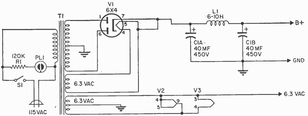
The schematic diagram for the oscillator and audio amplifier stages appears at the bottom of page 50. Unit is powered by full-wave rectifier and filament supply diagrammed above.
