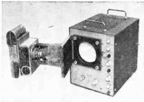
Quick-print Polaroid camera records oscilloscope pattern at each elevation measured.
