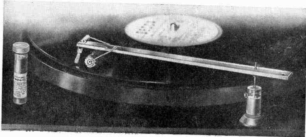
sound gets shrill and harsh. Gone is the tonal gloss, the radiance of sound which recording engineers had so carefully molded into the grooves. Later playings pile up more sound-shattering debris—and it acts like a grinding compound. The process accelerates, feeding on itself, and your prize records turn to scrap long before their time.
