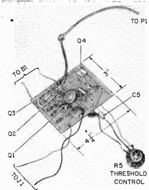
Almost all of the parts are mounted on a 3-by-4 $\frac{1}{4}$ -inch phenolic circuit board. Use stranded wire for leads leaving the board.
