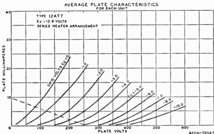
Fig. 2. The illustration on this page is taken from the RCA Receiving Tube Manual. The 12AT7 is a popular high-mu twin triode audio tube.
