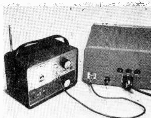
Here, the Ten-2 CB Checker is connected to the antenna terminal of the CB rig under test. One tester can rate your CB gear.
