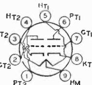
miniature nine-contact socket and may be mounted in any position. Each triode unit is independent of the other except for the common heater. For typical operation as a resistance-coupled amplifier, refer to Chart 10, RESISTANCE-COUPLED AMPLIFIER SECTION.
