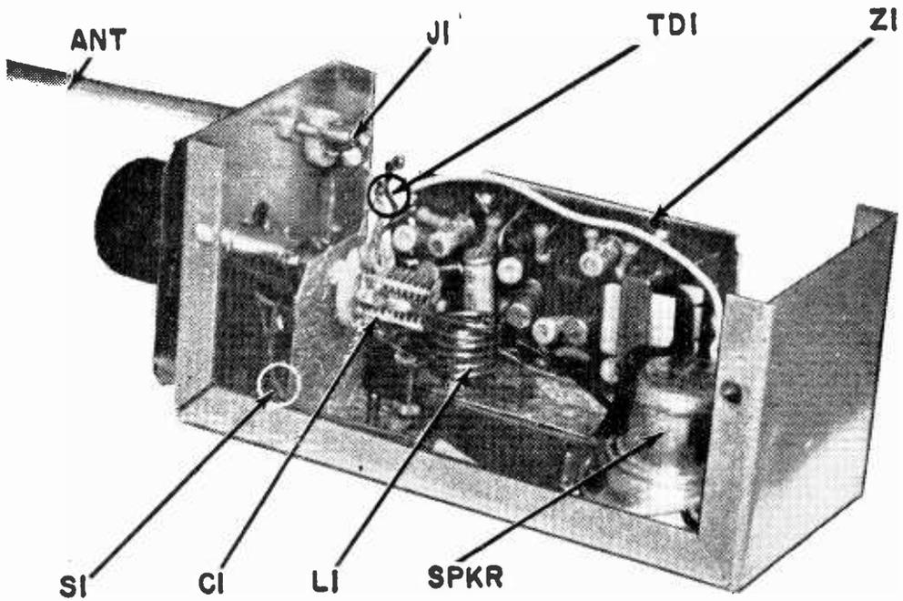
It's a tight fit inside the aluminum 2 1/4" x 2 1/4" x 5" chassis box. It would be best to copy the author's original layout of parts to avoid construction problems.
