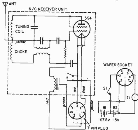
The receiver heart is the R/C receiver unit that is tuned through a small hole in its plastic case. Wafer plug and socket connect receiver to batteries. The socket also serves as a terminal point for connecting switch S1 and lamp.
