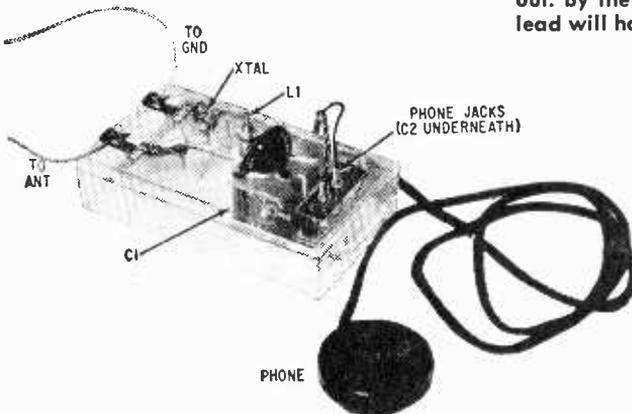
The home-grown radio at the left can be put together as easy as A, B, and C for crystal. See schematic diagram.
