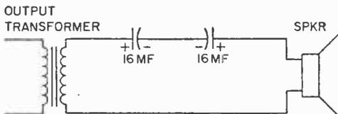
**A.** Connect two 16 ufd electrolytic capacitors back-to-back, as shown in the diagram, in series with the voice coil lead. The reactance of the capacitors is high at low frequencies and will cut bass response. By connecting the capacitors as shown, since they are polarity sensitive, they can be used in AC circuits such as audio.
