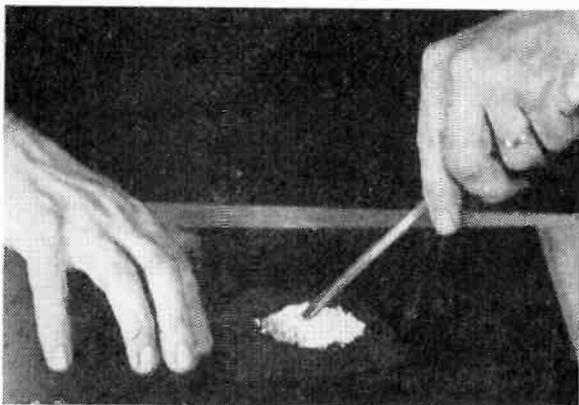
**Step 2.** Measure out six parts by weight of lead powder to one part of sulphur. Proportions aren't too critical. It's best to be liberal with the sulphur because, unfortunately, a great deal of it goes up in smoke. Be sure to mix the lead and sulphur together thoroughly.
