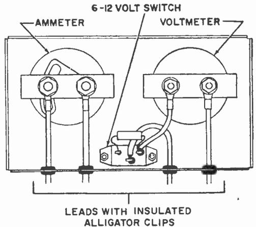
Outline drawing shows location of parts in tester and ease in which it can be assembled.
