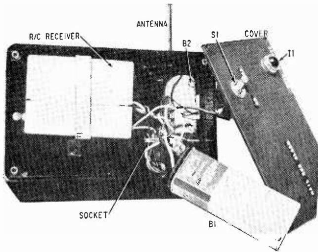
The receiver unit, a bakelite meter case, houses the commercial R/C receiver, its power supply, the wiring to the telescoping antenna, indicator light and on-off switch. This packaging makes unit versatile for placing in the house or yard.
