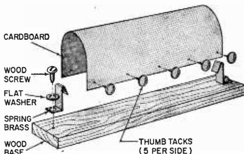
Assemble the battery holder by first determining the distance required between the spring brass end terminals. Do this by laying out the number of dry cells the holder will mount and scribe lines at ends.
