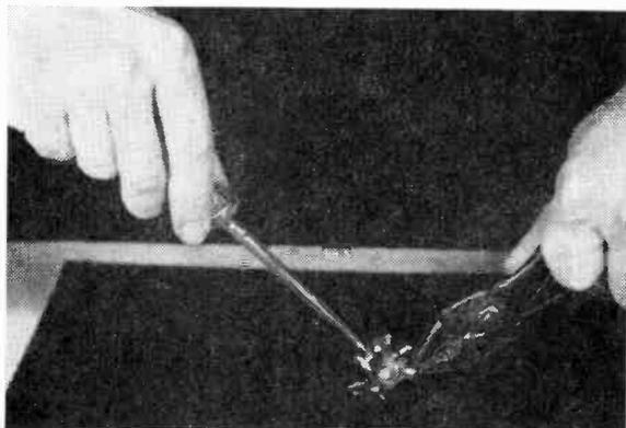
**Step 5.** Cut the tube open with a hacksaw and remove the lump of metal. If nugget breaks readily and the broken surface presents a sparkling appearance, you have lead sulfide. If lump is not brittle but malleable, the sulphur burned up before crystallization took place. Start over applying heat more gently.
