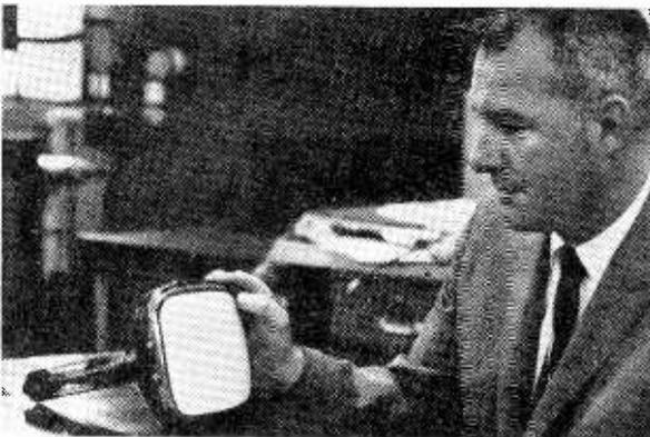
Mockup of basic Chromatron structure (upper left) shows glass phosphor screen, left, wire grid, center, then bellshape section leading to neck of tube. Layout of small Chromatron (above) that will be seen late next year. Note dark frame held by hand. It permits one-piece assembly of fine grid-wire suspension; an important breakthrough for mass-producing the Chromatron. At lower left, Engineer John Petro looks at 8" and 23" Chromatron.
