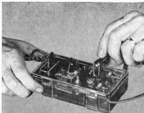
It will take a steady hand to bring the "catwhisker" in contact with shear face of crystal.
