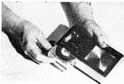
The tape cartridge snaps in and out with a gentle tap or pull when the recorder is set at off. Plastic case and window in recorder lets you see how much tape has been used.
