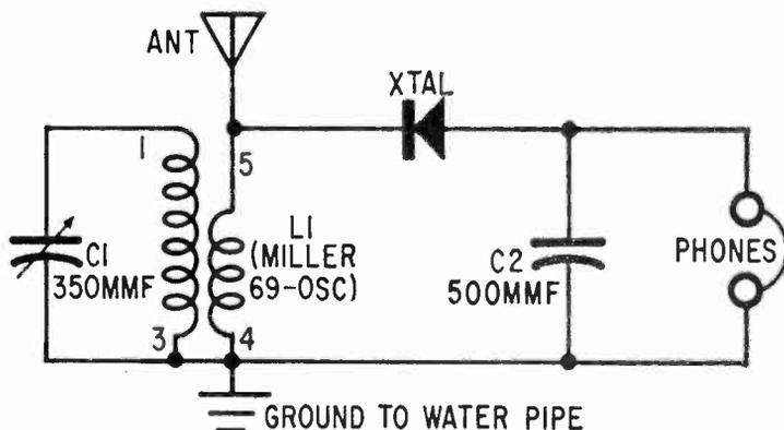
Using this schematic diagram, you can begin construction of a crystal receiver with a detecting diode you've homemade. If you wind your own coil to boot, you'll ignore coil detail.
