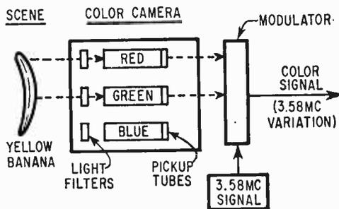
Fig. 2. TV camera breaks scene into primary colors—converts them to electrical signals.
