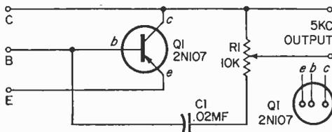
Feature of oscillator adapter is 10K potentiometer, R1, to attenuate the signal when working on a receiver front end. Transistor base diagram identifies leads.
