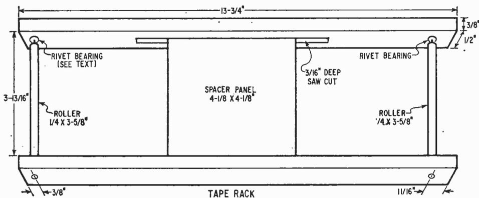
Detail drawing for making the four assemblies of the tape loop pack.
