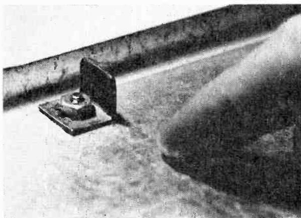
The angle bracket on the mailbox lid holds the mercury switch off until the lid is pulled open.
