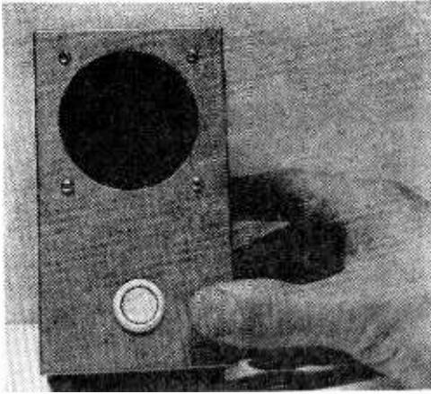
The rear door button and rear door speaker can be mounted in a single aluminum chassis box as the author did. However, both parts can be mounted on a metal plate and flush mounted in the door panel. If you wish, add a jewel lamp to illuminate the panel at night.
