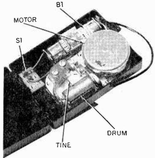
Small size of the music box movement makes Boinger feasible for use on telephone handset. Note the removal of all tines but one.
