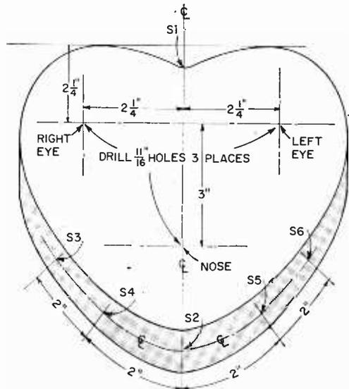
You'll find this heart-shaped chassis in the kitchen—it's a cake pan! It quickly changes to a "funny face" by placing lights, switches, batteries as shown in these chassis layouts.
