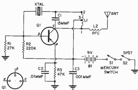
The transmitter radiates on R/C and CB channel 23—27.255 MC. The crystal controlled oscillator utilizes PNP transistor Q1. Switch S2, in series with mercury switch S1, is necessary to cut off transmitter at will without disarming S1.
