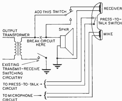
Delcon Corp., 943 Industrial Avenue, Palo Alto, Calif. manufactures a scrambler that fits over a handset. It can be used with a regular telephone or with a CB set that has a handset instead of a regular mike. A handset can be connected to a CB set as shown in the diagram. The handset must be equipped with a press-to-talk button and the microphone element must be of a type that matches the CB set. Handsets are available from Roanwell Corp., 180 Varick Street,
