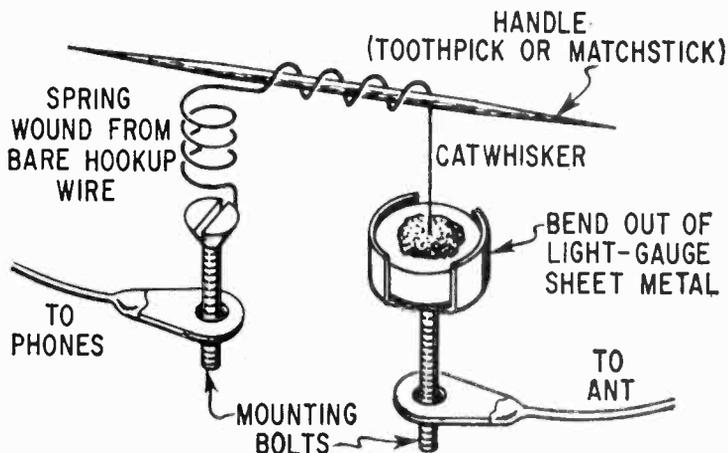
This being one method of engineering the catwhisker to make a contact with the crystal.
