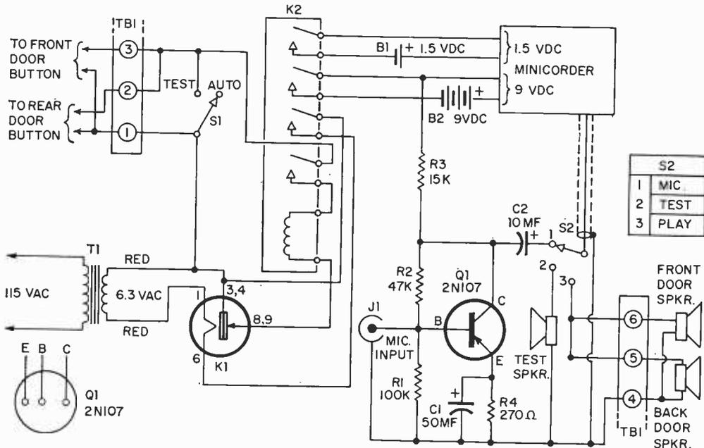
Schematic diagram for the Electronic Greeter. Wire Q1's circuit close to Minicorder
