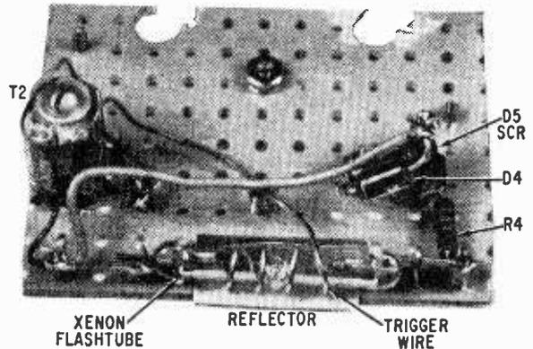
The stroboscope is wired into a flat, long, aluminum chassis box permitting uncrowding of parts. Perforated circuit board (above) mounts on meter screw posts (see below). Except for resistor R9 (hidden under capacitor C2) all parts are shown in photos.
