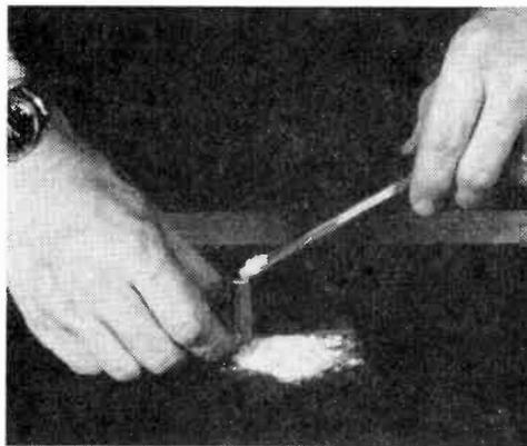
**Step 3.** Pour the mixture into a piece of copper tubing about 1½ to 2 inches long and tamp it down. Fill the tube about half full. Fill the rest of the tube with sand to reduce the amount of oxygen available to the sulphur in order to decrease its rapid burning.
