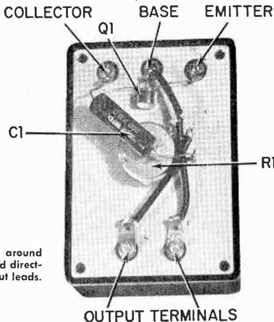
Rear view of front panel turned around in case shows transistor connected directly to bolts, and spaghetti on output leads.
