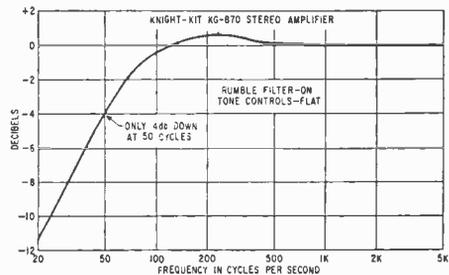
Curves at left and above show effect of scratch filter and rumble filter, respectively, with tone controls flat.
