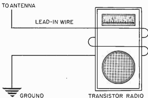
**A.** Wrap the antenna lead-in around the set. Two turns will do. And, ground the far end of the lead-in as shown in the diagram. The ground is important. The wire wrapped around the set acts as an antenna coil which is inductively coupled to the loopstick antenna inside the radio.
