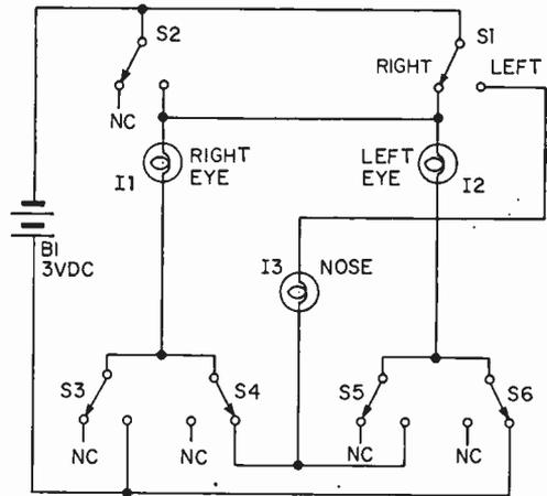
Lighting the face is easy when you can consult the schematic diagram to determine the correct combination of switches to close.
