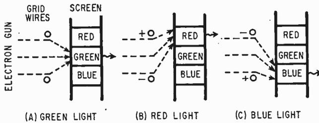
Fig. 5. Applying voltages to pairs of grid wires focuses the electron beam on one of the three phosphor screen stripes.
