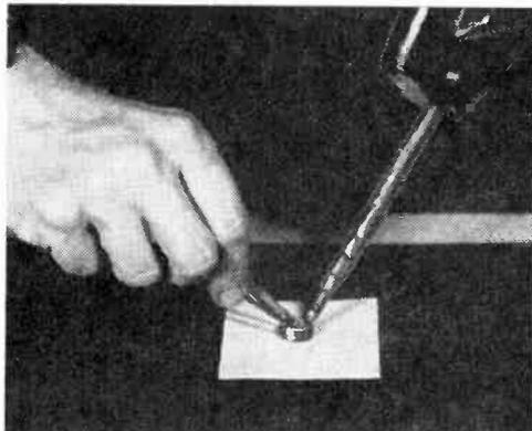
**Step 6.** Line a small ring of copper with paper to keep solder from sticking. Melt the ring full of solder and embed a fragment of crystal. When the slug cools, remove the ring and save for reuse. Clean the solder slug so it will make good contact with its holder. Now the mounted crystal is ready to be used.
