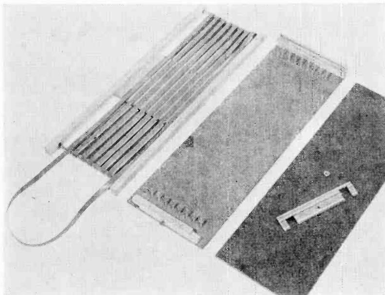
**FAR LEFT.** Paint dark bands on the spacer panel of the rack to facilitate loading of the tape (see text); at top of photo is front end of base panel, showing notched block and one set of tape spacer pins set in place.
