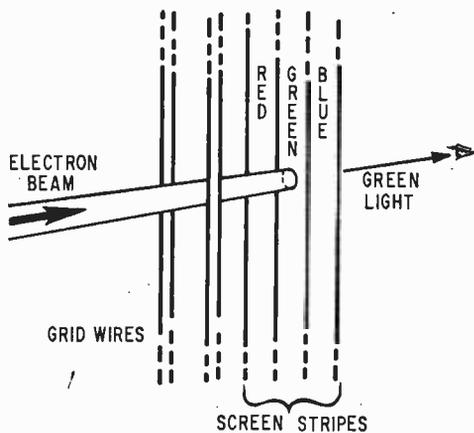
Fig. 4. Electron beam passes between grid wires undeflected—shown striking green phosphor stripe between red and blue ones.
