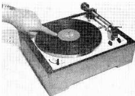
Finger points to the strobe disc which is an integral part of the turntable mat. Second knob from right is variable speed control.
