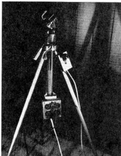
Central switch (left) for all your photoflood lights mounts on tripod leg (above).
