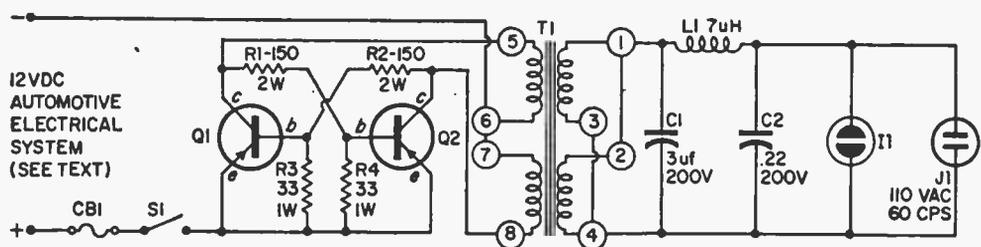
Schematic diagram of inverter shows two-transistor multivibrator heart and step-up transformer T1. Filter L1-C1-C2 de-spikes the transformer output and forms a trapezoidal wave approximating a sinewave shape.
