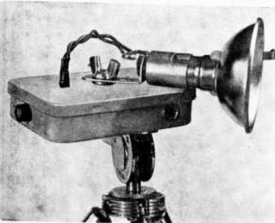
The completed slave photoflash can be mounted on a tripod as shown here. Enough twisted lead is left so the flash can be swiveled in any direction by loosening the wingnut.
