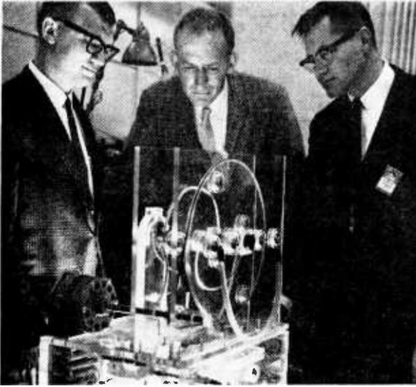
Boeing Company antenna experts T. L. Johnson, Robert Tighe, and Arthur Guy study the electrical impulse generator they designed for sub-surface antenna experiments in the Antarctic. One of the Boeing team, shown below, has his turn at the morning chore—digging antenna cable and supplies out of snowbanks constantly formed by drifting snow.
