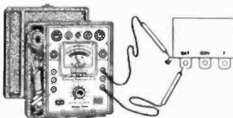
Proper test of regulators requires measurement of voltage, resistance and current drain. The Model 161 is one of the very few testers ever produced which provides all those services.
