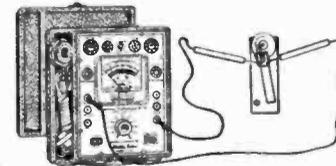
The thermostat is a very frequent cause of trouble in furnace control systems. The 24 voltage secondary usual with such units can be accurately measured with Model 161.
