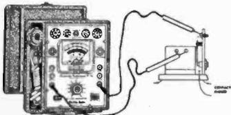
Model 161 Utility Tester tests all circuit breakers including the magnetic type.
