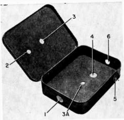
Refer to the text for dimensions of the holes drilled in the hinged metal box shown above. After drilling, deburr the holes and, after preliminary wiring, mount and finish wiring the components as shown at the right.
