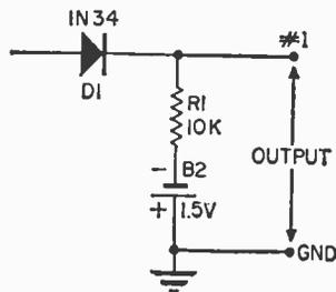
Fig. 5. Equivalent circuit for off signal.
