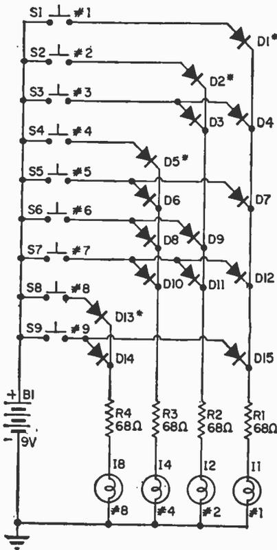
Fig. 1. Schematic diagram for an easy-to-build four digit, decimal-to-binary demonstrator.
