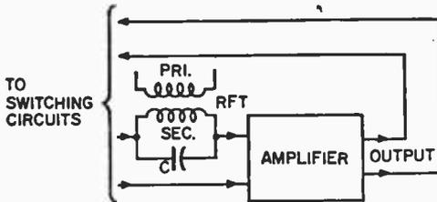
in the diagram. Use the secondary of a shielded RF transformer as the coil and an adjustable mica trimmer capacitor as the filter. Tune it carefully to 1520 kc, the point at which the radio signal is at a minimum or eliminated.
