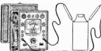
Model 161 tests both single and two post ignition coils.
