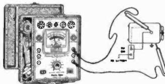
Testing heating systems. The causes of trouble vary but Model 161 will check out all. Detailed instructions are included in the Model 161 manual.
