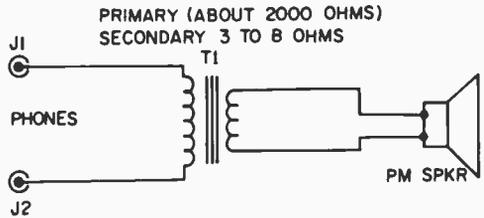
Fig. 3. How to add loudspeaker operation.
