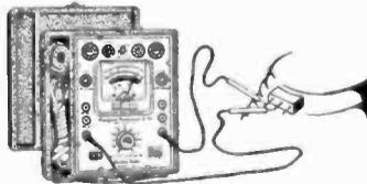
Two-heat broiler testing is a cinch with the Model 161. The "low" contacts should read 40 ohms and the "high" contacts should read 20 ohms.
