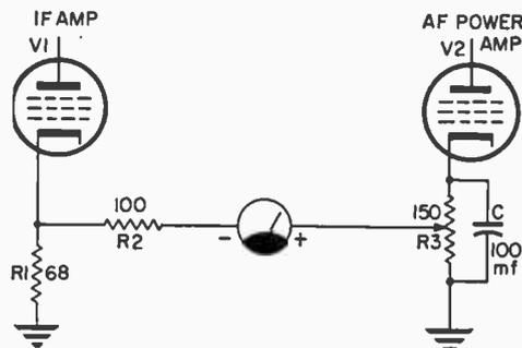
When a signal is received, the voltage drop across R1 falls off because V1 cathode current is decreased by the AVC voltage which is now higher. Hence, the voltage at the positive meter terminal is higher than at the negative terminal. The meter reading varies with the voltage drop across R1. The voltage drop across R3 remains steady. The value of R2 can be varied from the indicated value to calibrate the meter.
