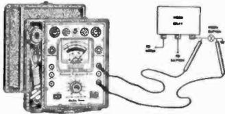
Ever experience anything more embarrassing and frustrating than trouble with the auto horn? Model 161 will check out the complete horn system including relays, buttons, etc.
