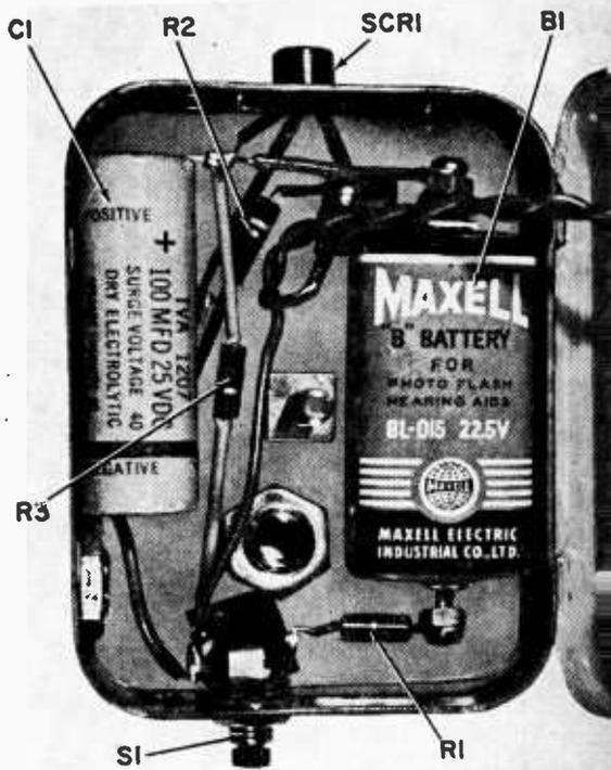
Screw the tripod socket adapters into holes 4 and 5, fastening on the inside of the case with  $\frac{3}{8}$ -in. flat hex nuts. Fit the stove bolt up through hole 3 and secure it with a corresponding nut. Install switch S1 in hole 6.
