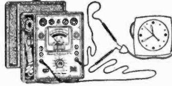
Electric clocks consume so very little current it is impractical to test them with line meters. The Model 161 will check such clocks accurately by simple connection to the electric cord.
