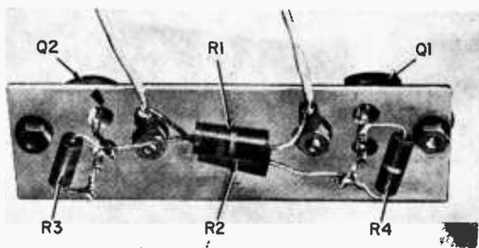
Transistors Q1 and Q2 are mounted on aluminum angle stock which acts as a heat sink. After transistors are mounted by following details in text, wire resistors R1 through R4 as shown above. Chassis punch, left is excellent for cutting a circular hole for the AC outlet, J1.
