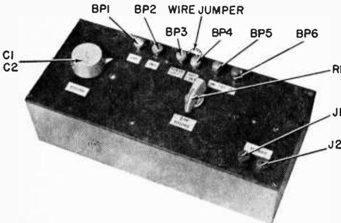
Front-panel view shows tuning and volume knobs. Binding posts along top edge are for connecting battery, antenna and jumper. Use a red post for BP6, black one for BP5. Other posts are white. Output is obtained at jacks J1 and J2.
