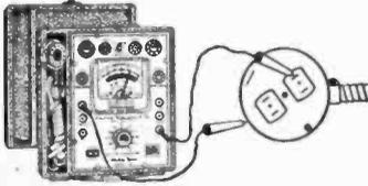
How to determine which side of power circuit is grounded! Simply connect one Model 161 lead to BX and the other lead to one of the two slots in the outlet. The side which is grounded will cause the meter to read.
