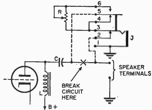
chassis or cabinet, break the circuit at X in the diagram and add R, a 10,000 ohm potentiometer, all connected as shown. When the phone plug is inserted in the jack, its 4-5 and 2-3 contacts open, disconnecting the speaker. Its 5-6 contacts connect the audio output to the ungrounded headphone lead (tip of phone plug) through R which is connected as a series rheostat and serves as a headphone volume control.
