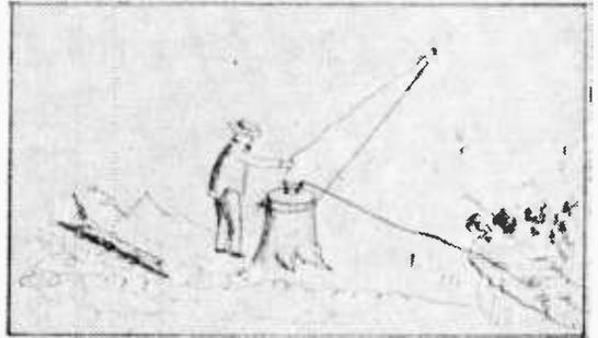
Diagrams from Loomis' notes record for posterity the equipment setup used in 1866. Above, receiving station consists of detector on log, antenna suspended by kite and ground wire in lake; below, identical setup, however, antenna is connected to detector to trigger impulse.
