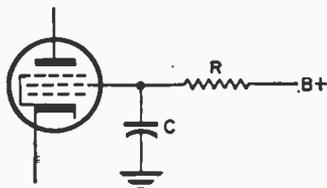
placements. The resistor should be color-coded to indicate its resistance. If the color code has been burned off, try various values from 50,000 ohms to 500,000 ohms until the sound is cleanest. Use an 0.1 mf. tubular rated at 200 volts or higher as the replacement bypass capacitor. Its value isn't critical.
