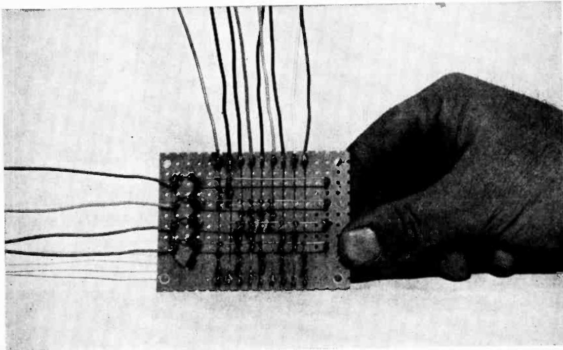
A simple rectangular array of semiconductor diodes plus some switches and lamps can be assembled by you to convert decimal numbers to binary digits
