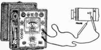
To test generators use the voltage range of Model 161 and when necessary the resistance range. Model 161 will test generators with external field coil terminals.
