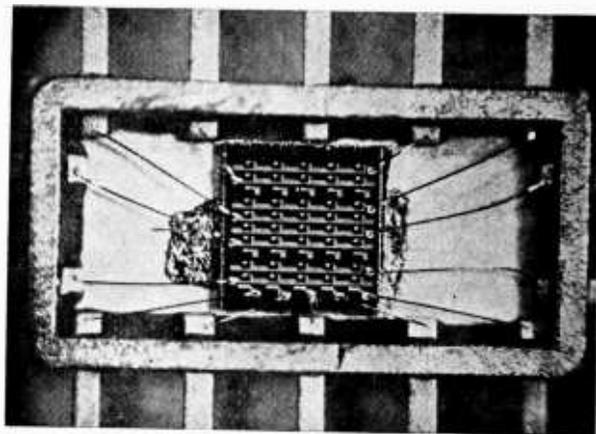
Microminiature matrix circuit designed for computer application—enlarged ten times.
