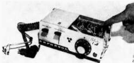
Amphenol's selective call unit can be placed directly on the transceiver (top, left) or mounted to an auto dash. Connection to CB set is simple. Since speaker muting is provided in Amphenol CB rigs, only three connections are made to the rig (top, right). The receiving code is easily changed (left) by rearranging four plug-in leads. No desoldering is necessary to pick one of 24 codes. Dial selects any transmitting code.
