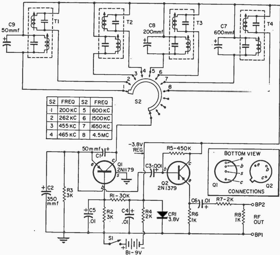
Frequency determining tank circuits are selected by switch S2 and passed to collector of Q1.
