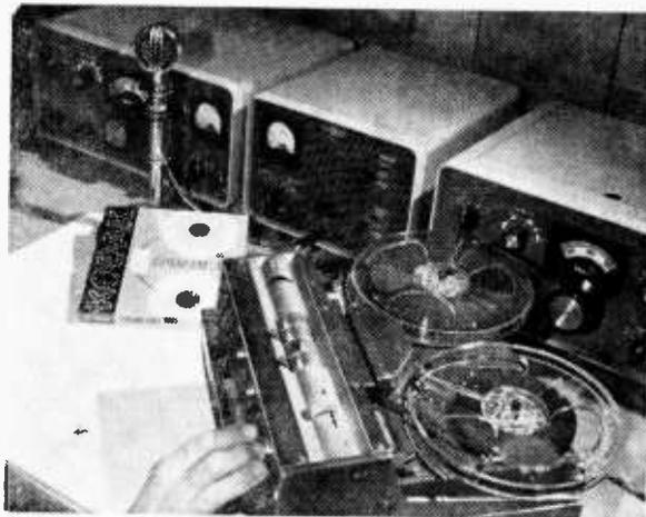
What's in the shack: Collins 325-1 transmitter, Collins 312B-4 speaker control, Collins 755-1 receiver, Wollensak T-1580 tape recorder loaded with Kodak high-output audio tape.
