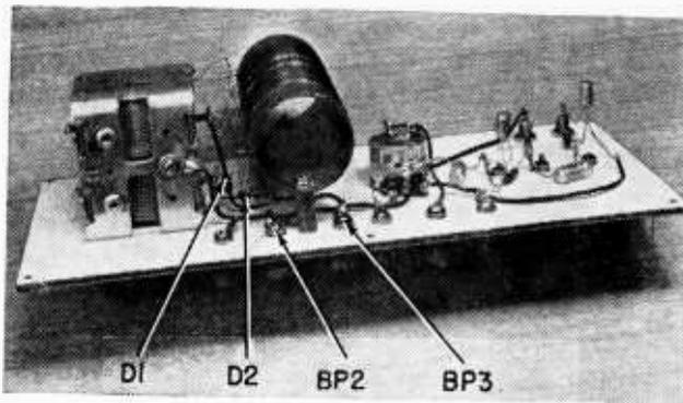
Coil is mounted above surface of panel with spacers or piece of wood dowel. Note the tuning capacitor at left; a solder lug is screwed in one threaded hole on frame. Lug receives wire from control R1 and BP6.
