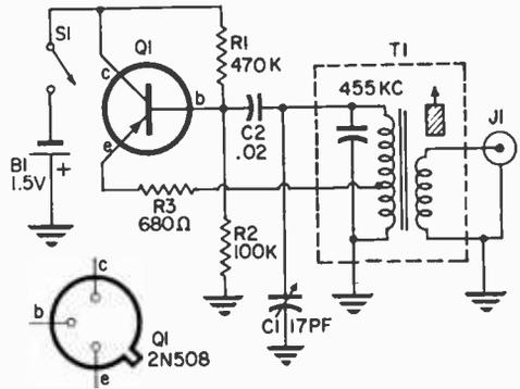
Be sure to follow Q1 connections, as shown in schematic above. Q1 mounts in transistor socket seen in left photo. Wire complete board before inserting in metal case.
