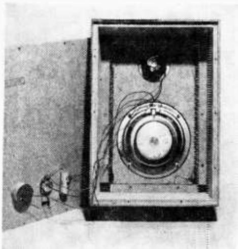
The completed speaker kit (left) is ready for its fiberglass stuffing. Now is the time to check your wiring. Below, a coat or two of clear lacquer will protect the oil stain finish.
