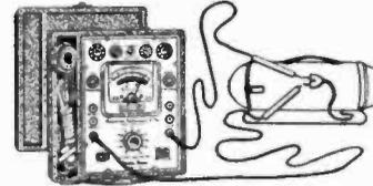
A vacuum cleaner can be tested best by resistance measurement first, and then, if necessary current consumption and applied voltage. All three measurements including leakage when necessary are supplied by Model 161.
