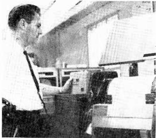
Pistol-packin' cop, trained by IBM, now operates console which stores information on reels of magnetic tape. This is just one section of a computer installation worth \$300,000. Filing cabinets (below right) contain over 150 data processing programs. Since computers can't really think for themselves, programs provide instructions for handling the data.
