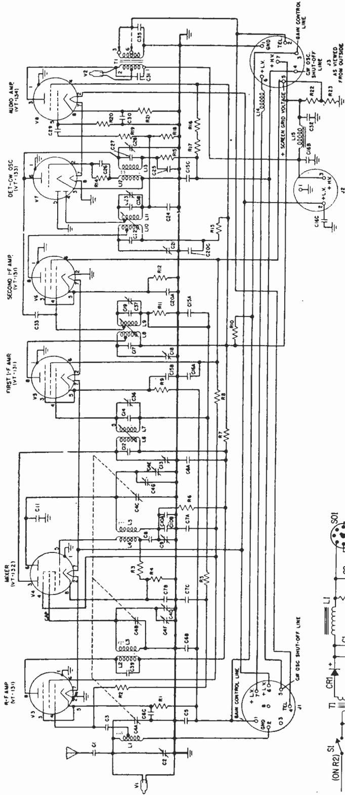
Fig. 1. Schematic diagram of the lowest frequency receiver of the "Command" type. The IF frequency of 85 kilocycles is amplified in two IF stages.
