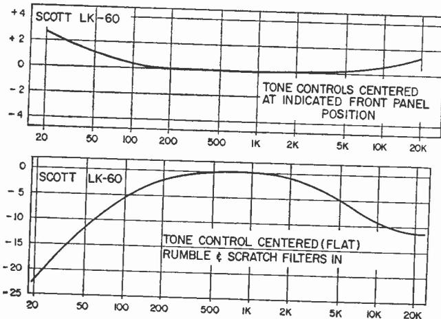
Fig. 1. Frequency response curve plotted with tone controls centered shows response boosted less than 3 db at 20 cycles. Adjustment of controls gives flat response within 1 db.
