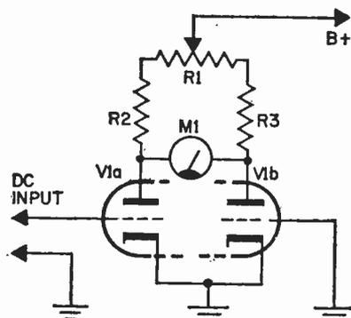
Fig. 2. Meter M1 reads zero in bridge circuit with zero input—DC input upsets balance.
