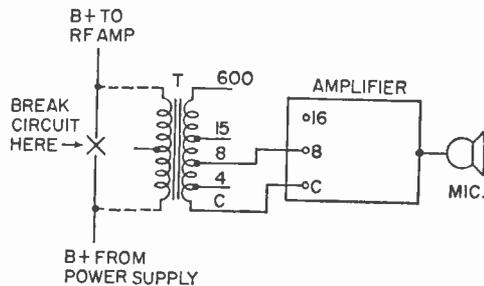
can be varied by trying various amplifier output and transformer connections such as 8-ohm or 16-ohm amplifier output to 4, 8 or 15-ohm transformer lead. Set the amplifier tone controls to reduce high frequency response so you won't cause excessively wide side bands to be produced.
