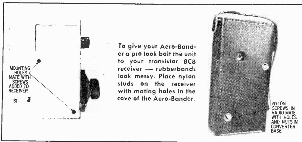
To give your Aero-Bander a pro look bolt the unit to your transistor BCB receiver — rubberbands look messy. Place nylon studs on the receiver with mating holes in the cove of the Aero-Bander.
