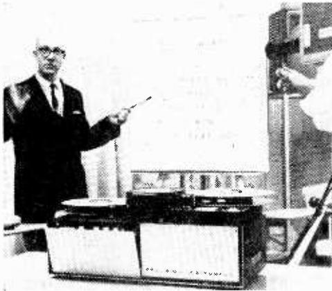
both pilot and landing control personnel. Developed by The Ampex Corporation in conjunction with the United States Navy, Pilot Landing Aid Television (PLAT) is a completely integrated system of electronic audio and video recording designed to monitor and simultaneously record aircraft landing operations from approach through final recovery under day and night conditions and to immediately play back the recording for post-flight analysis and evaluation.
