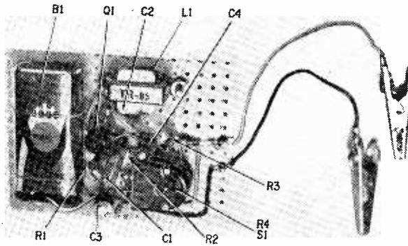
Finished project may be used without a cabinet. Two audio output leads are at right, ending with alligator clips.
