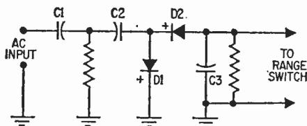
Fig. 3. AC input circuit is actually a simple voltage doubler that charges P-to-P, not rms.
