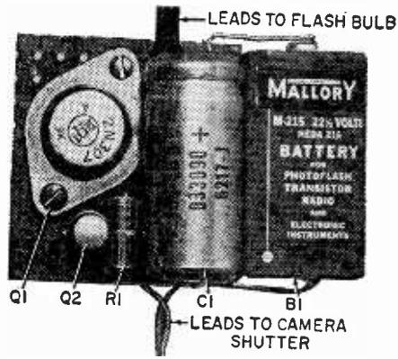
The handful of electronic parts that make up the Transiflash fit neatly on a 1 7/8 x 2-inch phenolic board as shown above. Dry cell battery (below) juts past board and is held in place by its leads. Entire unit can be potted with only the battery outside.
