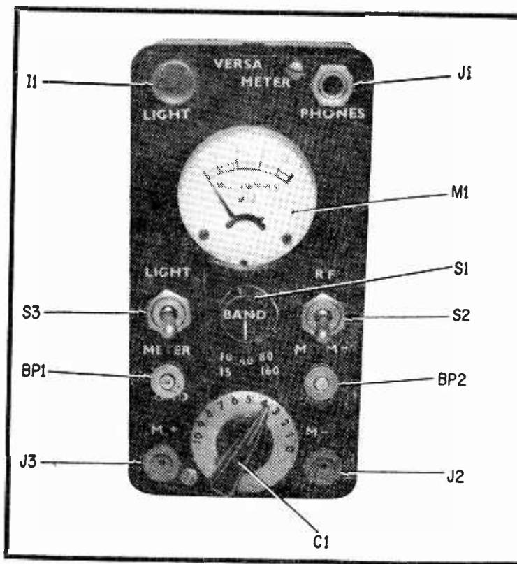
Front panel of Versameter, a multipurpose test instrument for the ham shack. Dials and switches are easily accessible to quickly select among the unit's various functions.
