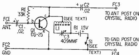
Simple? You bet it is! Only one tuned circuit is used to eliminate tracking error. Transistor Q1 is not critical. Almost any pnp unit rated at 2 mc., hfe 10 will do the job. Aside from units given in parts list, the following may be used for Q1: 2N247, 2N252, 2N274, 2N308-310, 2N315, 2N370-374, 2N384, 2N501, 2N504 and other pnp rf units.
