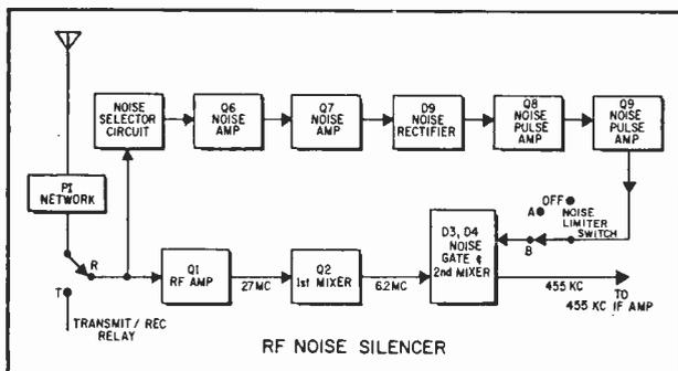
Block diagram shows signal flow in the RF silencer circuit. Noise selector circuit picks off noise on 25 mc.—same noise heard on CB band—then uses this noise to "punch holes" into the CB sound output when random noise pulses occur.
