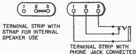
er and use an external speaker, or use both speakers. How can I install a headphone jack so the internal speaker will be disabled when I plug in the phones? The set is designed for use with a 3.2-ohm speaker.
