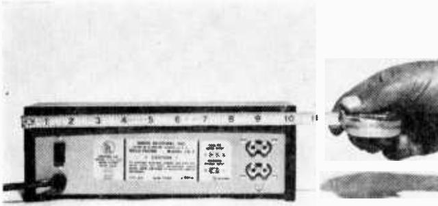
Width of amplifier is 10¼". At left are seen AC cord, and switched AC receptacle. At right are input sockets. Input impedance for phono is 47,000 ohms; for tuner or tape it is 250,000 ohms. AC power drain is 5 watts.
