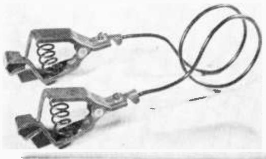
The "coil" shown above is a useful accessory for the ham or CB mobile operator. It forms a coupling link between a grid-dip meter and the whip antenna. To use it, disconnect the coax feed line from the base of the mobile antenna and attach this gadget. One clip goes to the base of the antenna and the other to a good ground on the car body. Move the grid-dip meter near this coil and operate the meter to find the antenna's resonant frequency.
