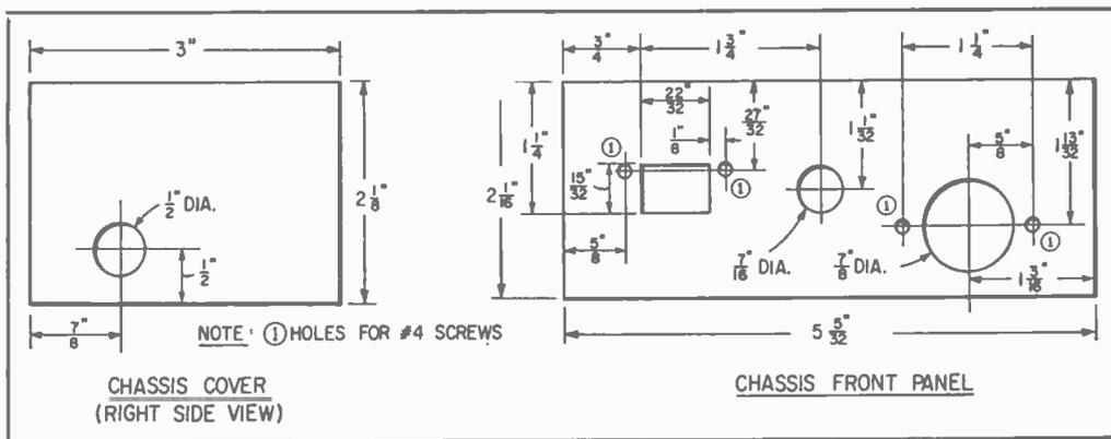
The drawings above provide exact locations for cutting the chassis to receive J1, S2, S1, and SO1. Side view of the chassis, at the right, shows contact strips of the lever switch. The wires going out of the picture connect to jack J1 mounted on chassis cover.
