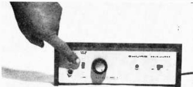
Switch on SA-1 front panel is used to select phono or high-level inputs such as tuner or tape. Knob to right is dual-type control for stereo balance and volume. Although fully transistorized, the SA-1 has self-contained power supply for operating from 117 VAC. Audio output power is 20 milliwatts; more than ample for listening on headphones.
