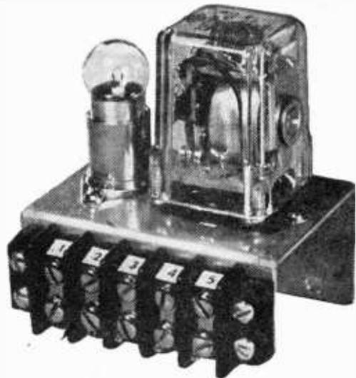
The cold weather car starter can be easily mounted in your engine compartment in the most convenient location. Then just make the five connections to terminal strip TS1.
