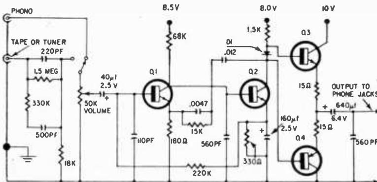
Schematic of SA-1 showing one of two identical stereo channels. Circuit is equalized for RIAA playback; output of unit is push-pull.
