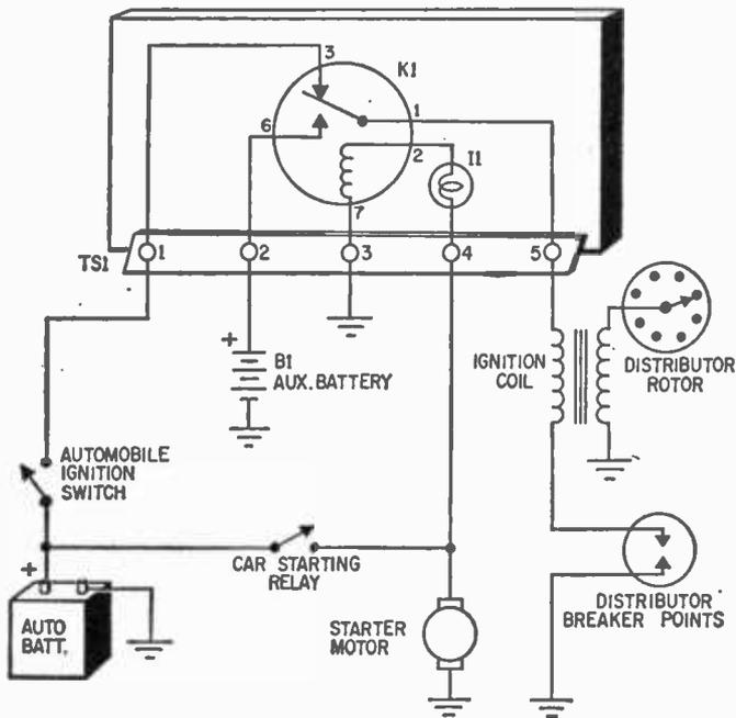
Combination schematic diagram and pictorial shows the car starting aid and its connections to your automobile starting and ignition systems. Current through the starter motor connects the auxiliary battery to the ignition coil through relay K1.
