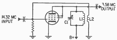
**B Frequency multiplier basic schematic.**
