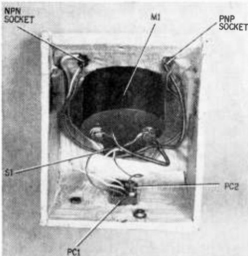
As far as the selection of photocells is concerned, you can use any type on hand, or you can order two from any of the electronic mail-order houses. The two used in the unit shown here were salvaged from a broken silicon cell by carefully soldering the leads to the top and bottom of each, being careful not to short the edges.
