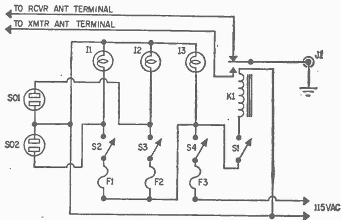
Schematic diagram shows wiring of power distribution center. Transmitter and receiver are plugged into SO1 and SO2, respectively. Switch S4 is master switch for control center. Below, Jerry's rig is set up ready for operation.
