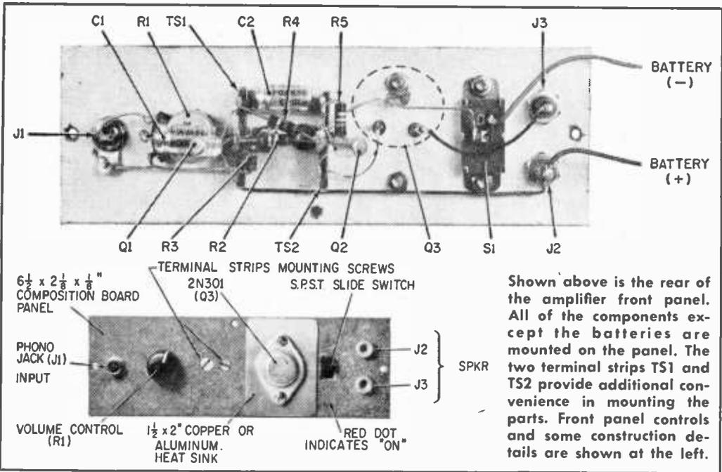
Shown above is the rear of the amplifier front panel. All of the components except the batteries are mounted on the panel. The two terminal strips TS1 and TS2 provide additional convenience in mounting the parts. Front panel controls and some construction details are shown at the left.
