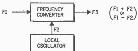
**A Frequency converter Block diagram.**
