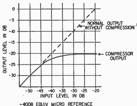
Graph plots C-577's compressor performance with controls adjusted as per unit's manual.
