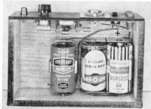
The three batteries of the solid-state amplifier are easily replaced from the bottom.
