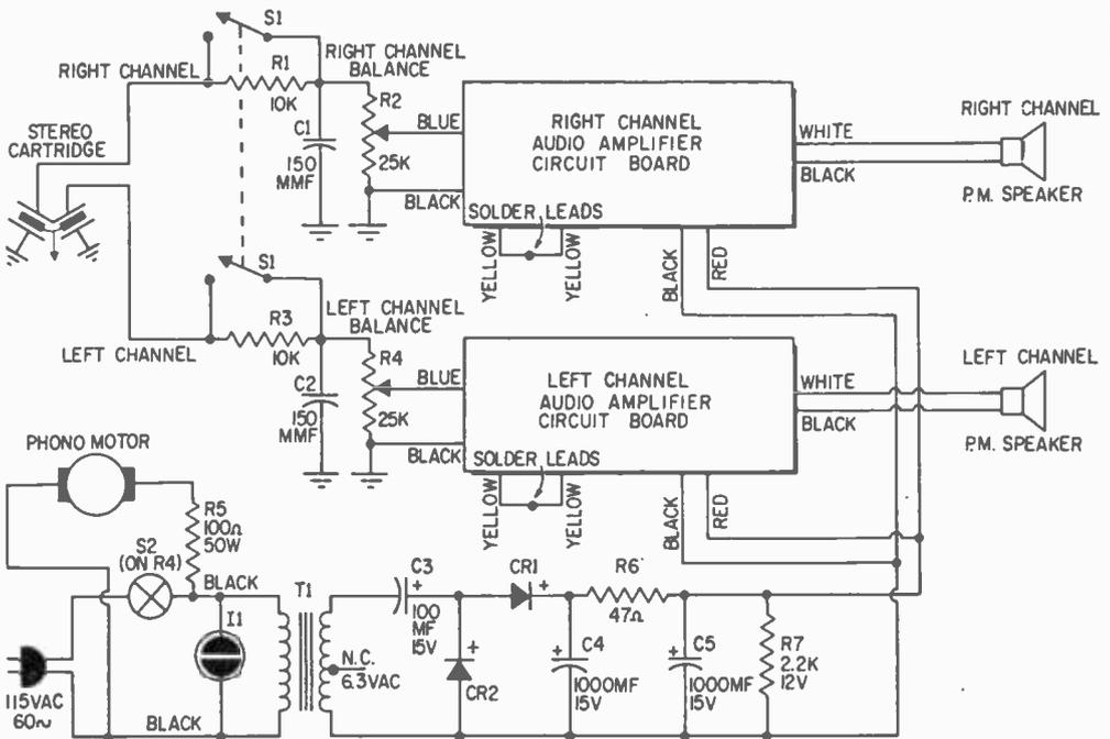
transformer is located. You will then keep all AC components away from the crystal input, eliminating possible hum pickup.
