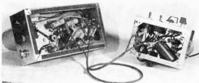
Several sets of patch cords like these are good for making temporary connections while checking newly constructed or modified equipment. A few feet of lamp cord, with an alligator clip soldered to each end of each wire is all that's necessary. A spot of paint can be added for color-coding so you can match up the correct clips at either end.
