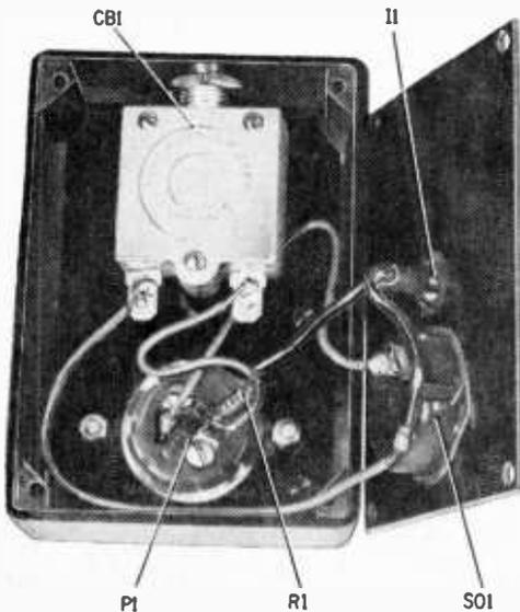
Detail drawing, top, pinpoints location of holes for mounting components. The schematic diagram, above, shows how I1 is paralleled with the circuit breaker to light when CBI opens. At the right is the back of the plastic case showing the AC plug, P1.
