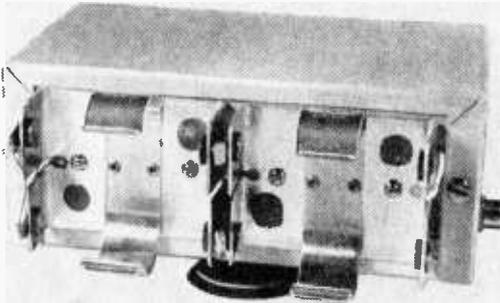
Side view of chassis shows speaker jack, J1, which is insulated from the chassis using a small square of bakelite. Rear view of the chassis, left, gives details of mounting the battery clips. Clean front panel of easy-to-operate unit is shown in shot above.
