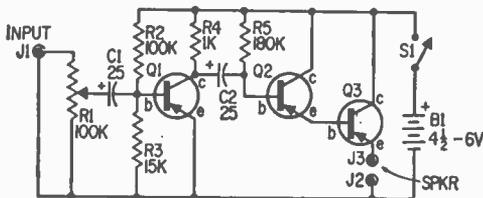
Wire amplifier using the schematic diagram.
