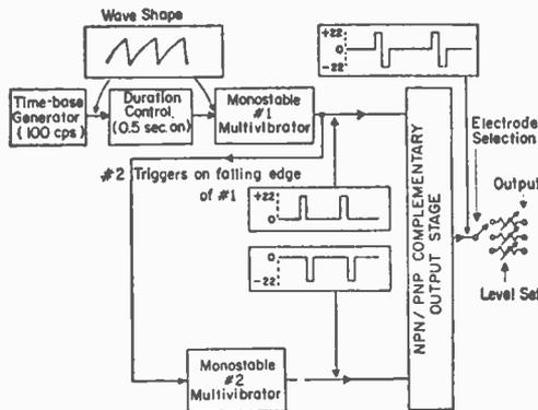
Block diagram of the Subcortical Stimulator, manufactured by Technical Associates of New Orleans, for experiments with ICSS in man.
