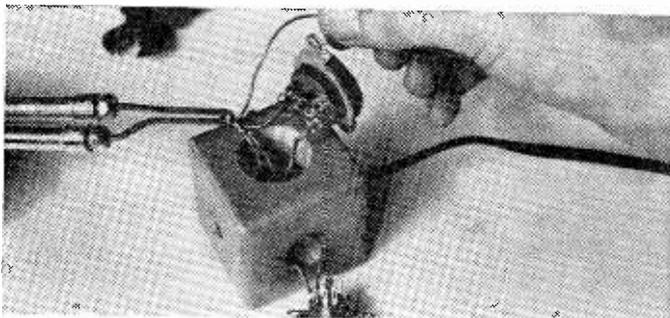
Wiring can be quite a chore for an all-thumbs wiper in the close confines of the wooden block—nothing is to prevent you from using a plastic case or a standard chassis box to hold the circuitry. Add a pair of metal strips to test fuses and lamps.
