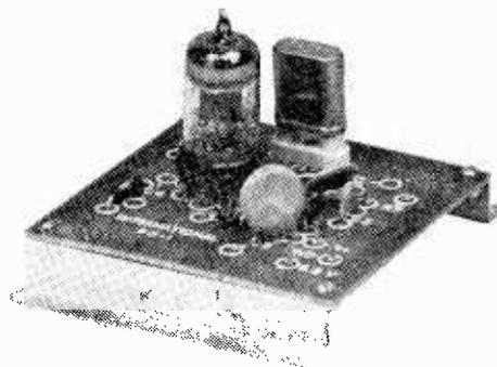
Improved accuracy of the BC-221 and LM frequency meters is due to this little FO-1 crystal oscillator manufactured by International Crystal as a subassembly.
