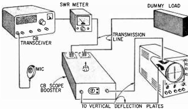
Setup for checking the CB rig's percentage of modulation requires considerable equipment—SWR meter, Dummy load (to replace antenna), and scope. Size of CB Scope Booster, as shown here, is greatly exaggerated in size. All interconnections should be made as short as possible for testing.
