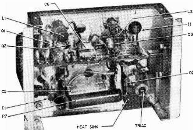
Inside view of chassis shows major components. Inductive coupling between L1 and L2 could cause Q2 to oscillate. Oscillations can be stopped by reversing wire leads to L2 or mounting L1 in end of the chassis parallel to chassis board—right angle to L2.
