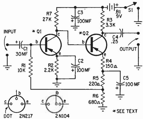
Super-Gain Amp circuit has direct-coupled transistors and bias network (R1, R4, R5 and R6) to reduce effects of temperature.
