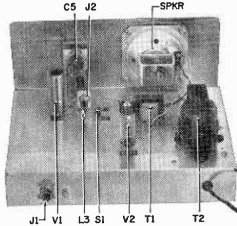
spaced as shown. The plug-in connector for the coil (J2) is mounted on an aluminum bracket approximately 1 in. high by ¾ in. wide. Use a single hole mounting type jack with ceramic insulation.
