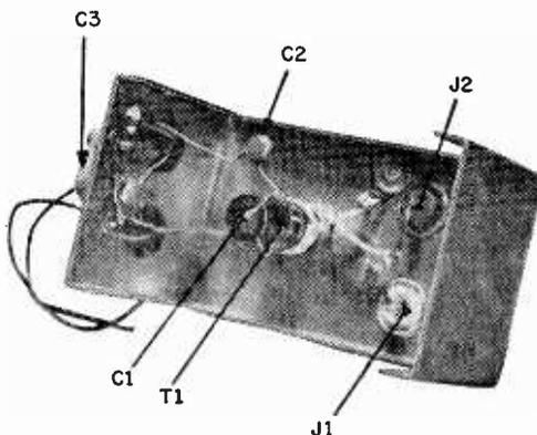
Internal view of the CB Scope Booster shows heavy-wire jumper between J1, J2 and 3-turn coil (L1) added to make T1.
