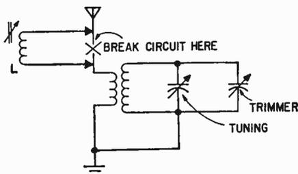
You are correct. The antenna trimmer usually corrects tracking error which is caused by variations in antenna capacitance loading. You can add a variable coil (L) in series with the antenna which functions as an antenna loading coil. The inductance of the coil is changed by adjustment of its ferrite core (Miller 4400 series, etc.) with a threaded rod. Too bad they don't make them with a tuning shaft to which a knob could be attached.
