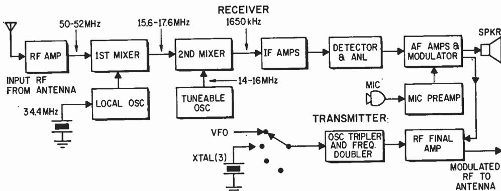
Block diagram shows signal flow in audio and RF circuitry of Knight-Kit TR-106 transceiver
