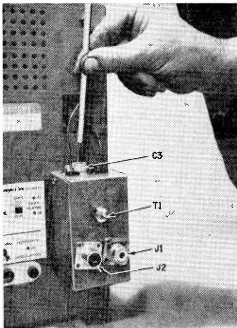
Capacitor C3 is adjusted according to the details in the text. For easier testing a dummy load (phantom antenna) can be built in—eliminating one of the coax connectors on the CB Scope Booster. Load should be shielded from transformer T1.
