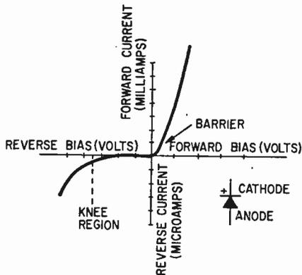
Fig. 1. Typical characteristic curve of a common diode shows forward and reverse current and bias (applied) AC voltages.
