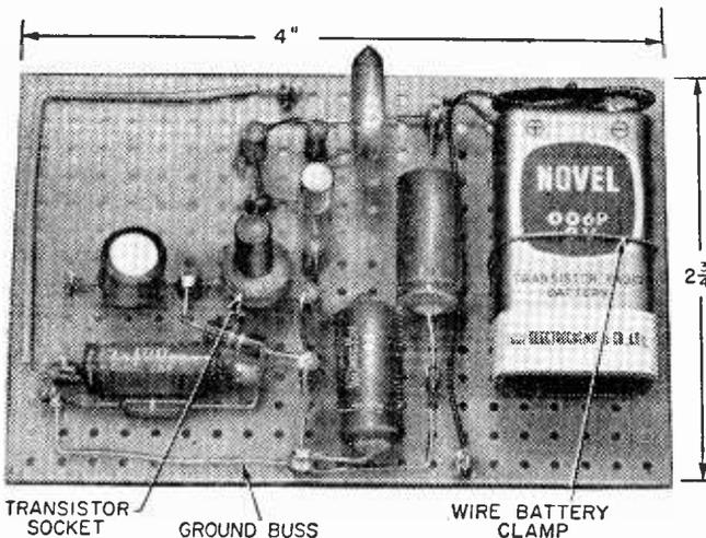
Perf board isn't crowded and it should be quite easy to shave a few square inches off the size if you have to make a smaller unit to fit into a particular cabinet or area of an existing amplifier. For a little more money you can get really miniature electrolytic capacitors—mounted vertically to save space.
