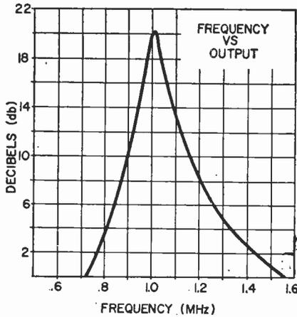
Actual frequency of L2-C6 isn't critical but response (above) must be sharp for best results. Grounding the power supply common lead through a .05 MF capacitor helps sometimes. L1, L2 winding connections and schematic diagram are below.
