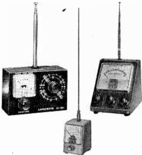
Field-strength meters have no connection to transmitter except through radiation. Lafayette units, above (right and left), Heathkit PM-2 (center) are fine for CBing.
