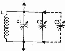
about 35 mmf maximum capacity. In the diagram L represents the oscillator coil, C1 the tuning capacitor, C2 the existing trimmer and C3 the added capacitor. Don't bother with bandspread for the FM band where the stations take up 150 kc and are spaced far apart. You don't need it. A pictorial diagram can't be given since receivers vary considerably.
