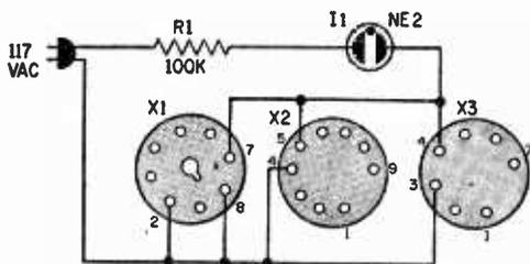
The circuit (above), is simple but you must remember it won't check all of the tubes—filaments on many 5-volt rectifier tubes are pins 2 and 8.
