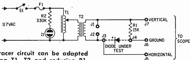
Fig. 3. Dynamic Diode Curve Tracer circuit can be adapted to high-current tests by changing T1, T2 and reducing R1.
