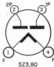
by—if you can't get one locally try a mail order house. Or you could change the socket (or make an adapter) to convert to a 5Y3 octal base tube. The filament connections on the 4-prong tube are the two large-diameter pins. The key on the octal socket is between pins 1 and 8.
