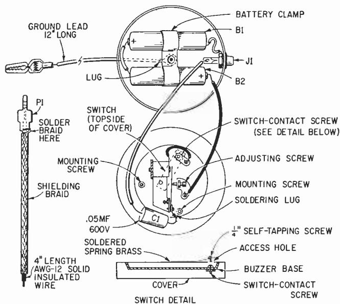
Pictorial diagram (at left) shows how parts are arranged in top and bottom sections of circular container. Batteries should be wired in series.
