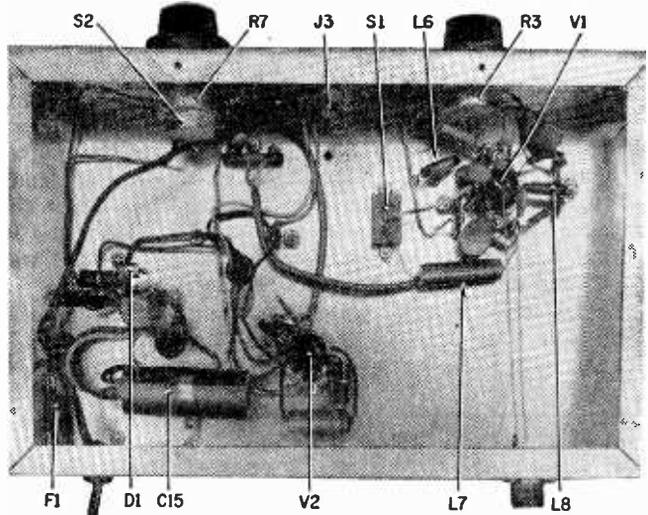
Under-chassis view (right) of VHF receiver shows there is little crowding. Leads to socket of V1 are kept short.
