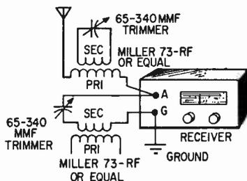
First try realignment. With many home radios, it is almost impossible to separate stations only 10 kc (kHz) apart when one is nearby and powerful. Try using a shorter antenna. Add a parallel-resonant wavetraps in series with the antenna and a series-resonant wavetraps across the antenna and ground terminal as shown in the diagram. Tune one trap to attenuate the 850-kc signal and the other to 900 kc, or both to 850 kc. However, the traps might not be selective
