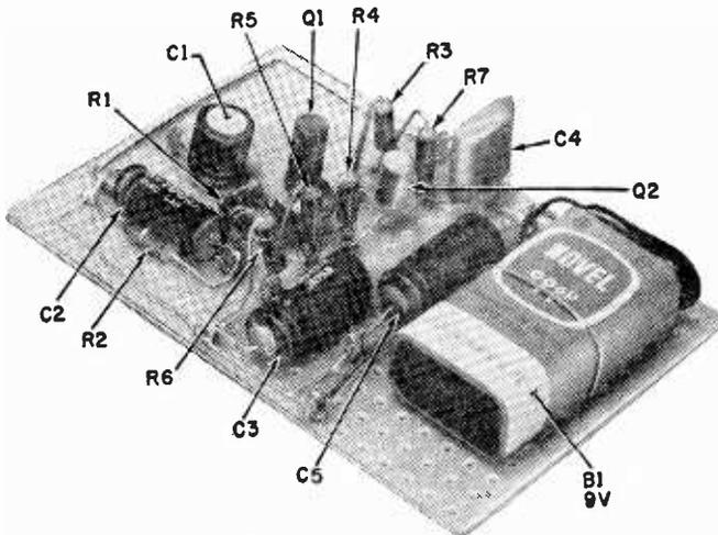
While flea clips are used here as solder terminals any push-in terminal will serve. For a more compact unit eyelets can be set in the holes used and extra pigtail lead-length can be used as under-chassis interconnections. It may not be as neat as a printed-circuit board but it's practical.
