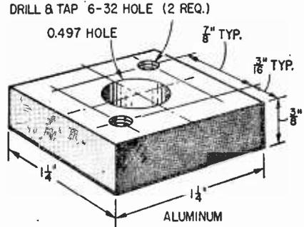
Press-fit heat sink should not be used unless you have a fairly well equipped shop. TRIAC can be broken if improper or unequal pressure is applied to unit.
