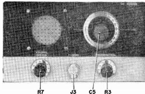
Front panel of the completed receiver is professional looking. Tuning knob for C5 can be replaced with a vernier drive for easier tuning on the communications bands.
