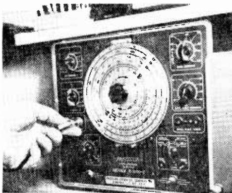
Service-bench signal generator is useful —RF (for receiver alignment) and audio signals (amplifiers) aid troubleshooting.
