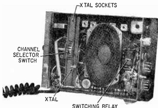
Bottom view of unit shows speaker inserted in maze of the components. Crystal socket is bar at left of speaker. IF and other tuned circuits are at top. Relay, right center, does switching for receive and transmit operations.
