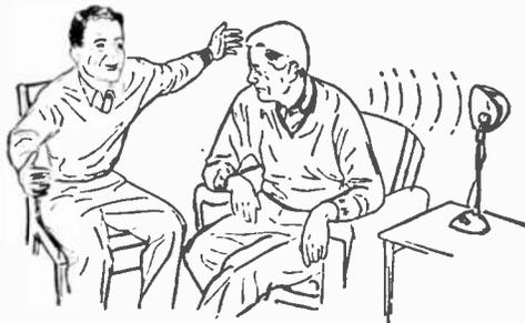
A microphone stand for hand mikes (such as those that come with less expensive tape recorders) can be improvised from a flexible neck desk lamp with its cord removed (or at least disconnected), a plug to fit the lamp's socket, and a  $\frac{1}{8}$  x  $\frac{3}{8}$  in. metal strip. Bend the metal strip to the size
