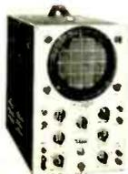
Model 460 Wideband Direct-Coupled 5" Oscilloscope. DC-4.5mc for color and B&W TV service and lab use. Push-pull DC vertical amp., bal. or unbal. input. Automatic sync limiter and amp. \$109.95 kit, \$149.95 wired.
