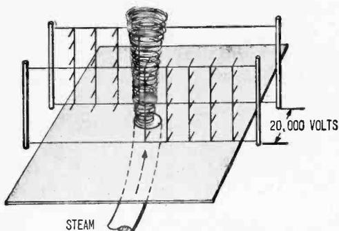
Fig. 9. This asymmetric grid arrangement simulates charged cloud regions over the earth.
