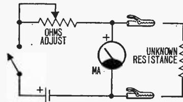
Fig. 2. Slide-back ohmmeter circuit isn’t suitable for high-resistance measurements and isn’t added to most VOMs for low-ohms.
