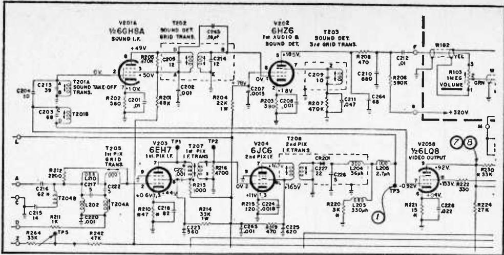
Schematic diagram above is typical of the circuit used in many television receivers. Top half of diagram is the sound IF and audio detector; bottom is video IF, output.
