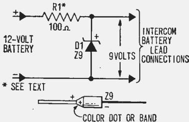
Simple two-component circuit drops output of 12-volt automotive battery to 9 volts. Be sure to watch polarity when connecting the Zener diode and leads between intercom and battery.
