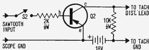
Simple amplifier increases sawtooth amplitude to Tach Stretcher for calibration.
