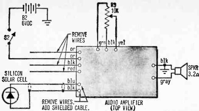
Fig. 5. Schematic diagram shows added components you must connect to use ready-wired transistor amplifier as receiver for infrared transmitter on facing page.
