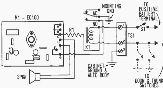
Noisemaker of the *Auto Siren Sentry* is the Eico EC100 (M1) module that drives the speaker. Relay K1 keeps siren sounding.
