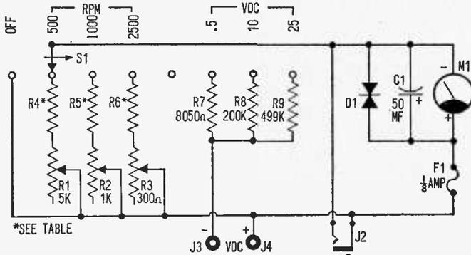
Tach Stretcher schematic diagram (above) is all you have to wire up to convert your present tachometer to read those very-low RPMs. Schematic diagram of tachometer (below) is for a Knight unit but method of adding the plug-in jack (J1) is typical of all the single-range tachometer accessories for high-performance autos.
