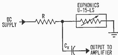
**Simplified circuit of Euphonics system shows need for DC power source and amplifier. Cartridge effectively serves as a voltage divider.**
