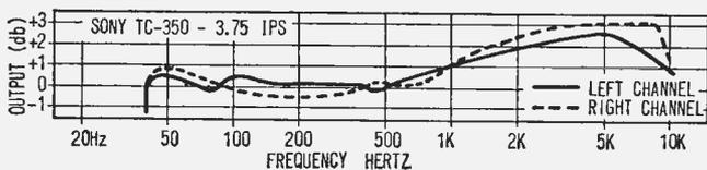
Curves show overall record/play response at both 3¾- and 7½-ips speeds for Sony 350 tape recorder (the identical tape deck, mounted in a carrying case for portable use, is also available as the Model 350C). Note that response actually extends to a low 20 Hz at the faster 7½-ips speed.
