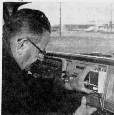
Master intercom unit is mounted on dash of pickup truck. Make sure wiring isn't dangling—tape it securely to bracket behind dash.
