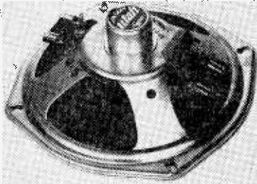
Utah multi-impedance speaker has plug-in terminals (above) while speaker in AC/DC set (see below) uses typical solder connection.
