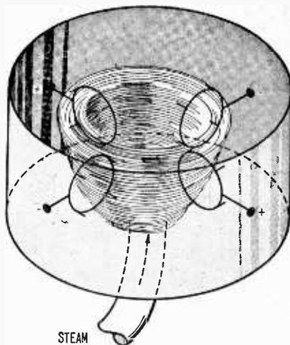
Fig. 7. With charged grids mounted in a circle, steam (injected at bottom) formed a rapidly turning tornado-like vortex in test chamber.
