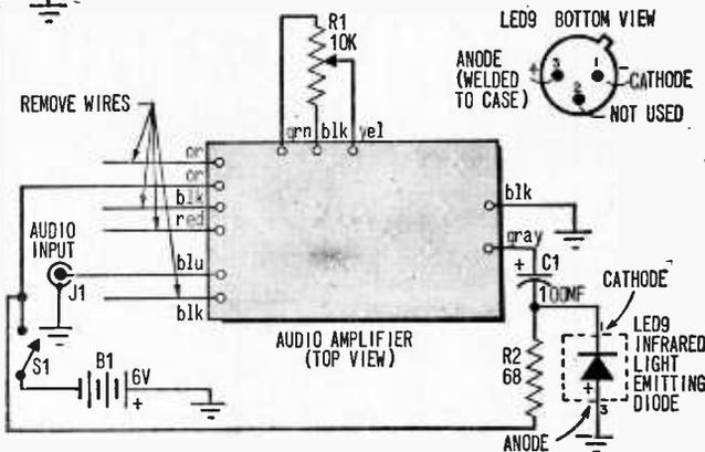
high-current, short-duration pulses. This special class of emitting diodes are sometimes referred to as *laser* diodes. The emitted light output of the GaAs diode can be amplitude modulated, and the operation is similar to an AM transmitter. GaAs diodes have inherently fast response and can therefore be modulated up to about 100 MHz. Audio and video information can be easily transmitted by these diodes.
