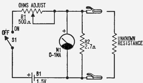
Fig. 3. Schematic diagram of Mini-Ohmer has only one difference from circuit in Fig. 2—R2 in shunt with meter. Meter indicates IR drop across R2 and unknown.
