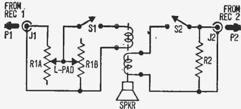
Signal Center schematic diagram shows two methods of connecting to the receivers. A load resistor (R2) can be used in place of the pad (R1) or two pads can be wired in the circuit.
