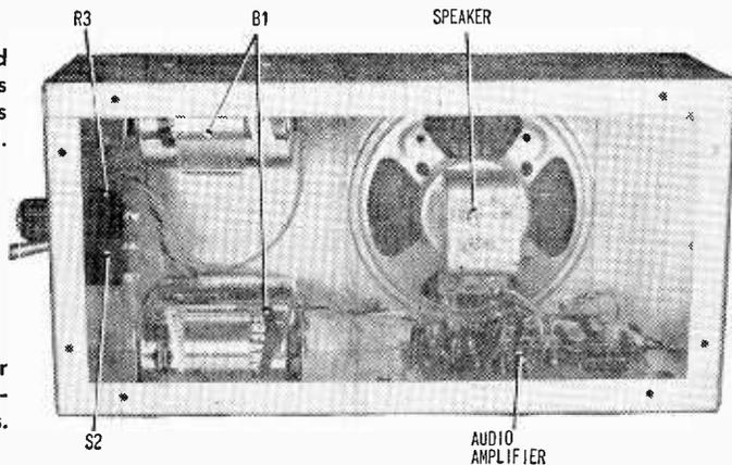
Fig. 11. Insides of the receiver shows speaker, amplifier, battery B1 and panel controls.
