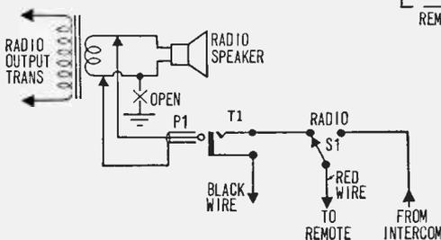
**Modification.** Before attempting to re-wire the intercom drill all necessary holes in the plastic case of the master unit. Two 1/4-in. holes are put in the right-hand bottom-end of the plastic case. One hole provides an entrance for the 12-volt leads. The other 1/4-in. hole is for the radio speaker wires. At the top center of the master unit drill a 3/8-in. hole to mount the s.p.d.t. toggle switch.
