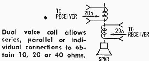
dependent of the other, and each voice coil can be connected to an individual receiver.
