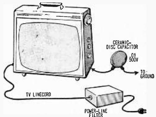
**Metal-cabinet TV sets are easy to ground but plastic and wooden cabinets do not act as shielding unless lined with metal foil.**
