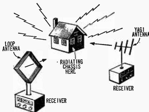
**Some sources of ITV must be tracked with direction-finding techniques. Loop and Yagi antennas are easily made and should be tuned to the interference frequency.**
