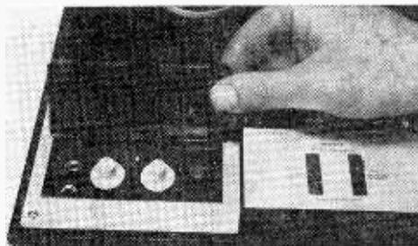
Snap-open door on top left conceals the 350's mike jacks and record level controls. Two mode switches are directly below heel of hand.
