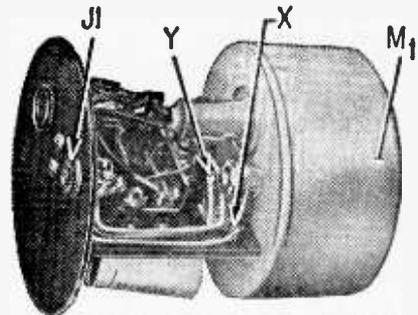
Internal view of Knight tachometer shows location of J1 and added solder terminal.
