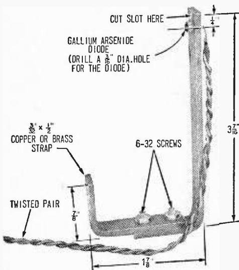
**Fig. 8. Diode mounting bracket (left) holds diode in focal point of mirror.**
