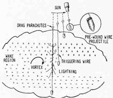
Fig. 11. Wires might be launched through charged area using coiled-wire projectile.
