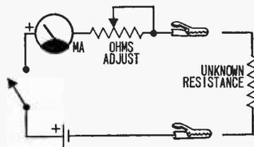
Fig. 1. Basic ohmmeter circuit is the same as that in most VOMs. Short clips and set ohms adjust for zero indication.
