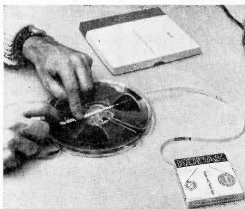
Adding leader-timing tape protects tape during threading operation. "No-trim" tabs let you make splices right on the reel.
