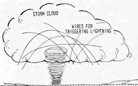
Fig. 10. In theory, a tornado conceivably could be short-circuited by launched conductors.
