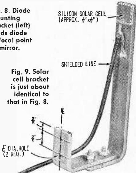
**Fig. 9. Solar cell bracket is just about identical to that in Fig. 8.**
