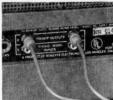
Outputs from master unit should ideally come from preamps. This way, any distortion in unit's power amps can be bypassed.
