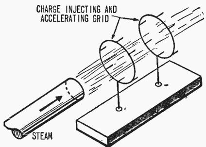
Fig. 6. A linear accelerator was used to study grid shapes. Wire points, directed downstream of steam jet, were found necessary in order to achieve maximum vapor acceleration.
