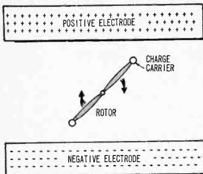
Fig. 2. Diagram of electrostatic motor shows how rotary motion is developed in vortex by effect of accumulated high-voltage charge.
