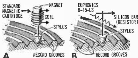
**Standard magnetic cartridge and newer solid-state type do same thing, but in entirely different manners. Stylus in standard cartridge moves magnet or coil to generate voltage output; stylus in Euphonics unit simply varies resistance of silicon bar to produce signal.**
