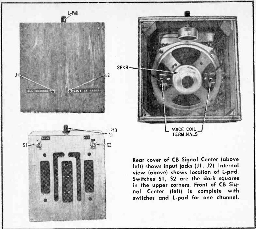
Rear cover of CB Signal Center (above left) shows input jacks (J1, J2). Internal view (above) shows location of L-pad. Switches S1, S2 are the dark squares in the upper corners. Front of CB Signal Center (left) is complete with switches and L-pad for one channel.
