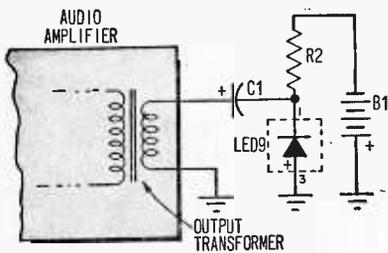
Fig. 2. Simplified schematic of output circuit used to modulate gallium-arsenide diode.
