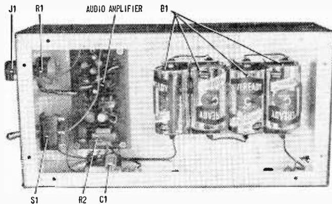
Fig. 10. Completely wired transmitter (above) only needs to have mirror and GaAs diode mounted at one end.
