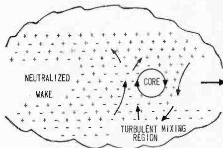
Fig. 4. As charge builds up a core or vortex is created. Core advances along charged area leaving a neutralized wake which often contains both rain and hail as well as light.
