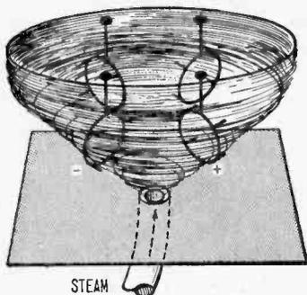
Fig. 8. The circular grid arrangement produces an electrostatic vortex over a ground plane when cylindrical boundary is absent.
