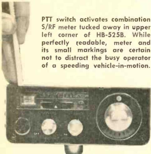
PTT switch activates combination S/R/F meter tucked away in upper left corner of HB-525B. While perfectly readable, meter and its small markings are certain not to distract the busy operator of a speeding vehicle-in-motion.
