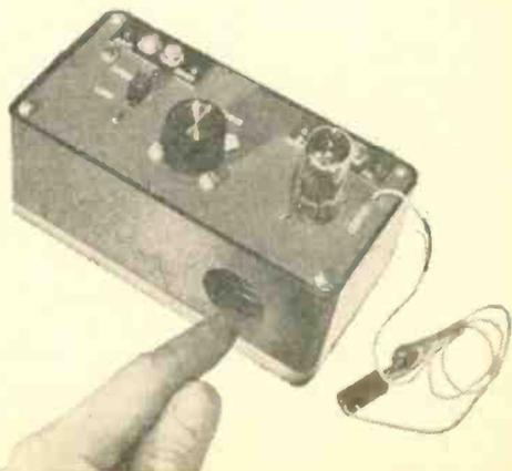
A 1-in. access hole is made in the case for entry of the GDO coil. The hole lines up with L3 inside the case.
