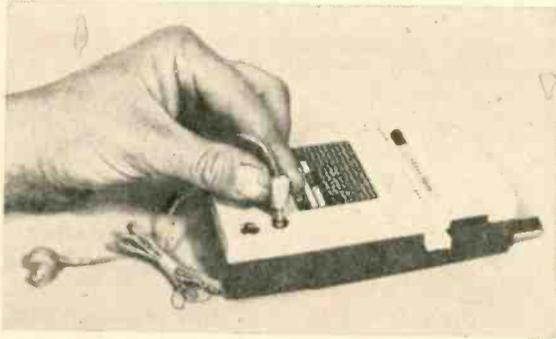
Common source of "no sound" is flimsy headphone jack (above) which might fail to make normal/through-speaker connection; remedy is to clean or replace jack in effort to increase spring tension. At right, non-technical users often assume W-T is defective when selector has been accidentally moved to unused channel.
