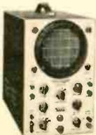
Model 460 Wideband Direct-Coupled 5" Oscilloscope. DC-4.5mc for color and B&W TV service and lab use. Push-pull DC vertical amp., bal. or unbal. Input. Automatic sync limiter and amp. \$99.95 kit, \$139.95 wired.
