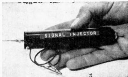
Completed Mini-jector is ready to go to work tracking down the culprit in just about any piece of electronic gear, from hi-fi tuners to public address systems.
