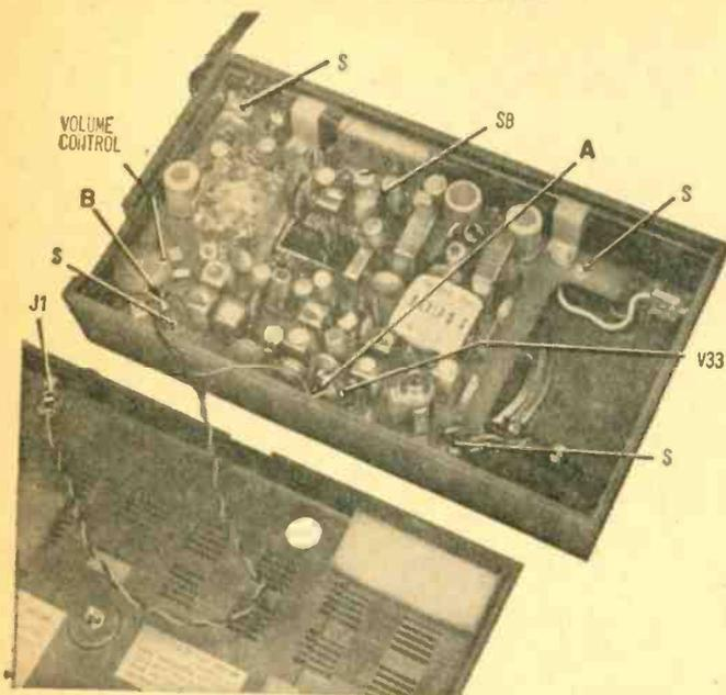
Circuit board on Patrolman receiver must be lifted so wires to J1 can be soldered in place. This is accomplished by removing screws marked S and SB.
