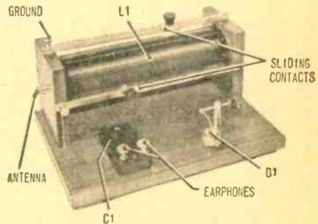
Completed receiving apparatus is good performer when outdoor antenna and ground are connected. It looks pretty snazzy, too.
