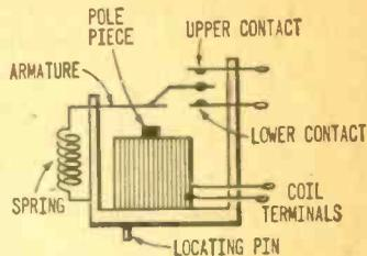
Fig. 3. The only critical part in building Shush Box is adjusting relay K1 above. Detailed instructions are given in text and should be followed.
