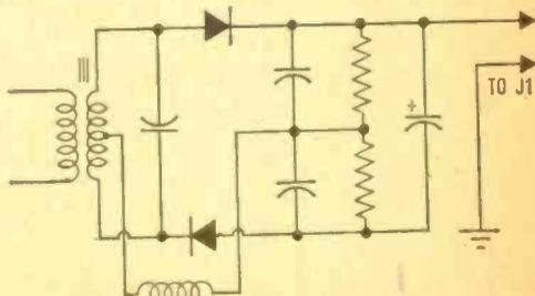
Shush Box can be added to any receiver using a ratio detector. Typical circuit above shows how detector output is hooked to J1.
