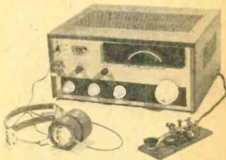
Heathkit's new transceiver designed especially for the Novice runs up to 90-watts transmitter input but has meter marking for 75. The rig features break-in operation and a tunable dual-conversion receiver section.
