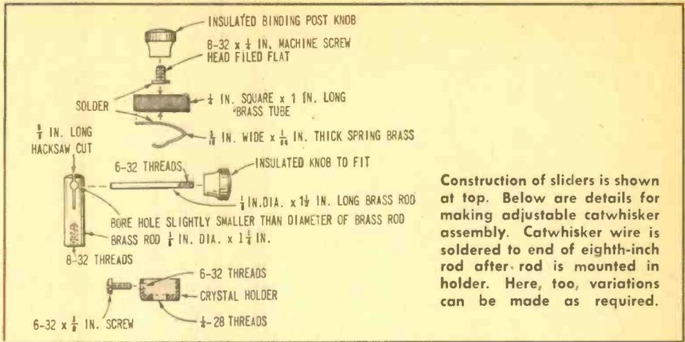
Construction of sliders is shown at top. Below are details for making adjustable catwhisker assembly. Catwhisker wire is soldered to end of eighth-inch rod after rod is mounted in holder. Here, too, variations can be made as required.
