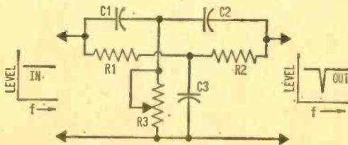
Secret of Hum Bug's success is the parallel-T filter. Tuning rejection frequency is accomplished by varying setting of R3; positive feedback tends to narrow rejection notch.
