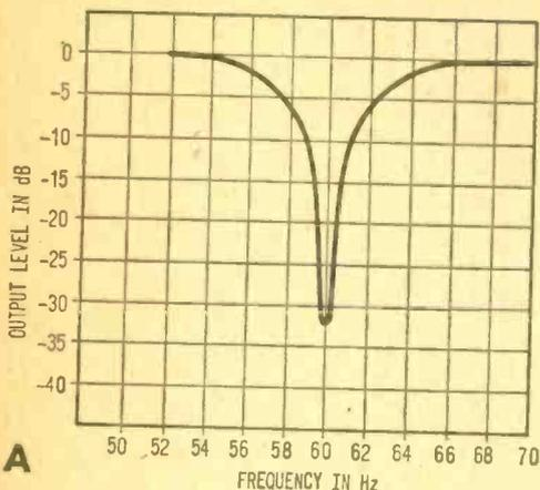
**A** Hum Bug's sharp rejection of 60- and 120-Hz hum frequencies is shown in curves A and B, respectively. Positive feedback increases effective Q sharpness of parallel-T filter.
