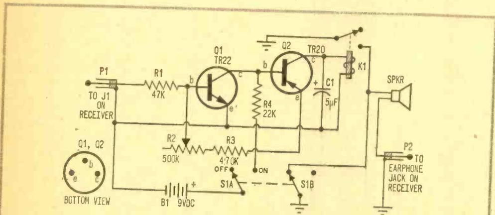
Fig. 2. Schematic diagram of Shush Box. Circuit functions as a simple amplifier energizing relay K1 whenever receiver picks up a signal.
