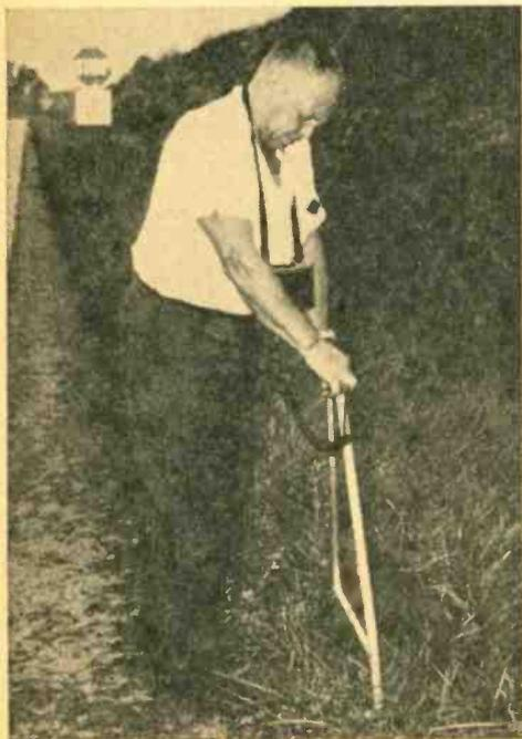
Probing cable's course with contact frame, operator watches first for peak reading, then for null indicating exact position of break.
