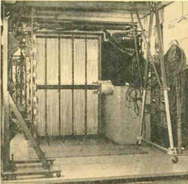
Here's the ten-ton Columbia University aluminum spark chamber installed at the Alternating Gradient Synchrotron for the 1962 experiment which showed that there are two types of neutrinos. One type produces only electrons (with positive charge) in collision with protons; the other produces only mu mesons.
