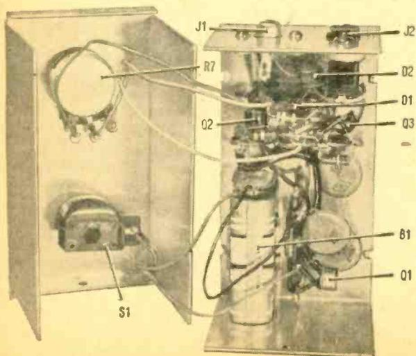
Parts layout isn't critical and any arrangement should work. In prototype, terminal strips are used for mounting components.
