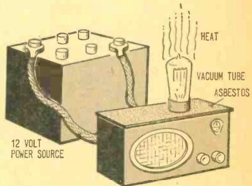
Fig. 5. Follow the above layout (more or less) when substituting a vacuum tube for the transistor you ruined by careless handling.
