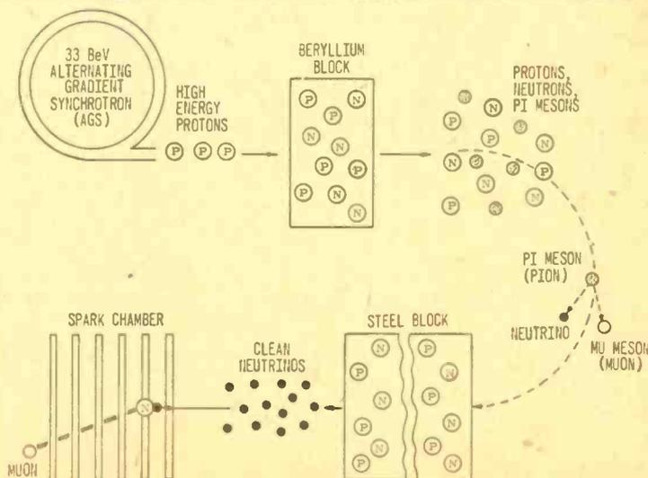
A flow diagram on how to find the elusive neutrino. Steel block "cleans" neutrinos by stopping all other particles before entry to spark chamber.
