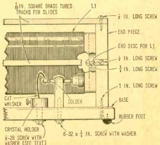
Assemble the finished coil, sliders, crystal, and condenser following detail drawing above.
