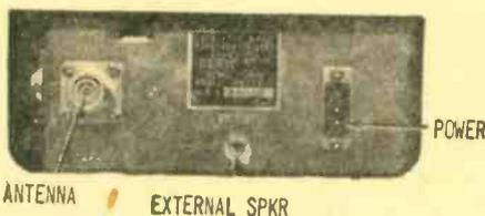
The receiver's rear panel has jacks for the required external antenna, the 12-VDC power source, and an external remote speaker.
