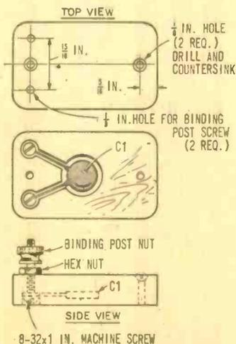
Replica of Murdock phone condenser is made from a wood block drilled to hold a small disc capacitor and phone binding posts. After block has been cut out, drilled, and sanded, paint it flat black for antique appearance.
