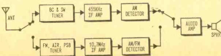
Allied's portable all-band receiver employs two separate IF strips and three detectors for full coverage of five major communications bands.
