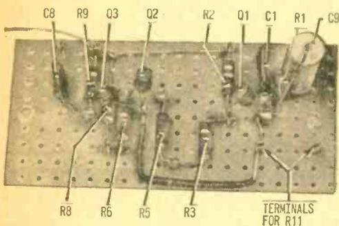
Most components except for power supply are mounted on perfboard subchassis. Follow photo for approximate layout to avoid parts clutter; see text for info on resistor R11.
