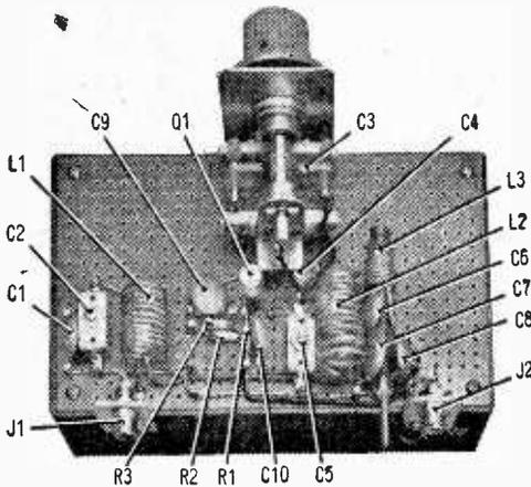
Here's the completed CB Grabber, all hooked up and rarin' to go. Needed: an antenna into jack J1, a lead to a BCB set from jack J2.
