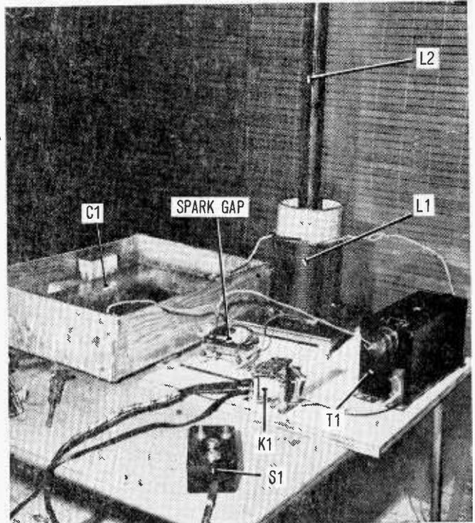
Completed Lightning Generator stands ready to go with all of a million volts! Wiring between components is AWG-12 or 14.
