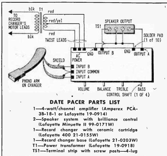
*pads*, pre-tinned spots on the printed-circuit board approximately ¼-in. square.
