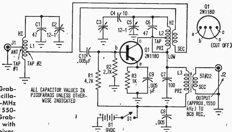
Schematic of the CB Grabber reveals simple oscillator that converts 27-MHz signals at J1 into 1550-kHz signals at J2. Grabber must be used with a broadcast-band receiver.
