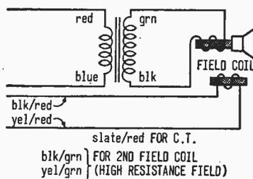
The diagram shows the standard color coding. If the output transformer is mounted on the speaker, the leads running to the transformer primary are probably blue and red
