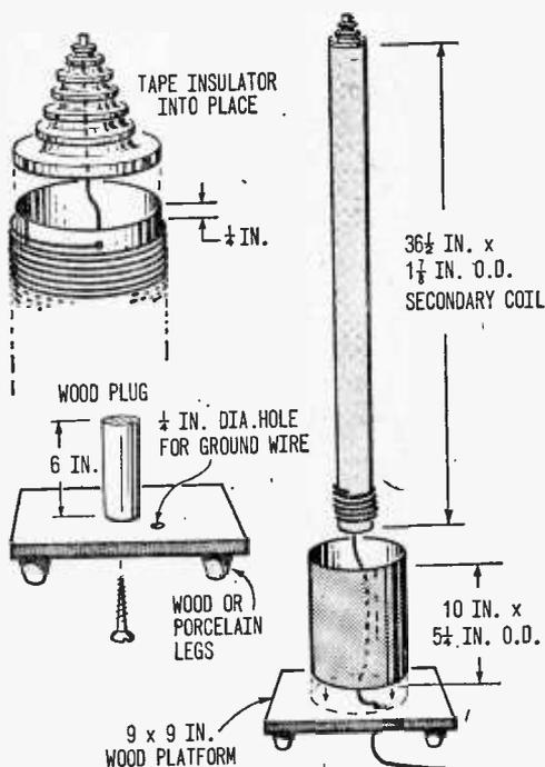
Platform for coil L2 is made from 9 x 9 in. square of 1/2-in. plywood.
