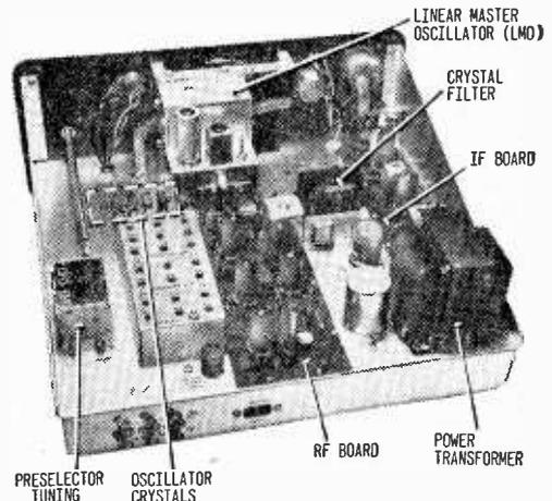
Though the SB-310 is jam-packed with features, chassis layout is neat and wide-open.
