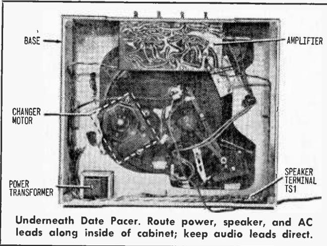
Underneath Date Pacer. Route power, speaker, and AC leads along inside of cabinet; keep audio leads direct.
