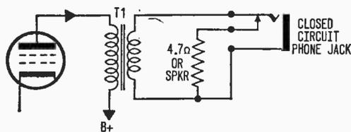
Yes, you can omit the speaker as shown in the diagram. And you can use a coil with more inductance in order to tune to lower frequencies.
