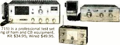
EICO Trans/Match (Model 715) is a professional test set designed for complete checking of ham and CB equipment. Kit \$34.95; Wired \$49.95.
