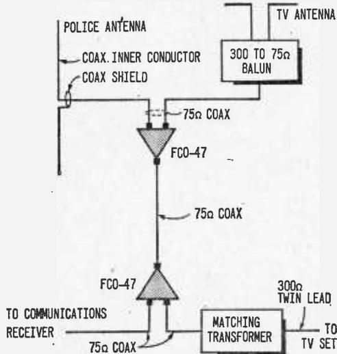
47 through the same kind of coax and a 75-ohm to 300-ohm matching transformer. All connections to the FCO-47's must be made with suitable coax connectors. The FCO-47 (available from Jerrold Electronics, 401 Walnut Street, Philadelphia) passes signals from 5 to 47 MHz
