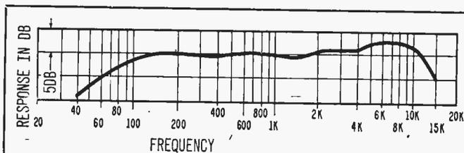
Fig. 2. Smooth as it is, frequency response of the 631 fails to reveal unit's relatively low distortion and freedom from breakup—two very potent factors affecting performance.
