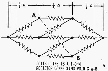
Now, all resistors fall into one of three parallel groups that are in series with other groups. The first group on the left consists of three one-ohm resistors, which effectively add up (or is it down, in this case?) to  $\frac{1}{3}$  ohm. The same summation is true for the group on the right. The center group consists of six resistors and sums to  $\frac{1}{6}$  ohm. Hence, when you add up  $\frac{1}{3} + \frac{1}{6} + \frac{1}{3}$ , the answer comes to  $\frac{5}{6}$  ohm.
