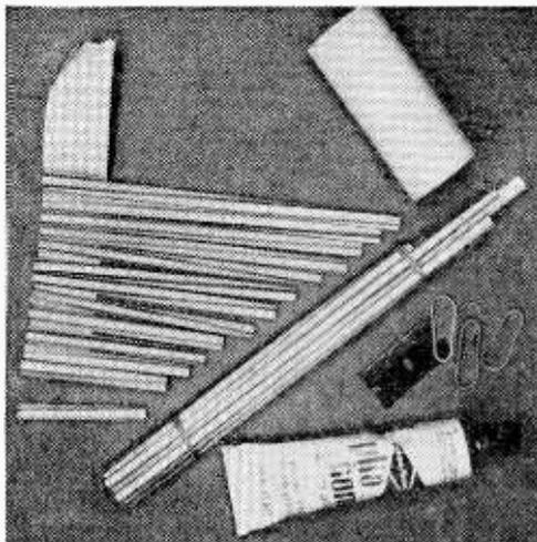
Here's what your workbench will look like part way through the construction. Straws are kept in place by sticking them to some masking tape. Other construction items are Pliobond cement, razor, rubberbands and white plastic hood. See photo below.
