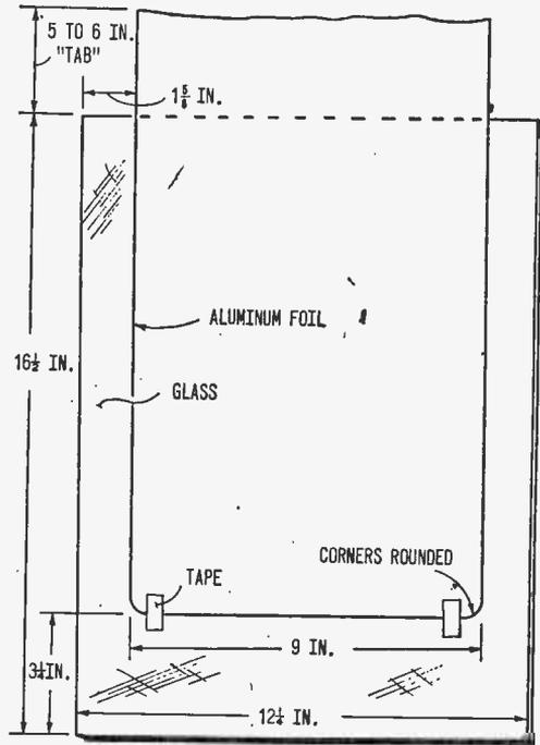
Aluminum foil is taped to the glass foil-side up, with tabs protruding from opposite ends.
