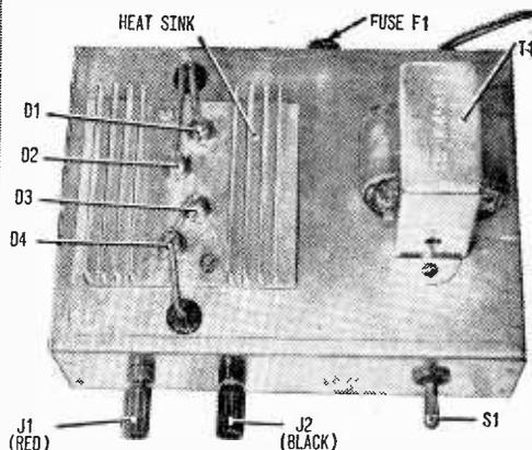
Top and bottom views of Charger, showing parts placement. Diodes run cool as cucumbers due to high conductivity of heat sink.
