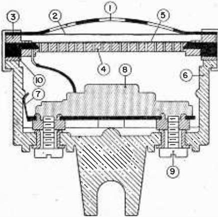
A cross-sectional view of the electret transmitter showing (1) screen, (2) dust and humidity cover, (3) contact spacer, (4) perforated back plate, (5) electret diaphragm, (6) cup, (7) contact spring, (8) amplifier assembly, (9) screw terminals and (10) contact ring. This new electret microphone fits directly into the present telephone handset with no modifications.
