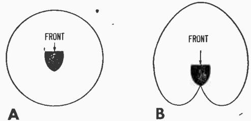
Fig. 1. Though mikes are similar in design, 631 has an omnidirectional pickup pattern (drawing A), 627 a cardioid pattern (drawing B).
