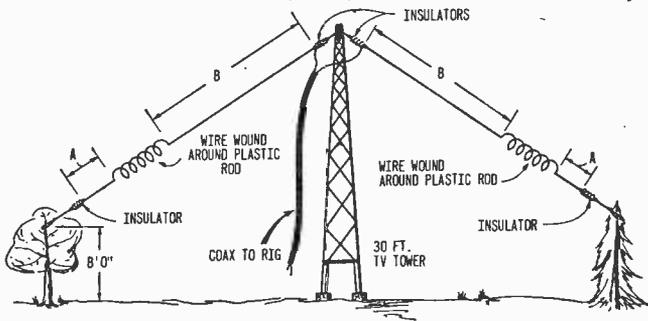
W7DQS made use of a 30-ft. TV mast and a couple of trees to support his 80/40 doublet, but your installation needn't be the same. Lengths *A* and *B* were 4 ft. 6 in. and 35 ft. 10 in. in his case — exact dimensions must be determined through use of an SWR bridge as described in text.
