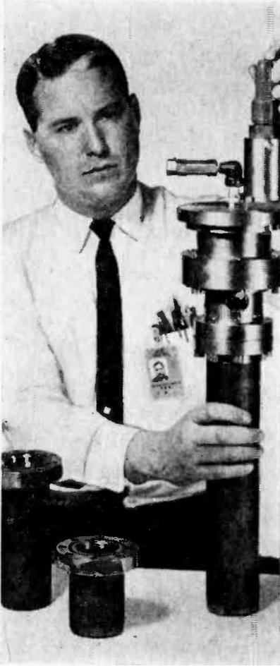
Used for seismic measurements, digital-air gun by Texas Instruments (above) is electro-mechanical device that forces air bubbles of predetermined sizes under water. Below, ship-board oceanographic system, also developed by Texas Instruments, digitizes, corrects, linearizes, arranges, and plots variety of data.
