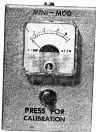
High-speed meter has expanded scale between 0.2 and 0.8 so CB accessories such as speech compressors and clippers can be readily adjusted.
