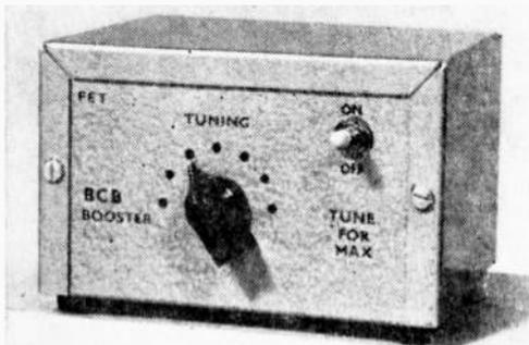
Booster covers entire BCB with single tuning capacitor. No calibration is necessary—you simply tune for maximum signal.
