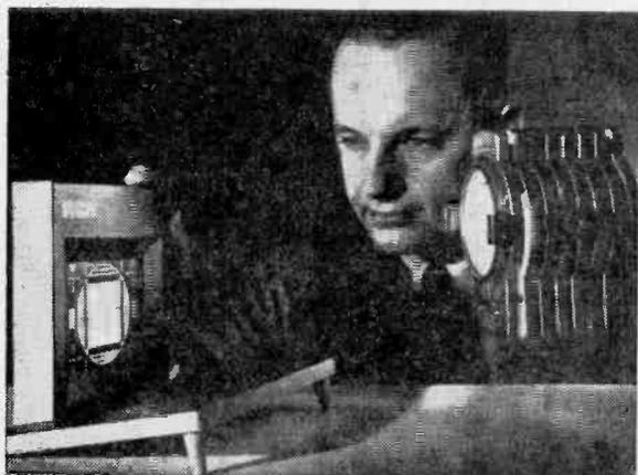
Here are some highlights of RCA liquid window. Top photo shows two windows: left one is clear; right one is opaque. Middle photo shows scientist putting drop of liquid crystal between two plates. Bottom photo shows potential TV application giving bright and clear picture even though window is illuminated by a 500-watt stage floodlight.
