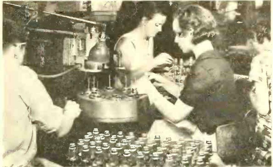
Welding metal-tube shells in the Raytheon factory. The complete assemblies are placed upside down in the rotating welder table.
