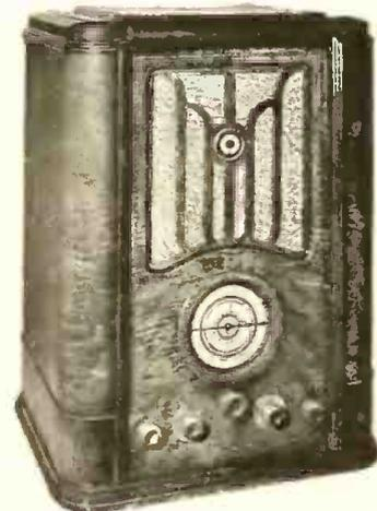
★ Metal-tube superheterodyne with 12 tubes featuring cathode-ray tuning indicator. Four band tuning with selective dial lighting—bass accentuator and static reducing control. Triode power detection and automatic volume control. Designed for export and tropic use as well as domestic. Pilot Radio Corp., 37-06 36th St., Long Island City, N. Y.—**RADIO TODAY**
