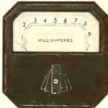
★ DS meter of D'Arsonval type with unusually long scale (4¼ in.)—jewelled pivots. Semi-flush type mounting—bakelite case. Accuracy within 2 per cent—made in all popular current and voltage ranges. Mounts through 2¾ in. diameter hole. Hoyt type 573—10 milliamperere movement—list \$8.50. Burton-Rogers Co., 755 Boylston St., Boston, Mass.—**RADIO TODAY**
