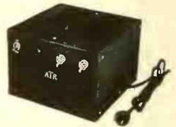
★ Power supply designed to take place of storage battery in demonstrating auto radios—delivers pure direct current for operation of any set. Employs full-wave dry-disc rectifier. Equipped with fuse and pilot light—operates from 105-125-volt AC line. ATR auto radio "A" battery eliminator—net \$12.95. American Television & Radio Corp., 128 E. 10th St., St. Paul, Minn.—RADIO TODAY
