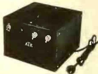
★ Power supply designed to take place of storage battery in demonstrating auto radios—delivers pure direct current for operation of any set. Employs full-wave dry-disc rectifier. Equipped with fuse and pilot light—operates from 105-125-volt AC line. ATR auto radio "A" battery eliminator—net \$12.95. American Television & Radio Corp., 128 E. 10th St., St. Paul, Minn.—RADIO TODAY
