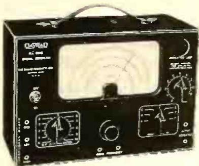
★ Test oscillator using fundamentals on all bands covering 60 to 60,000 kc. Cast aluminum case with compartments for individual circuits—Faraday shield isolates instrument from AC lines. Has 6E5 tube for output indicator—modulated output at 400 cycles. Size 10 x 7 x 4½—weight 10 pounds. DayRad model 36-A—net \$36.75. Radio Products Co., 125 Sunrise Pl., Dayton, Ohio—RADIO TODAY
