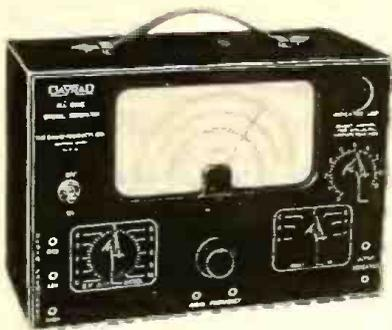
★ Test oscillator using fundamentals on all bands covering 60 to 60,000 kc. Cast aluminum case with compartments for individual circuits—Faraday shield isolates instrument from AC lines. Has 6E5 tube for output indicator—modulated output at 400 cycles. Size 10 x 7 x 4½—weight 10 pounds. DayRad model 36-A—net \$36.75. Radio Products Co., 125 Sunrise Pl., Dayton, Ohio—RADIO TODAY
