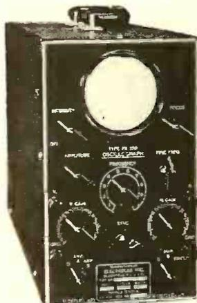
★ Oscillograph for service and laboratory work. Sweep has extremely fast return allowing waves up to 1 megacycle to be observed—no amplifier used on sweep. Sweep frequency independent of amplitude adjustment. Amplifier on horizontal and vertical plates. Weight 22 pounds. Model PR100—list \$84.50. Electrolab, Inc., 15 Ward St., Bloomfield, N. J.—RADIO TODAY
