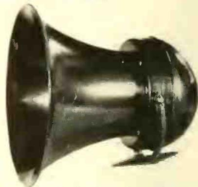
★ Speaker horn for use with ten-inch dynamic speakers—projects sound in desired direction thereby saving on amplifier power. Constructed of spun brass with black enamel finish. Mounted on searchlight type bracket. 18-inch bell and 17 inches long—weight 5 pounds. Model 42. Operadio Mfg. Co., St. Charles, Ill.—RADIO TODAY
