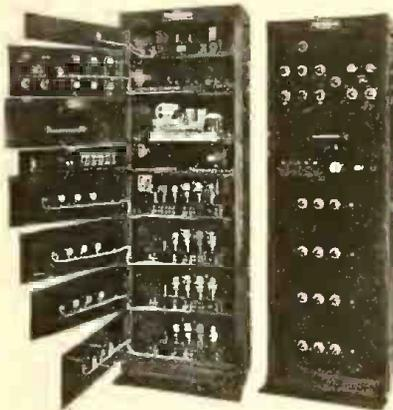
★ Rack and panel for amplifiers and sound systems. Removable panels attached to channel by continuous hinge on one side and screws on other—provides for easy servicing. Sides and rear provided with steel dust cover. Can be placed against or built into wall. All work can be done from front of rack. Type RH-1. Radio Receptor Co., Inc., 106 7th Ave., New York City—RADIO TODAY—see also advt. p. 32.
