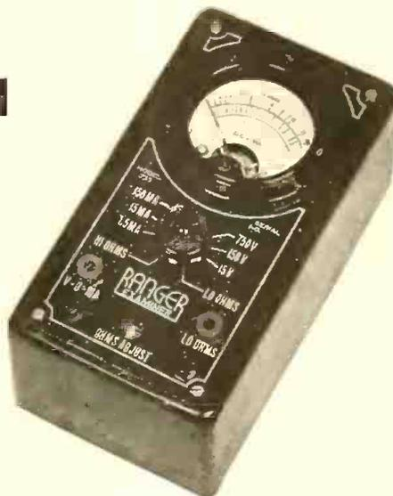
Reads D.C. 15-150-750 volts at 1000 ohms per volt; 1.5-15-150 Milliamperes; 1/2-1000 low ohms; 0-100,000 high ohms at 1.5 volts.
