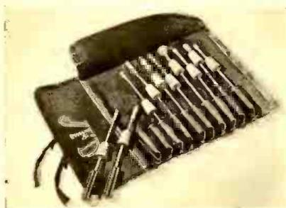
★ Set of 10 wrenches for aligning and tuning the set in car or on the bench. Flexible shaft and adjustable bushing. No need to remove shaft and head from car. Complete in leatherette roll—net \$4.50. J. F. D. Mfg. Co., 4111 Ft. Hamilton Pky., Brooklyn, N. Y.—**RADIO TODAY—see also advt. p. 65.**
