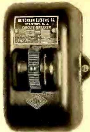
★ Magnetic circuit breakers for protecting tubes and amplifier equipment. Available in models for 50 milliamperes to 35 amps. Time-delay type trips in about 1/100 of a second on short circuit—5 seconds to 8 minutes on 125 per cent load. Instantaneous type may be adjusted for plus or minus 20 per cent of rating. Heineemann Electric Co., Trenton, N. J.—**RADIO TODAY**.
