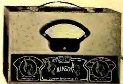
★ AC-DC operated instrument measuring AC and DC volts 0/15/150/750. On AC non-reactive to 10 megacycles. Capacity ranges .001 to .1, .1-32 mfd. Resistance—.03 to 500, 500 to 5 megs. Inductance 2-1000 henries. Housed in wrinkle-finish shield cabinet. Weight 4 pounds. Superior Instruments Corp., 136 Liberty St., New York, N. Y.—**RADIO TODAY—see also advt. p. 69.**
