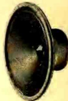
★ 5-inch permo-dynamic speaker using Nipermag alloy for field. Dust-proof voice coil—polyfibrous speaker cone for large frequency response. Available in 2 models  $5\frac{3}{4}$ -inch diameter with mounting holes— $5\frac{3}{4}$  diameter without mounting holes. Cinaudagraph Corp., Stamford, Conn.—RADIO TODAY—see also advt. p. 98
