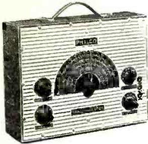
★ Precision type AC operated all-wave oscillator. Tunes 115 to 37,000 KC in 5 bands. Large direct reading scale with commonly used adjusting frequencies marked. 400-cycle audio modulation. Moisture-proofing insures permanency of calibration. Mirror-polished brass panel, unaffected by line voltage variations. Model 077—net \$27. Philco Radio & Television Corp., Tioga & C Sts., Philadelphia, Pa.—**RADIO TODAY**.
