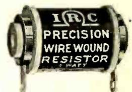
★ Wire-wound type resistor for use with precision equipment. Made in values up to 1¼ megohms—extremely small, 1¼ long by ¾ diameter. Standard tolerance of 1 per cent—on special order to 1/10 of 1 per cent. Non-inductive, low noise level, impregnated against moisture. Type WW-5. International Resistance Co., 401 N. Broad St., Philadelphia, Pa.—RADIO TODAY—see also advt. p. 44.
