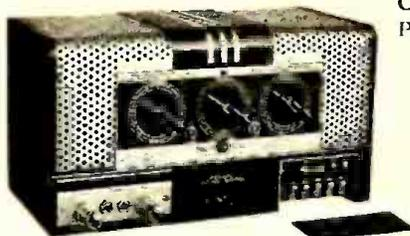
● (above) A de luxe, 24-watt amplifier with remote electric mixer. Splendidly shielded and cushioned input circuits insure quiet operation. Inverse feed back circuit... continuously variable tone control... automatic bass compensation for phonograph reproduction... two 250 ohm and two 0-5600 inputs... variable output impedance 4 to 250 ohms... finish, silver gray and aluminum. MI-4284, Price \$133.50 (Less Tubes and remote electric mixer unit).
