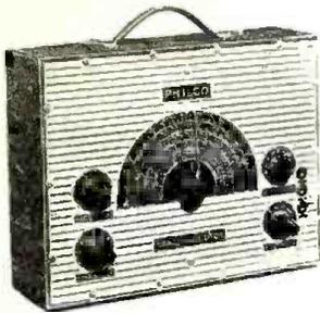
★ Precision type AC operated all-wave oscillator. Tunes 115 to 37,000 KC in 5 bands. Large direct reading scale with commonly used adjusting frequencies marked. 400-cycle audio modulation. Moisture-proofing insures permanency of calibration. Mirror-polished brass panel, unaffected by line voltage variations. Model 077—net \$27. Philco Radio & Television Corp., Tioga & C Sts., Philadelphia, Pa.—**RADIO TODAY**.
