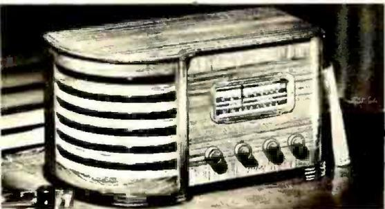
6 TUBE MODEL D-12. A two-band AC-DC Superhet of brilliant styling. Tunes 1720 to 535 K.C.; 2200 to 7000 K.C. Features: 2 Watts Output; Beam Power Tube; Tone Control; A.V.C.; 6" Slide Rule Dial; 6" Electro-dynamic Speaker. Size: 16" x 7 1/2" x 9 3/4". The new type table cabinet has the exclusive SONORA louvre grille.
