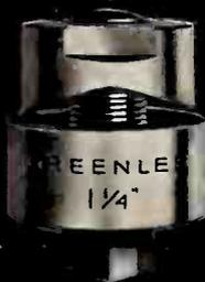
Here's a handy tool to help the radio worker save many hours of work when cutting holes for sockets, plugs, connectors, meters, and other receptacles in radio chassis. A cap screw is inserted in a small drilled hole, and the punch is easily forced into the die by a few turns of the cap screw with an ordinary wrench. Smooth holes, requiring no filing or reaming, can be cut in metal up to 1/8-inch thick in 1 1/2 minutes or less.
