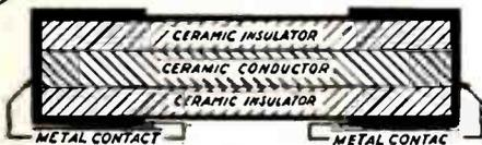
Magnified cross section shows center core of resistance material surrounded by a non conducting shock proof ceramic.
