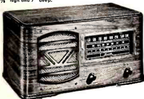
FARNSWORTH MODEL CT-42 . . . 4-tube Superheterodyne. 6" permanent magnet dynamic speaker. Automatic volume control. Cabinet takes any standard make battery pack. Standard and police broadcasts, high legibility slide rule dial with two-tone metal escutcheon. Beautiful walnut veneer cabinet size 18 1/2" long, 9 1/2" high and 10 3/4" deep.
