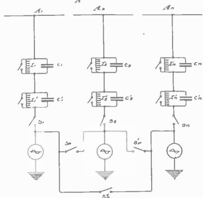
for limiting the currents caused by the electromagnetic or electrostatic induction between any two sections.
