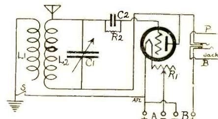
FIG. 36.—Wiring diagram of the Solodial, single-control circuit.
