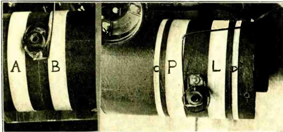
TWO VIEWS of the stator windings are shown in Fig. 7, above, at left. For Figs. 1 to 6, inclusive, see front cover. In Fig. 7 A has 20 turns of No. 26CCC wire, and so has B, but B is tapped at its tenth turn, or the thirtieth turn from the beginning, because A and B are a continuous winding. The tap is carried out to binding post No. 1. (See Fig. 2 on front cover).
