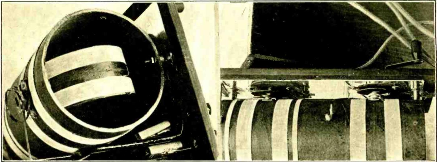
THE ROTORS (Fig. 9, at left) are wound on 2½" diameter tubing, 1¾" high, and have 17 turns each. Notice that pigtail connections are used, as these afford secure contact. The coiled pigtail may be plainly seen at left in Fig. 9. The objects at lower right in this photograph are fixed condensers. The photograph at right (Fig. 10) shows the aluminum shield, placed 1" in front of the tuner unit and connected to ground.
