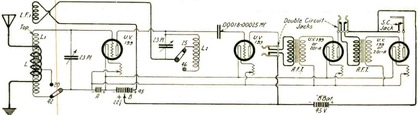
THE FAMOUS SUPERDYNE circuit which has held the interest of thousands of fans since its inception. Coils L, L1 and LF1 compose the variocoupler, and coil L2 is the plate coil. The use of the grid leak as shown is optional, as in many cases better results are had by placing from the grid post to the positive filament post on the socket. With low loss parts this circuit is said to be the equal of a 6-tube set, and is noted for its extreme clarity.
