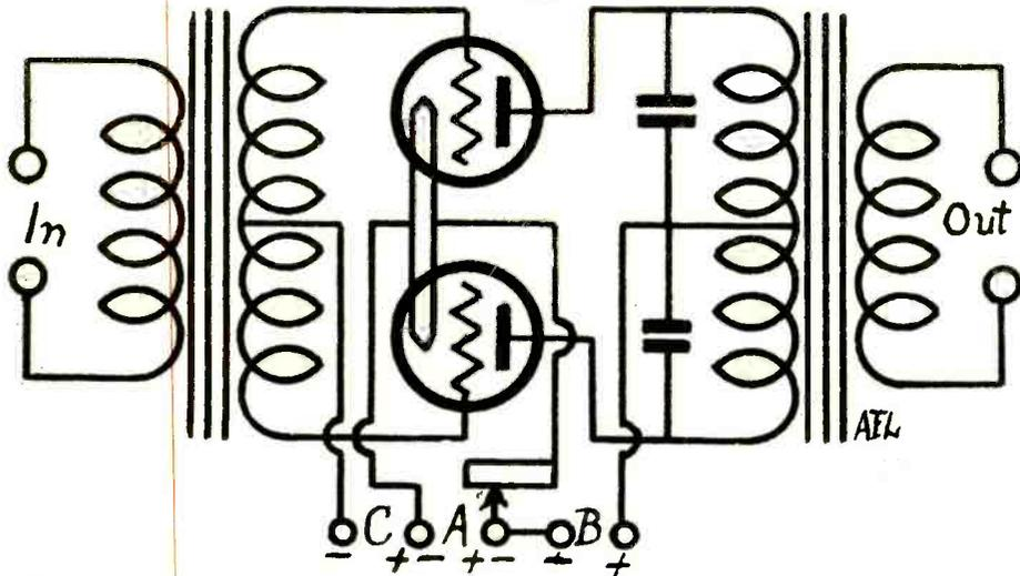
FIG. 38.—Push-pull power amplifier circuit asked for by Frank Baertich of Troy, Indiana. The transformers are purchased in pairs and are matched. Ninety volts are used on the plate and one rheostat controls both tube filaments.
