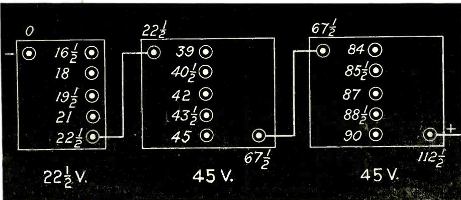
FIG. 39 shows how the connections come from the audio-frequency transformer.
