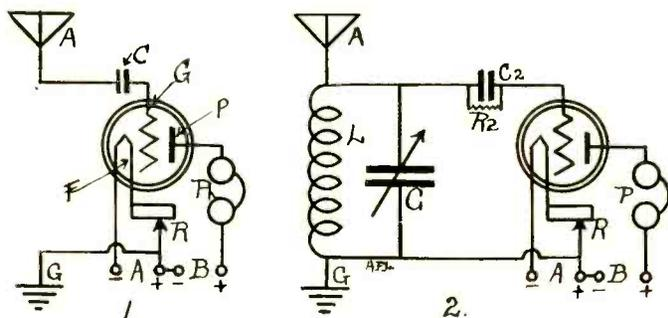
FIG. 1, A, antenna; G, grid; P, plate; F, filament; Ph, phones; R, rheostat; G, bottom, ground. In Fig. 2, L is a coil; C, a variable condenser; C2, grid condenser; R2, grid leak.
