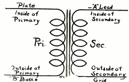
HOW the connections are made to an audio-frequency transformer. The plate lead, if this was the first AF, would be from the detector tube. FIG. 40
