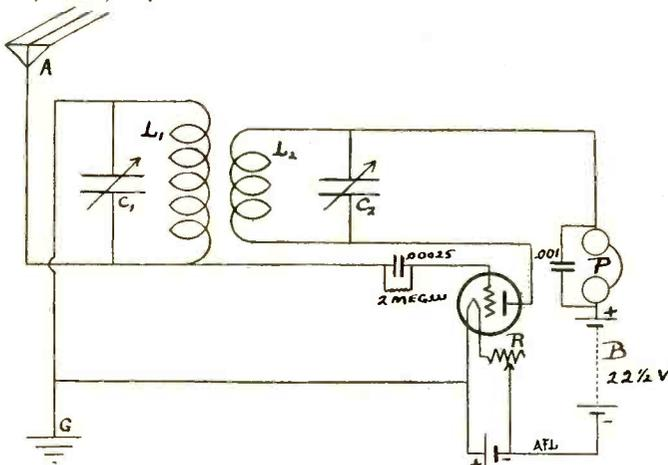
FIG. 37.—Circuit of a 1-tube set you can log.
