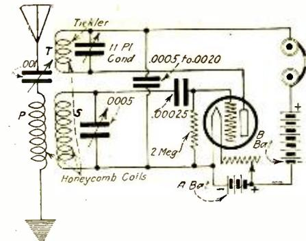
FIG. 35.—Diagram of a 3-circuit tuner using honeycomb coils.
