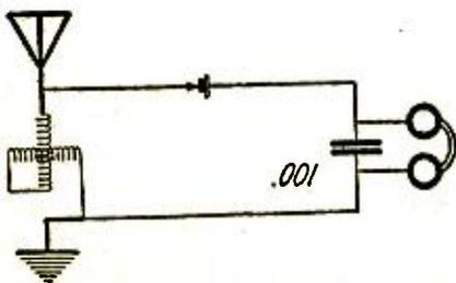
THE SIMPLEST crystal set, using a variometer. It is not selective enough.
