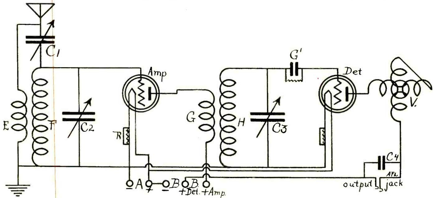
THE OSCILLATIONS in this circuit are kept under control by the condenser C1, which, when at a setting to be determined by experiment, will keep the tube at its most sensitive point. This setting may remain, hence there are three active controls in the circuit, not four. Both coils, E and G, are the same, E and G being 5 turns and F and H 50 turns, No. 22 DCC wire. All the variable condensers are 23-plate and must be low-loss for best results.
