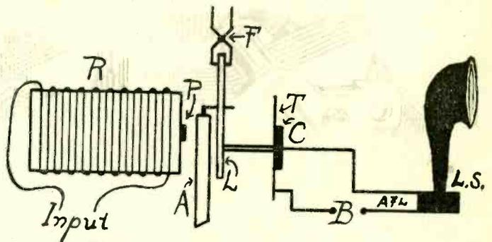
THE PARTS of the amplifier (Fig. 4). R is the receiver magnet; A, armature; L, lever; T, transmitter diaphragm; B, battery, 6 or 7 volts; LS, loud speaker; C, carbon button; F, fulcrum of lever; P, pole of the magnet, i. e., core.
