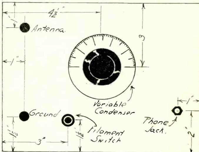
FIG. 3, panel layout. As no rheostat is used a filament switch is substituted to turn the tube on or off. The panel is 7 inches by 9 inches.
