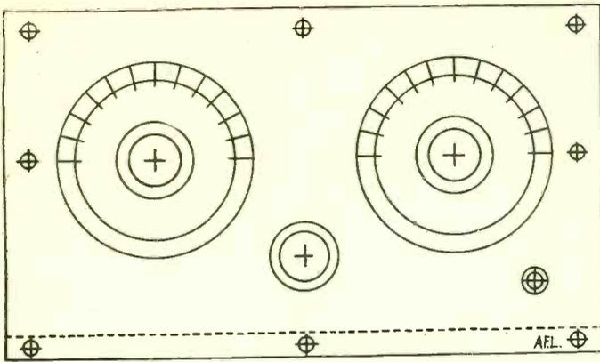
IF THE CONTROLS are to be kept down to two in a regenerative set, an aperiodic primary must be used for best results. Two controls will suffice for a reflex, if it consists either of crystal detector and a tuned RF stage or if a tube is used for detection. The Super-Heterodyne has only two controls.
