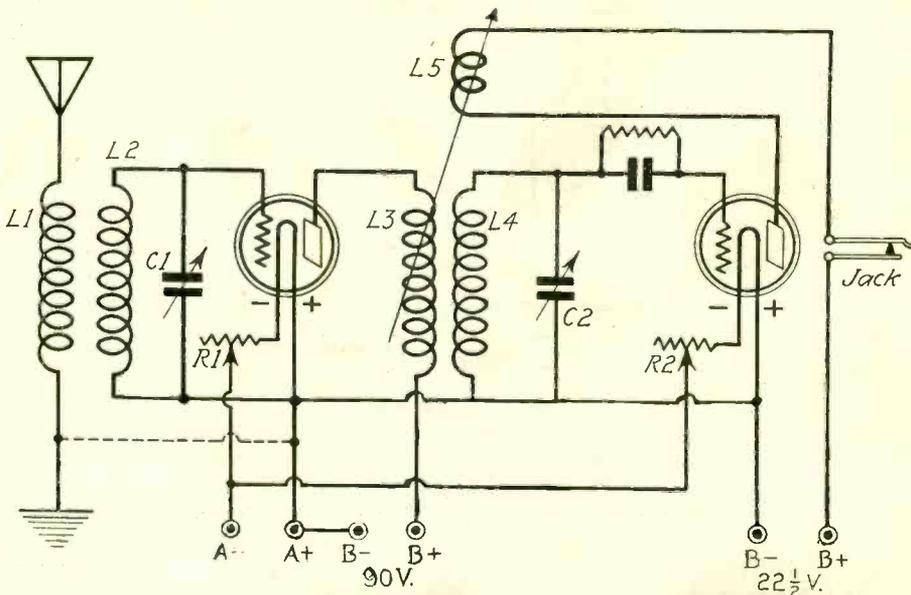
FIG. 1—Circuit network of the 3-circuit tuner, preceded by a stage of RF. The coil L1L2 is the RF transformer, home-made. L3L4L5 are the primary, secondary and tickler of the tuning coil, which preferably should be low-loss, though if you have a coil of another sort you may still get good results. Even a standard variocoupler may be used. In the July 5 issue of RADIO WORLD appeared an article describing how to convert a coil or variable condenser into the low-loss type.
