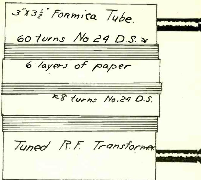
HOW to wind the timing coil (Fig. 2). A Formica or other tube, 3 inches in diameter by 3 1/2 inches high, is used. The secondary, 60 turns, is wound first. Six layers of wrapping paper go over this. Then the 8-turn primary is wound atop the paper, which, in the diagram, hides part of the secondary.
