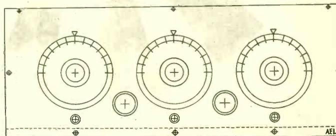
FIG. 3—Panel layout of a 3-circuit tuner preceded by an RF stage. At left, the RF condenser dial. Center, detector wavelength dial. Right, dial for rotor of variocoupler.
