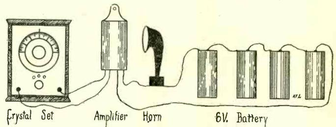
ARRANGEMENT of detector, amplifier, loud speaker and 6 or 7-volt batteries in circuit used by Father Judge.
