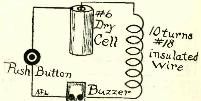
FIG. 4—A dry-cell, buzzer and small coil of wire, the coil placed a few inches away from the tuning coil of the receiving set, makes the correct adjustment of the crystal possible whether or not signals are being received. This is the well-known "buzzer test."
