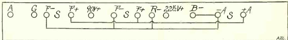
THE TERMINAL STRIP (Fig. 2), at right angles to baseboard, located at rear.
