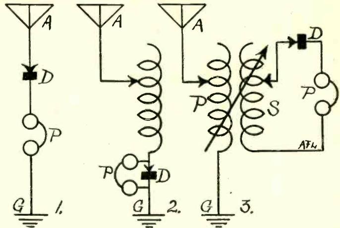
FIG. 1—The simplest receiving circuit, untuned. Fig. 2—The addition of a tuning coil enables the selection of different wavelengths. Fig. 3—Adding selectivity to the simple tuned circuit.
