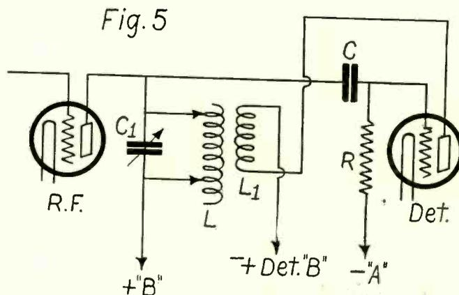
HOW THE SINGLE-CIRCUIT SET may be adapted to RF amplification. Note that regeneration is retained, the coil L1 feeding back the plate current to the grid of the detector, with a suggestion of RF and detector plates being in parallel. The plate of the RF tube and the B+ 90 volts (through L) replace the former aerial and ground connections, which are moved over to the RF circuit.
