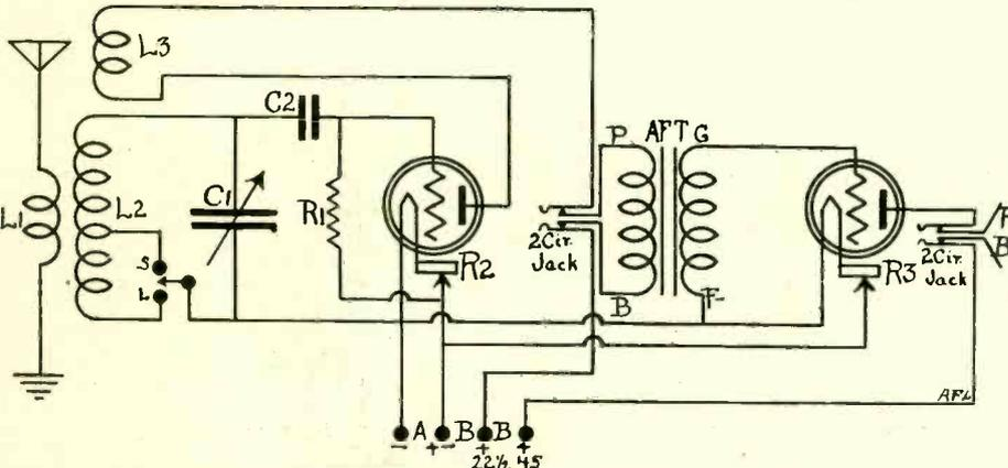
FIG. 36—One stage of audio-frequency transformer-coupled amplification connected to single-tube regenerative set. Locals may be heard with good volume on the loud speaker and DX stations on the head phones. An extra 22 1/2-volt B battery is necessary. Circuit requested by Paul Whalen, 5302 Buchanan St., Los Angeles, Cal.
