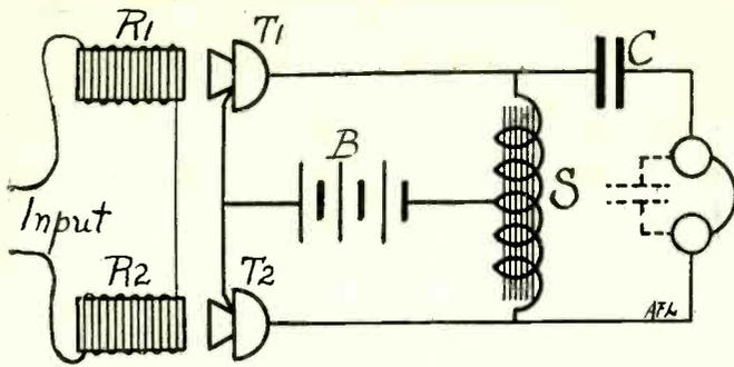
TWO RELAYS were used by Father Judge and better results obtained (Fig. 5). R1 and R2 are the receivers, i. e., the output of the crystal set and input of the amplifier; B, battery, 6 or 7 volts; S, split coil; C, 1 or 2 mfd. condenser; T1 and T2, amplifier transmitters.
