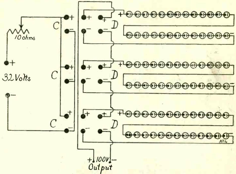
FIG. 35—How to charge a 110-volt storage B battery from a 32-volt farm lighting plant (direct current). The cells are arranged in three groups of 26 or 78 cells in all. These three groups are charged in series-parallel and discharged in series. Asked for by C. R. Lytle, Hitchcock, S. D.
