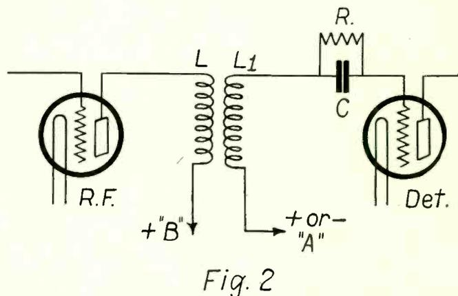
AN UNTUNED RF TRANSFORMER is shown here (LL1). Two honeycomb coils L, 25 turns, L1, 75 turns may be used, closely coupled. Remove twelve turns from L. A variocoupler may also be pressed into service, L being the primary. But the rotor, L1, must have more turns put on it or be shunted with a .0005 mfd. variable condenser. In either event the RF stage would be tuned, however. Note how the plate of the tube at left is connected by L to the B+ 90 volts, as referred to in the caption of Fig. 1.
