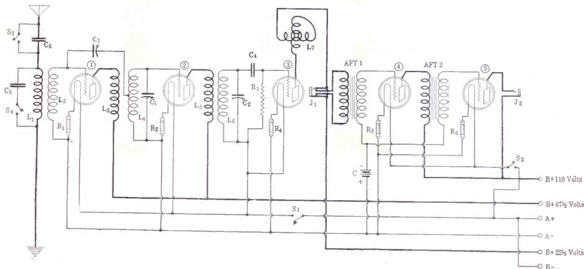
Fig. 1, showing the electrical diagram of the Improved Diamond. There are 5 tubes in this set instead of 4 tubes as in the original Diamond.
