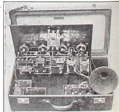
AN INTERIOR view of a 6-tube receiver, employing 3 steps of untuned radio-frequency amplification, a detector and 2 steps of transformer coupled audio-frequency amplification. A .0005 mfd. variable condenser tunes the antenna.
