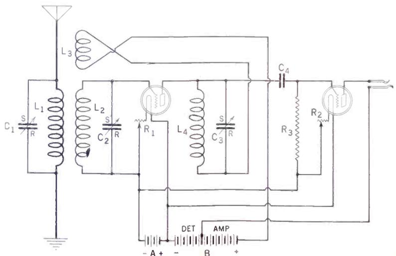
CIRCUIT diagram of 2-tube set with tuned aerial (Fig. 183).
