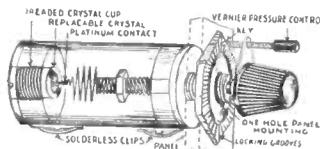
FIG. 8, detail of a semi-fixed crystal detector.
