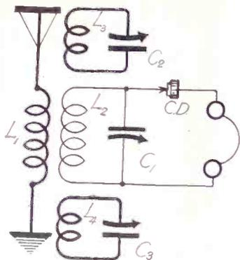
A SELECTIVE CRYSTAL SET for a point of reception that has a 3-station range. Any one of the three stations may be tuned in by C1, the two others tuned out by the wave traps, L3C2 and L4C3. As the primary L1 is not tuned there is no compensating effect and the set may be logged. (Fig. 1.)
