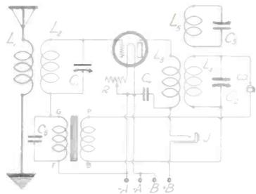
**THE WAVE TRAP** idea embodied in a 1-tube reflex. This circuit is good for earphone reception even in congested areas. (Fig. 4.)
