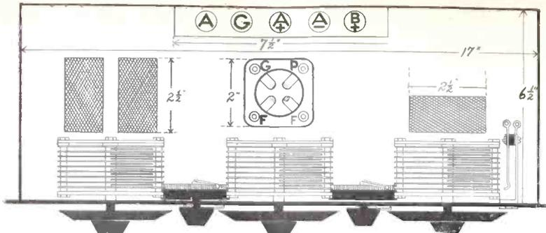
THE LAYOUT for The 3-Circuit Tuner You Can Log, using honeycomb coils. (Fig. 186).
