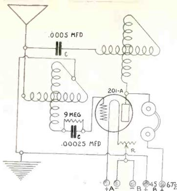
FIG. 189, showing a receiver employing 1-Tube, the grid and plate being tuned by variometers. The rheostat has a resistance of 10 ohms. When building this set, place the variometers no more than 2 3/4" away from each other. The mid-tap is taken where the rotor and the stator join.
