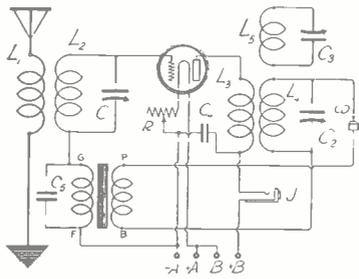
THE WAVE TRAP idea embodied in a 1-tube reflex. This circuit is good for earphone reception even in congested areas. (Fig. 4.)
