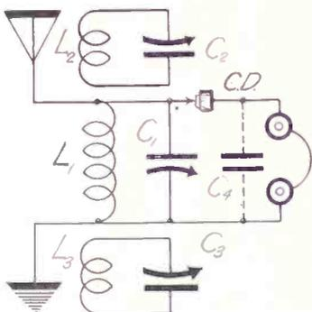
A TUNED IMPEDANCE primary gives more volume than the inductive coupling method shown in Fig. 1, but the set suffers in selectivity. Under certain conditions, explained in the text, this hook-up is very good. (Fig. 2.)
