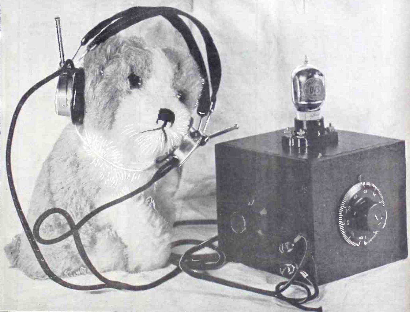
THE THOROUGHbred, shown above, at right, is a 1-tube DX set of extreme simplicity and economy. The home-made cabinet is only 5 1/2" square. Compare its size with that of the headphones the toy thoroughbred (at left) is wearing. See constructional article on page 3. (Hayden Photo.)
