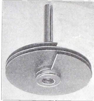
FIG. 5, closeup showing how the Spiral Condenser looks. The rotor plates enter the field of the stator one in spiral fashion. From maximum to minimum capacity is represented by 500 divisions of the dial. A counter tells the number of revolutions.
