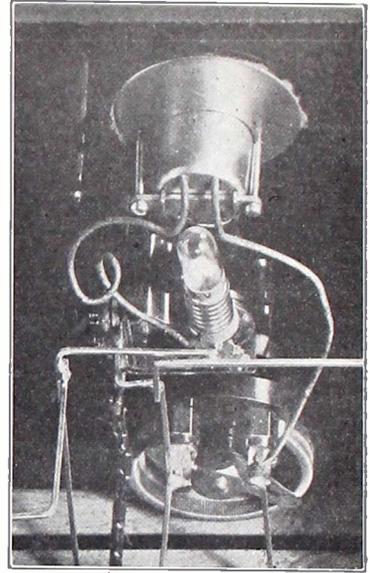
FIG. 5, a pilot light in use in a set. The top instrument is a voltmeter measuring the radio tube filament voltage.
