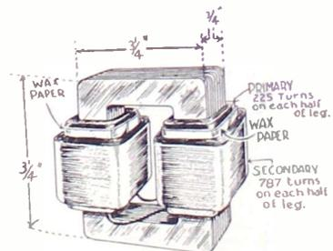
HOW an AC transformer with an output of 340 volts is wound is shown above. No. 22 SCE wire is used to wind the primary and No. 30 SCE is used to wind the secondary.
