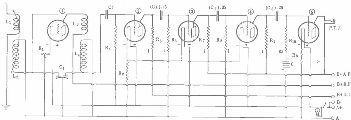
THE circuit diagram (Fig. 1) of the 1-dial receiver, with a separate B-plus lead for the RF amplifier tube, as this voltage must be just right. The primary is adjustable, as distinguished from a variable primary. A pilot lamp is used (lower right).
