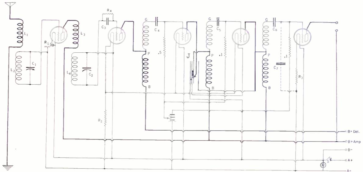
A DIAGRAM of a set similar to that above, except that a tube is used as detector, instead of a crystal. L1L2 and L3L4 are all standard radio-frequency transformers.
