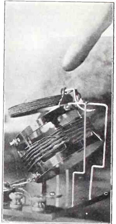
**FIG. 7, the adjustable primary.** This differs from a variable primary in that the adjustment, once made, is left that way.
