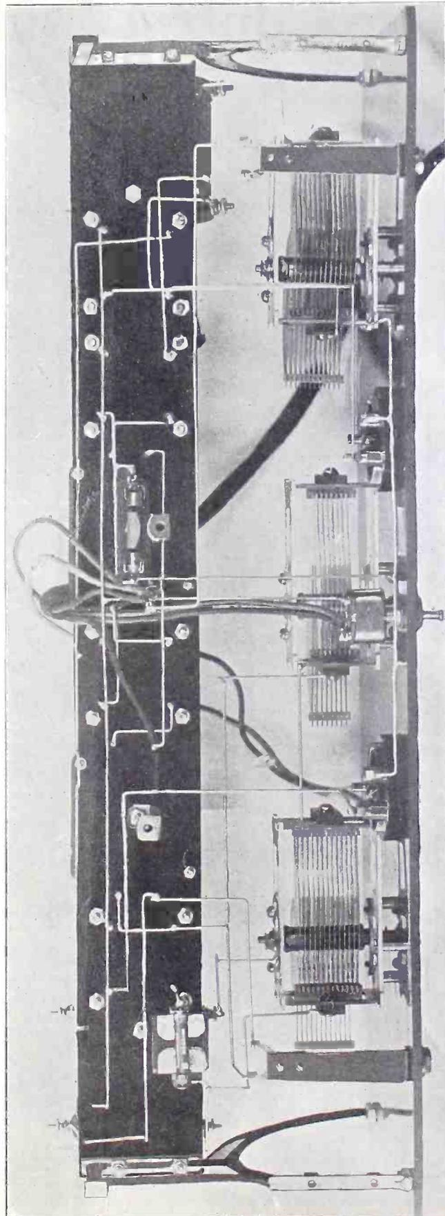
**FIG. 6, the bottom view of the receiver, clearly showing the wiring. Note that, to support the socket shelf, angle brass is used. The bottom view of these angles is shown 3¼" and 6", respectively, from the left bracket. The grid leak and grid condenser are behind the left-hand jack.**
