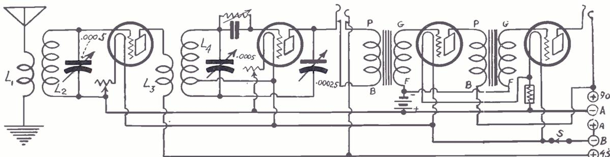
FIG. 1 shows the circuit diagram of the 4-tube DX Symphony. This set uses one stage of tuned radio-frequency amplification, a detector regenerated by the Hartley system, and two stages of audio-frequency amplification, employing transformers. As for the switching plan consult text.
