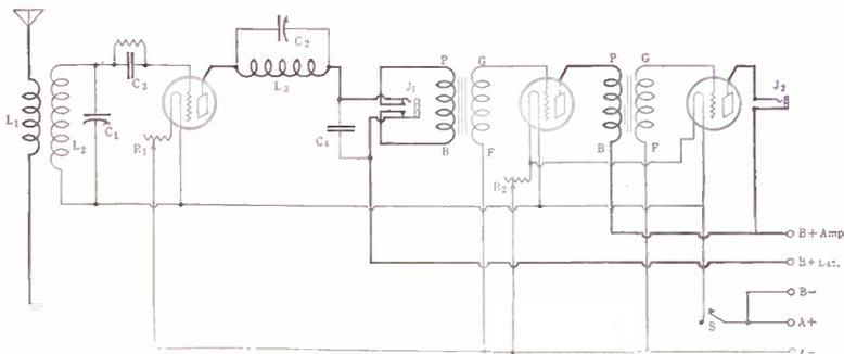
A 3-TUBE regenerative receiver with a variable condenser, C2, having a capacity of .0005 mfd. tuning the plate. R1 is a 10-ohm rheostat, while R2 is a 6-ohm rheostat.
