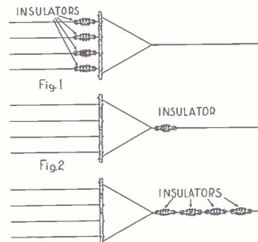
placed at the extreme end of the antenna, as in Fig. 2, for then the total resistance would be 40 ohms. If the four insulators were connected in tandem as in Fig. 3, the total resistance would be 160 ohms or sixteen times as much insulation as with the arrangement in Fig. 1.
