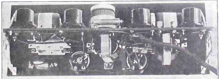
REAR VIEW showing the manner of mounting the Radio Foundation toroids, the Carborundum fixed crystal detector, the sockets, AF transformers and other parts.
