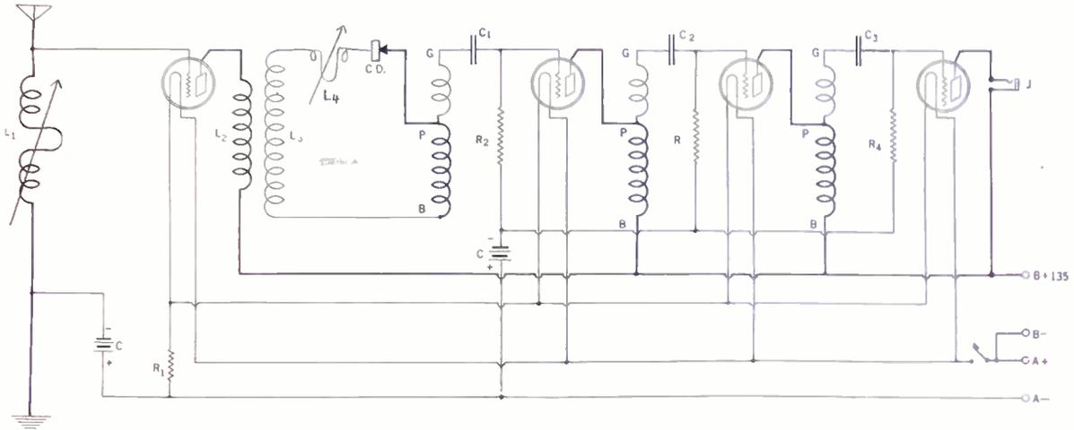
THE electrical diagram of a quality 4-tube receiver. L1 is a variometer. L2L3 is a radio-frequency transformer, 10 turns for L1 and 45 for L2 on 3½" diameter. L4 is a variometer. Three autoformers are employed. R2, R and R4 are all 500,000 ohm resistors. C1, C2 and C3 are 1 mfd. fixed condensers. R1 is a 1 ampere resistor. All the tubes are of the 201A type. The first C battery in the RF stage has a voltage of 4½. The second C battery, in the audio circuit, has a voltage of 6.
