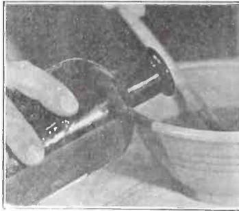
IN making a storage battery solution, always add the acid (sulphuric, H<sub>2</sub>SO<sub>4</sub>), slowly to the water, and not the water to the acid. If the opposite method is employed, a boiling and sputtering of the solution will take place. After each few drops of the acid are added in the correct fashion, stir carefully.
