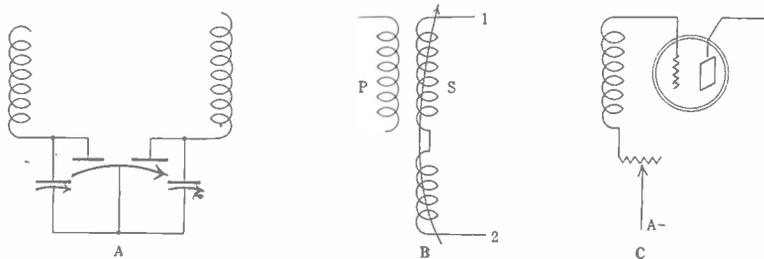
FIG. 2—A variable primary may be used as a balancer (Fig. 1) or small extra condensers may be used ("A"), or inductive variation in a conductively coupled secondary may be employed ("B") or the inductance of a rheostat may be utilized (a bad method).
