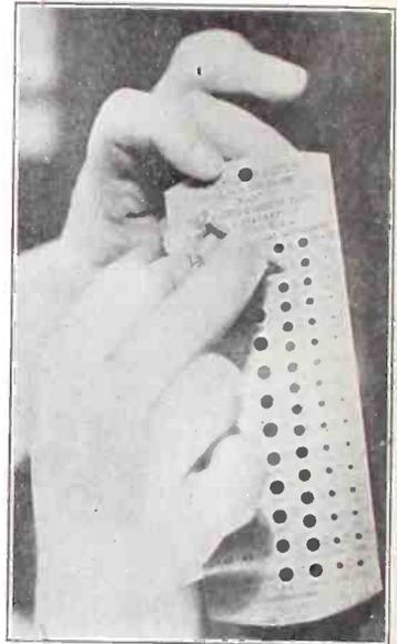
With the above chart, which is called a drill and Wire Gauge Chart for Machine Screw Taps, you can learn the standard number and size in decimals of an inch, of all types of machine screws. This enables you to know what size hole to drill in the panel. Besides finding out the size of screws, the diameters of shafts, of condensers, couplers, etc., may also be ascertained by inserting the shaft into the holes.
