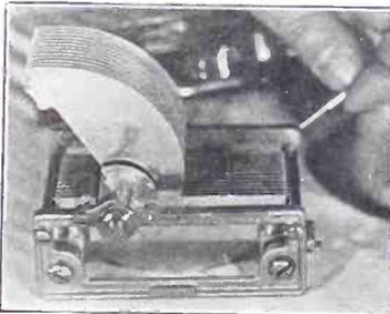
WHEN you test a variable condenser for a complete circuit a faint click may be heard, due to the charge and discharge of the condenser. Should you hear a loud click there is a short circuit in the condenser, that is, plates are touching each other.
