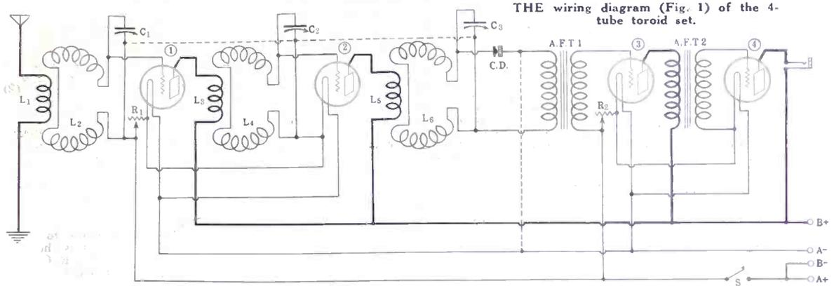
THE wiring diagram (Fig. 1) of the 4-tube toroid set.
