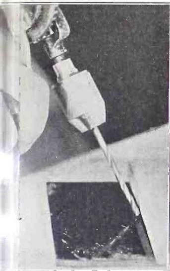
PHOTOGRAPH shows how to drill a hole in a panel, without having the drill slip off over the panel, thereby scratching it and delaying the work. Place a piece of wood snug up against the panel where the hole is to be drilled. Tighten down with a vice. Then you can drill the hole without any fear of the drill slipping, as it will rest up against the board.
