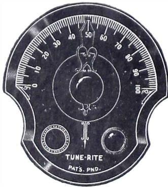
THE Tune-rite dial which, when used on a SLC condenser makes it tune on the SLF basis.
