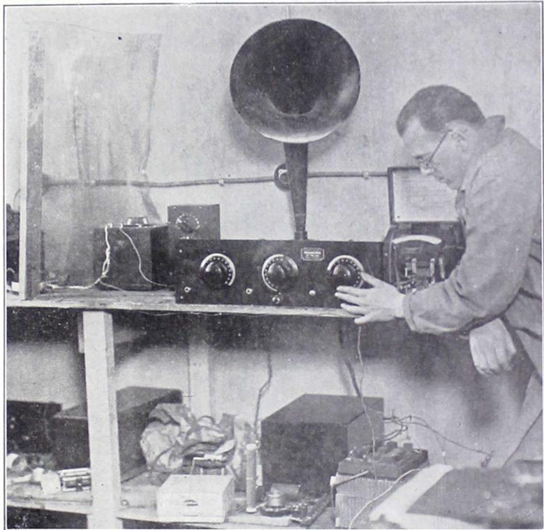
"EXTENSIVE TESTS have proved that a variable grid leak is necessary in every set that-uses a tube as detector," says John F. Rider, noted radio engineer, shown above, testing the Bretwood Variable Grid Leak in the 1926 Model Diamond of the Air. "The output voltage," he adds, "may be increased as much as 25 per cent. by correct leak setting." (Foto Topics)
