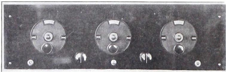
FIG. 3, the panel view. Three vernier dials are used. The two rheostats show up plainly. The jack and switching arrangement may be selected to suit the constructor's taste. See text.
