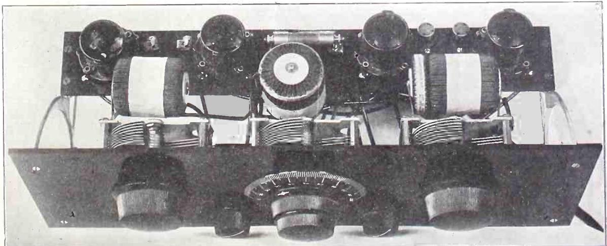
TOP VIEW. The tuning dial is vernier, while the compensating knobs adjust the first RF and detector input condensers for synchronized tuning. The toroids are mounted on the socket shelf behind the U. S. L. condensers.
