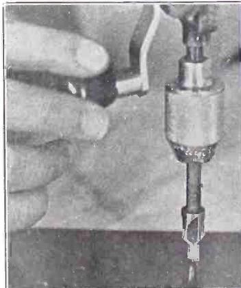
INSTEAD of taking the drill out of the bit to insert a countersink you may use a combination drill and countersink. After the drill has pierced the panel the countersink functions.
