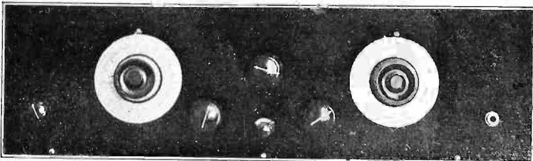
ON the front panel are the two 360-degree Remler dials for tuning. At left is the antenna series condenser knob. The rheostat for the three intermediate amplifying tubes is at right of the first dial. Next come the switch and the potentiometer. The oscillator rheostat and detector jack complete the list.
