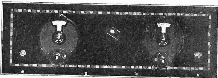
THIS SET has only two tuning controls. Jack, switch and rheostat complete the panel parts.
