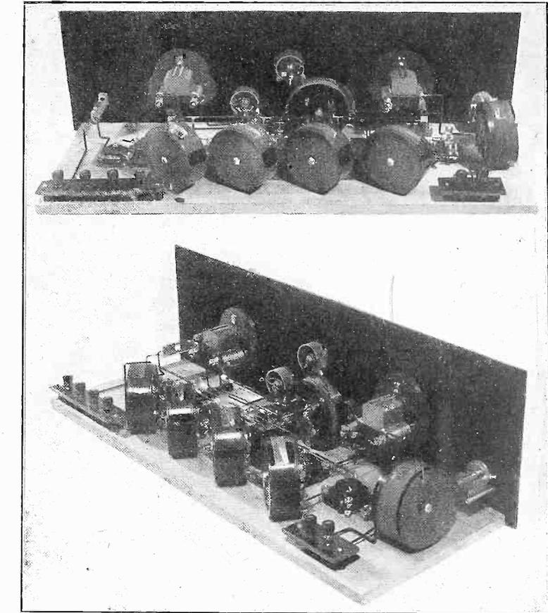
THE baseboard and panel layout of parts is shown in these two photographs. The angular position of the antenna coupler, extreme right, is to be determined experimentally. The conventional position is shown, but it is not always the best, as self-oscillation may be strong.
