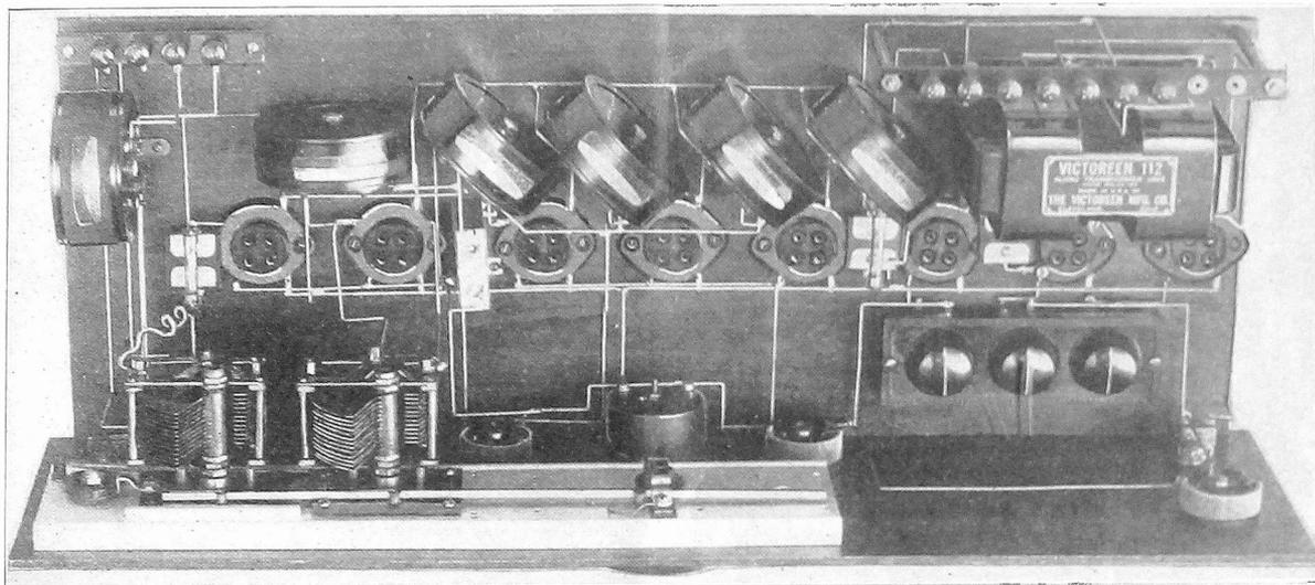
THE ATTRACTIVE LAYOUT of the 1928 Victoreen Universal, showing placement of coils and the 112 Victoreen audio unit, as well as Eby sockets, condenser and all other parts.
