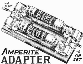
By means of a new device just introduced, it becomes possible to modernize the old set without the use of tools or the performance of a major operation. In fact, not a single wire within the set is altered; not a thing is changed; not a single practical fact need be known about radio; yet the old set is instantly transformed into a modern set so far as efficient and simplified operation is concerned.
