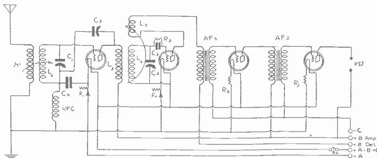
THE RHEOSTATS in the Knickerbocker Four are used for volume control and for sensitivity adjustment.
