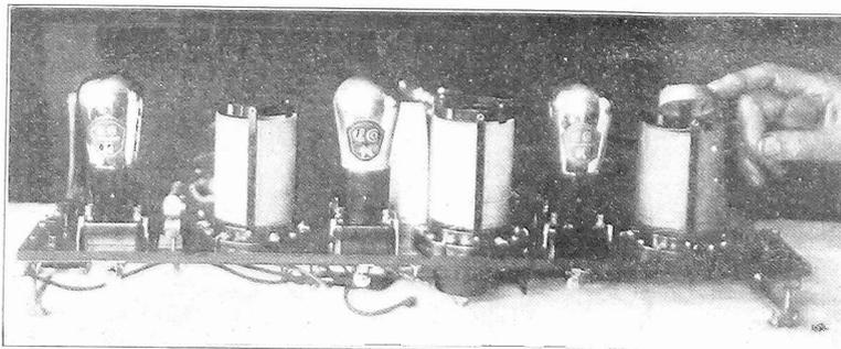
THE TUBES AND COILS are evenly distributed along the socket shelf. The antenna-ground posts are at right.
